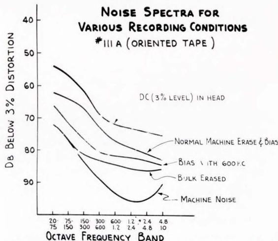
Figure 4. Noise spectra showing the effect of various imperfect erasing conditions.
