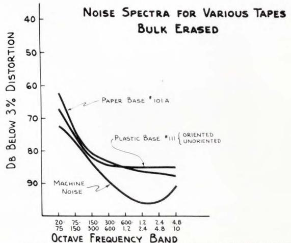
Figure 3. Bulk erased noise spectra for the same tapes as in Figure 2. The machine noise (tape motion stopped) is also shown.
