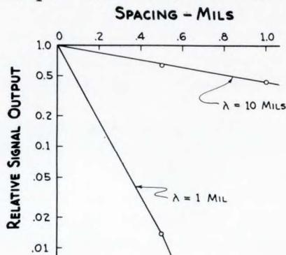
CURVES SHOWING FALL OFF OF REPRODUCED SIGNALS VS SPACING FROM REPRODUCE HEAD
