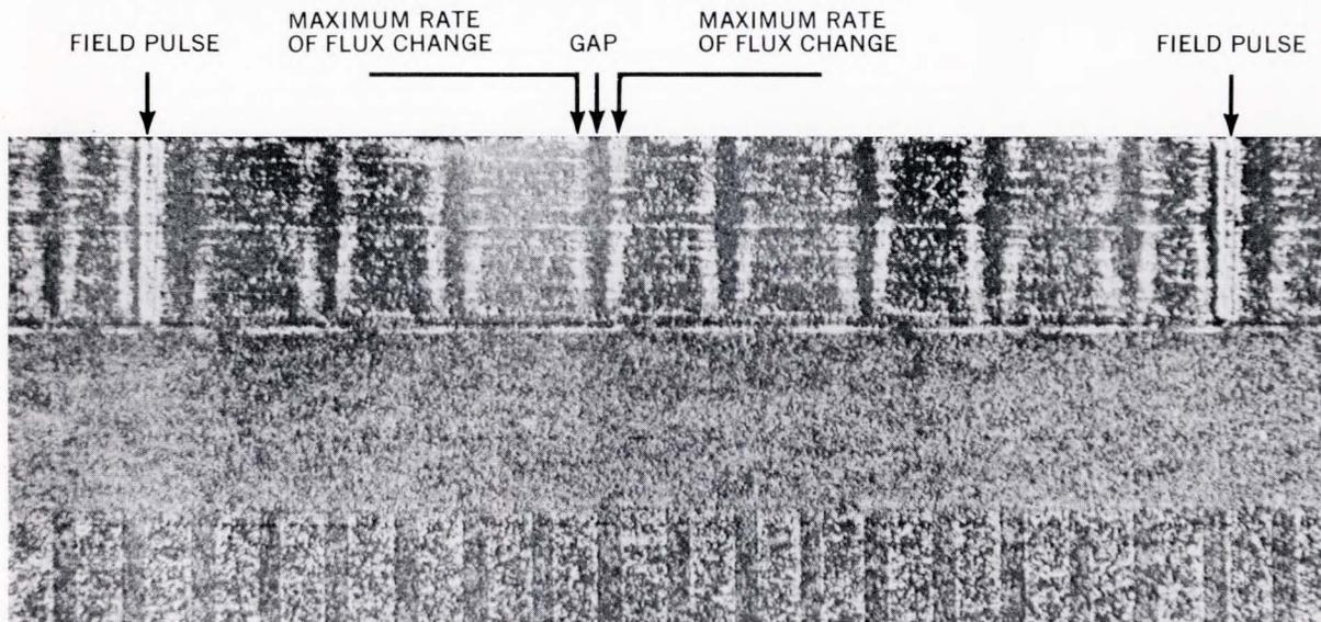
FIG. 2 PHOTOGRAPH SHOWING DEVELOPED CONTROL TRACK PATTERN.
