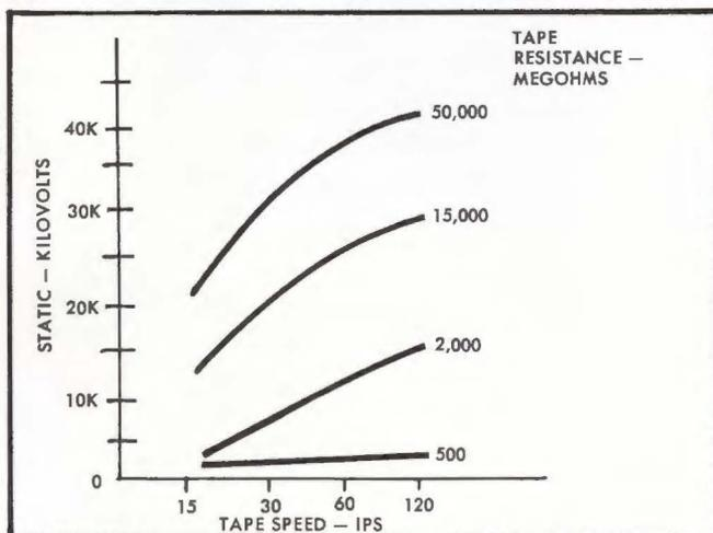
FIGURE 1. STATIC BUILDUP VS TAPE SPEED AND TAPE RESISTANCE
