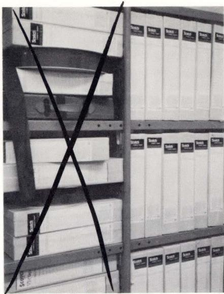
Tape should be stored "on edge" rather than horizontally in a stack. Basically, the reasons for this evolve around two considerations: Convenience and protection against damage to tape.
