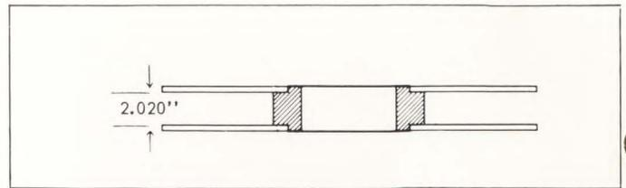
Under excessive pressure anything less than a perfect wind can result in edge damage to the tape with permanent audio and control track dropout.
