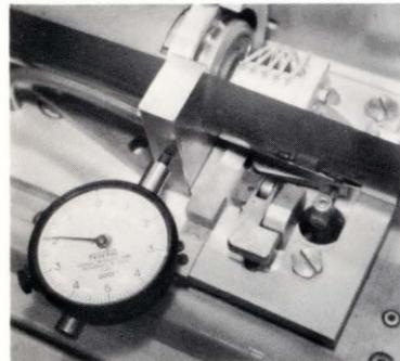
Measurement of Tip PENETRATION
