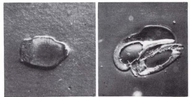
Photo-micrographs of two common types of coated-in tape flaws which have been largely eliminated by modern coating methods.
