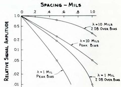
Curves Showing Fall Off of Recording Signals vs Spacing from Recording Head
