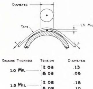
Optically Measured Size of Dropout Area Caused by 1.5 Mil Protuberance on 1/2" Tape Wrapped on a 1" Dia. Rod.
