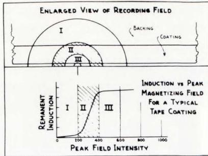
Diagram showing magnetic field pattern near the recording head (above). Below is a graph showing the relation of the recording field intensities to the magnetization curve of the tape coating.
