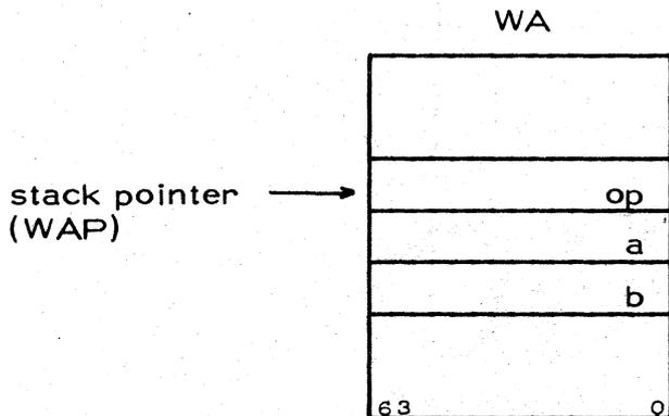
We wish to take two operands, a and b, and an arithmetical or logical operator, op, from the stack and place a op b on the new top of stack. The following microinstruction sequence does this.
