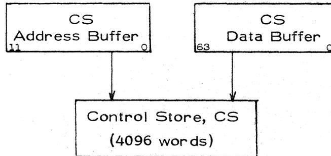
The CS Address Buffer is loaded from the Microinstruction Address Selector as shown in Figure 2.30. The CS Data Buffer is actually Device number 15 associated with Output Port A, OA. Let A be the address of the current microinstruction. The microoperation CS Load, if executed in the current microinstruction, can be interpreted as follows:
