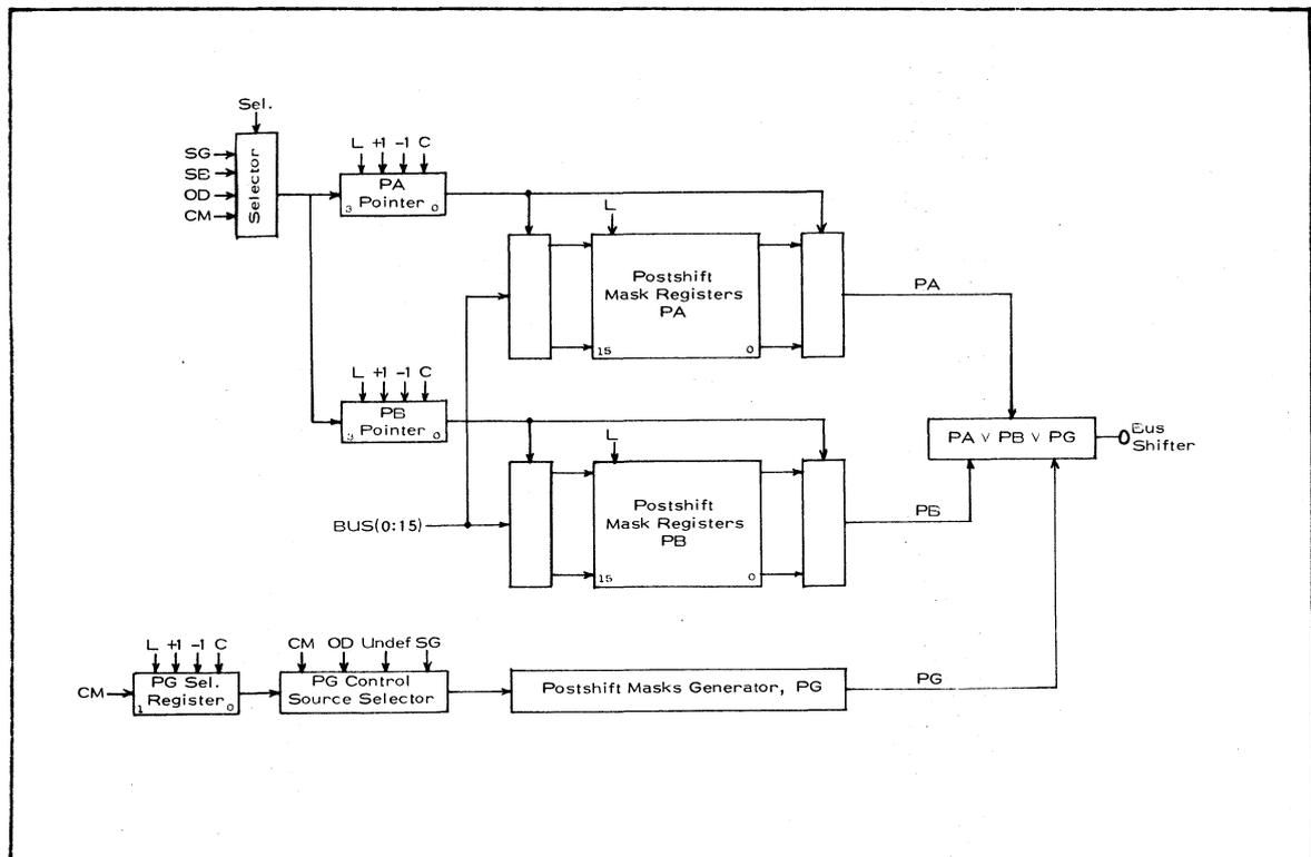
The most important thing to note from this diagram is that the PA/PB structure is indeed the same as the MA/MB structure (see Figure 2.9.).
