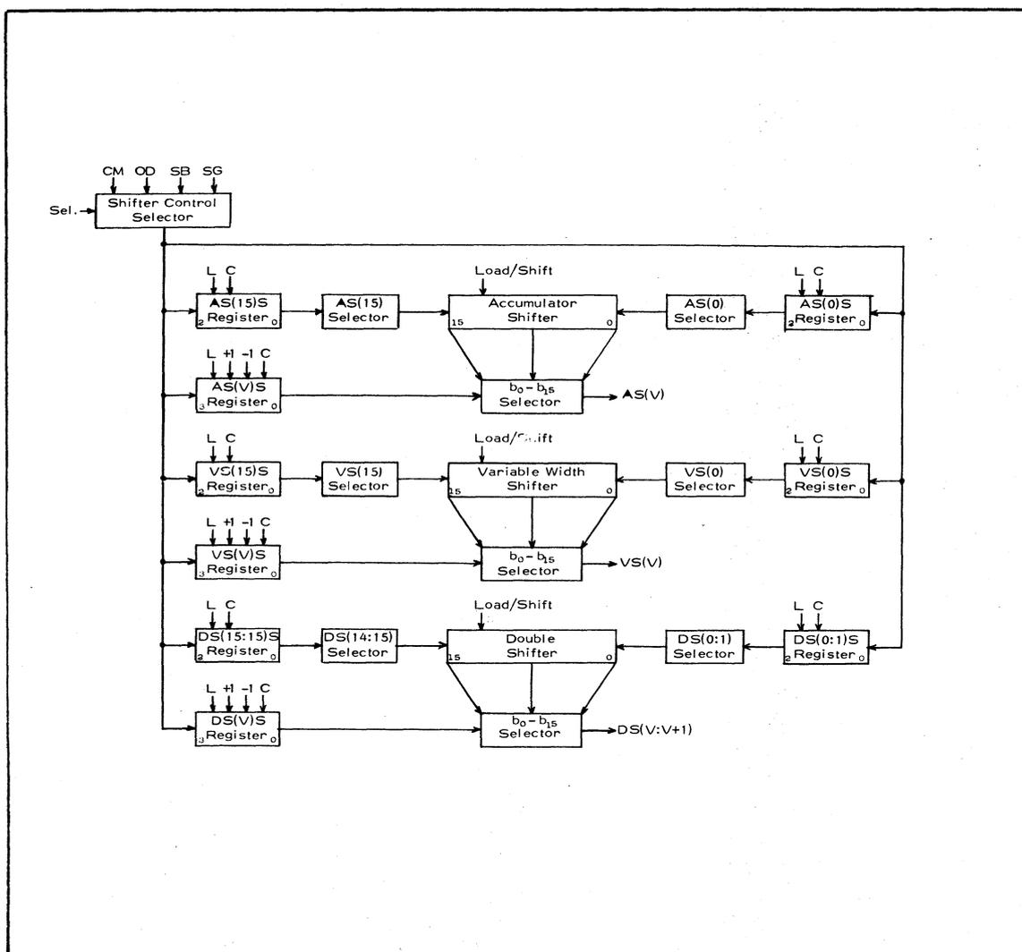
The SG which is associated with this selector is called the Common Shifter SG. Various shifter control data can be stored in this SG for various shifter interconnections and then used in environment prologues. The microoperations associated with the CS SG are shown in Table 2.16.
