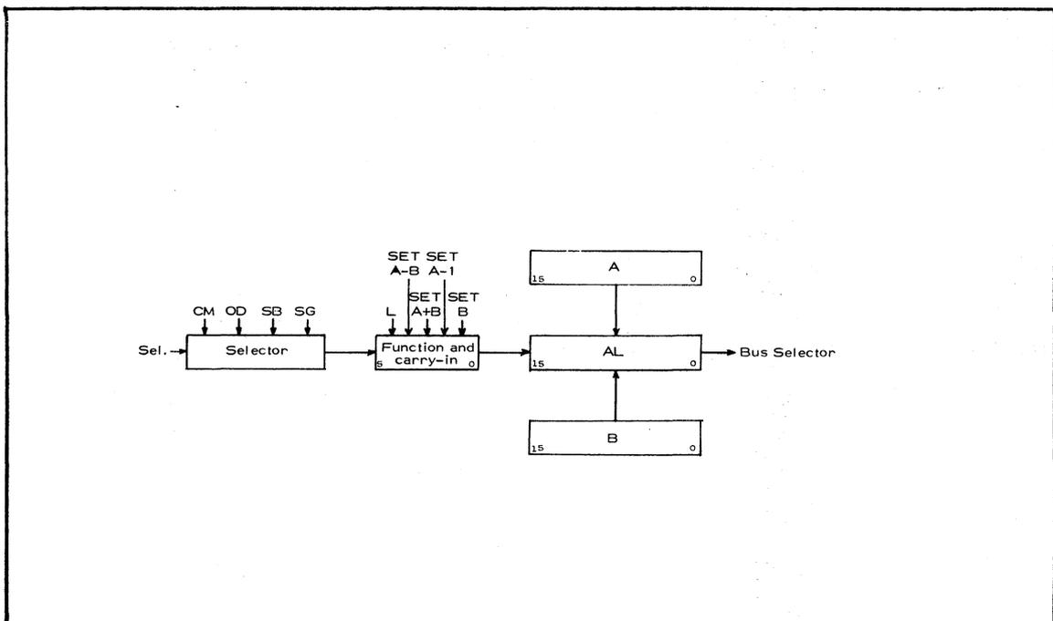
6 bits are required to control the AL: 5 bits to select one of the 32 operations listed in Table 2.10. which this unit can execute on A and B and 1 bit which specifies the carry-in bit into the AL for any arithmetic operations.
