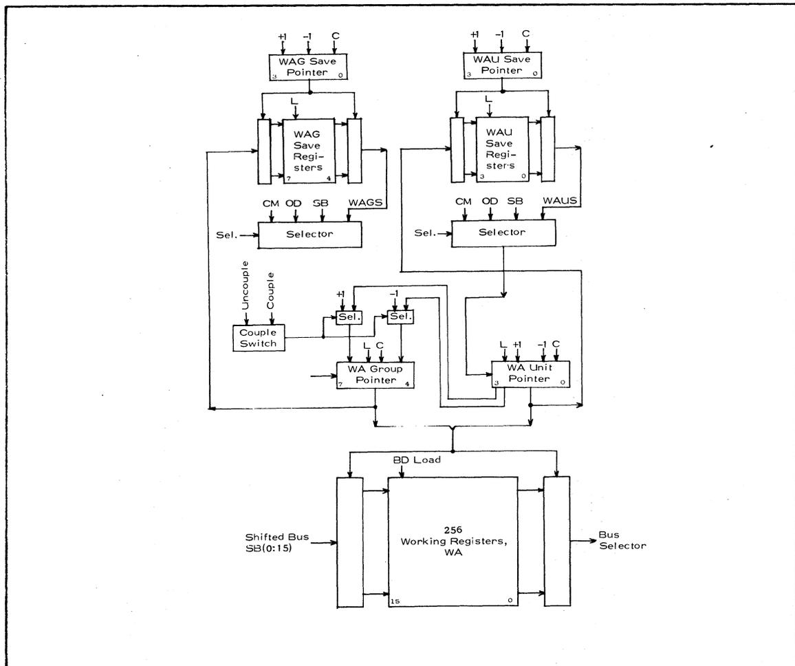
When the microoperation CPL A is executed, the Group and Unit pointers are connected together to give the 8-bit wide pointer, WAP. After the microoperation UNCPL A is executed, the Group and Unit pointers function as independent pointers. The low order 4-bits of the 8-bit address required to specify a particular register are given by the WA Unit pointer, WAU; high order 4-bits of the address are
