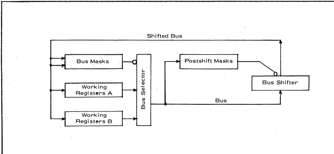
One of the purposes of the PM is to apply a mask to the output of the BS which will mask off the unwanted "cyclic" bits and replace them with 0's thereby simulating a logical shift. As an example, if the bus transport
