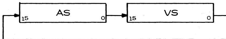
Just as with the AS, there are 2 bits in each microinstruction which control the operation of the VS: shift left,  $VS \leftarrow$ , shift right,  $VS \rightarrow$ , load, i. e.,  $VS := SB(0:15)$ , or remain idle.
