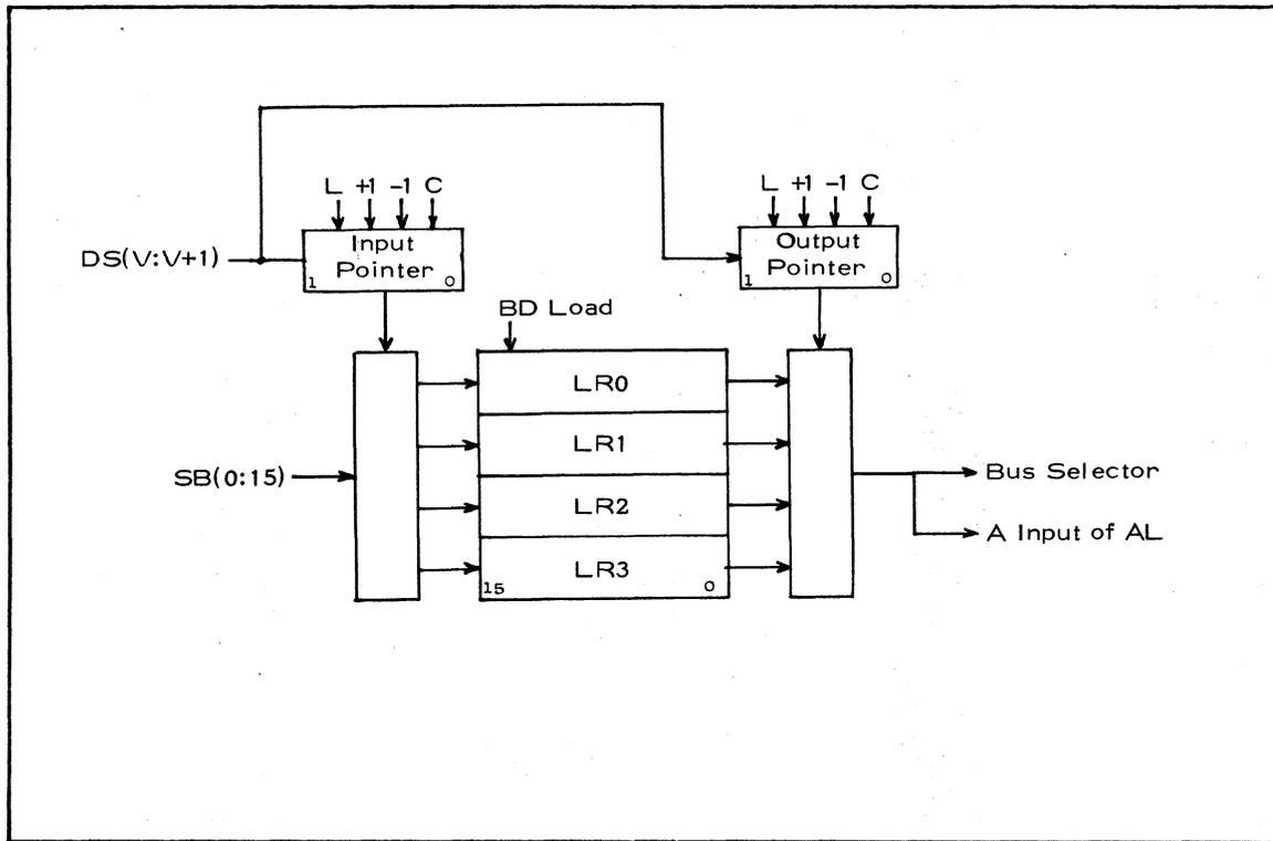
Both the LR input pointer, LRIP, and the LR output pointer, LROP, are incrementable, decrementable, clearable, and loadable with two bits from the Double Shifter,  $DS(V:V+1)$ , see Section 2.12. The utility of this last feature will be demonstrated with examples when the Double Shifter is introduced. Table 2.12. gives the microoperations associated with the control of the LR.
