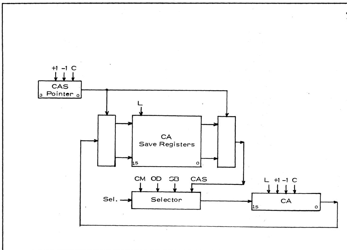
CA has four microoperations associated with it as shown in the box labelled 'CA' in this Figure. These microoperations are given in Table 2.2.
