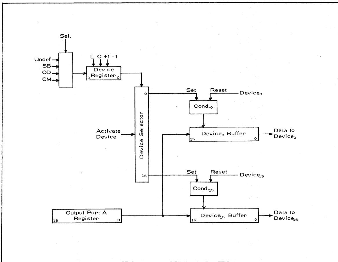
The particular device which is selected for output is pointed to by a device register. There is a condition associated with a selected device: space available, OASA. The microoperations associated with the control of OA and OC are shown in Table 2.20. The microoperations for OB are identical to those for OA and the microoperations for OD are identical to those for OC.
