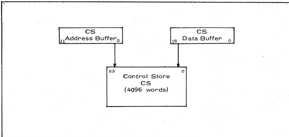
The CS Address Buffer is loaded from the Microinstruction Address Selector as shown in Fig. 2.32. The CS Data Buffer is actually Device no. 0 associated with Output Port B.
