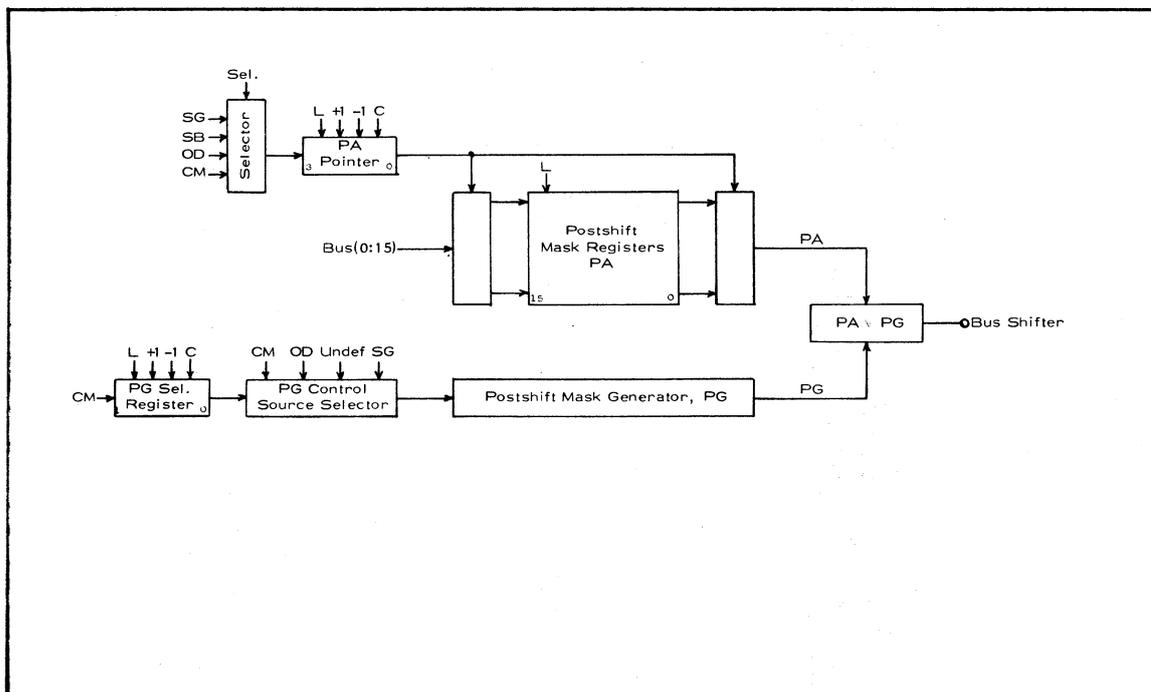
Which particular source is to be used as data for the mask generation is determined by the contents of a 2-bit Postshift mask Generator Selection register (PGS) as shown in this figure and in Table 2.8. below.
