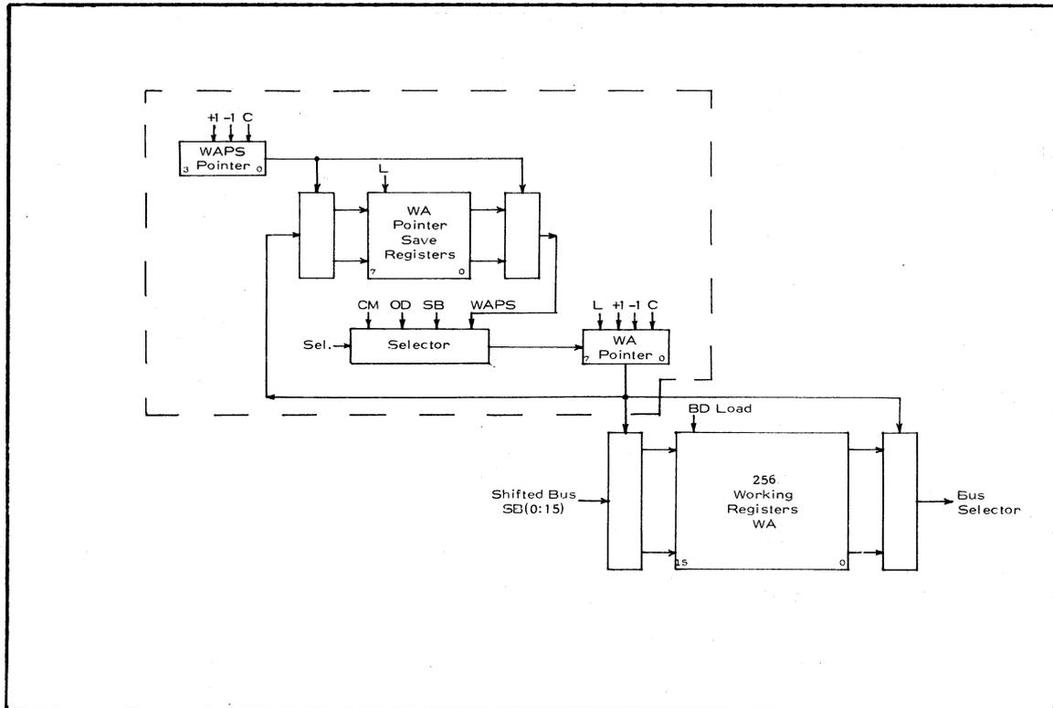
called the WAP Save registers, WAPS. This is identical to CA being saved. Also, as indicated in the box labelled "Selector" in Figure 2.5. the WAP can be loaded from any of four sources:
