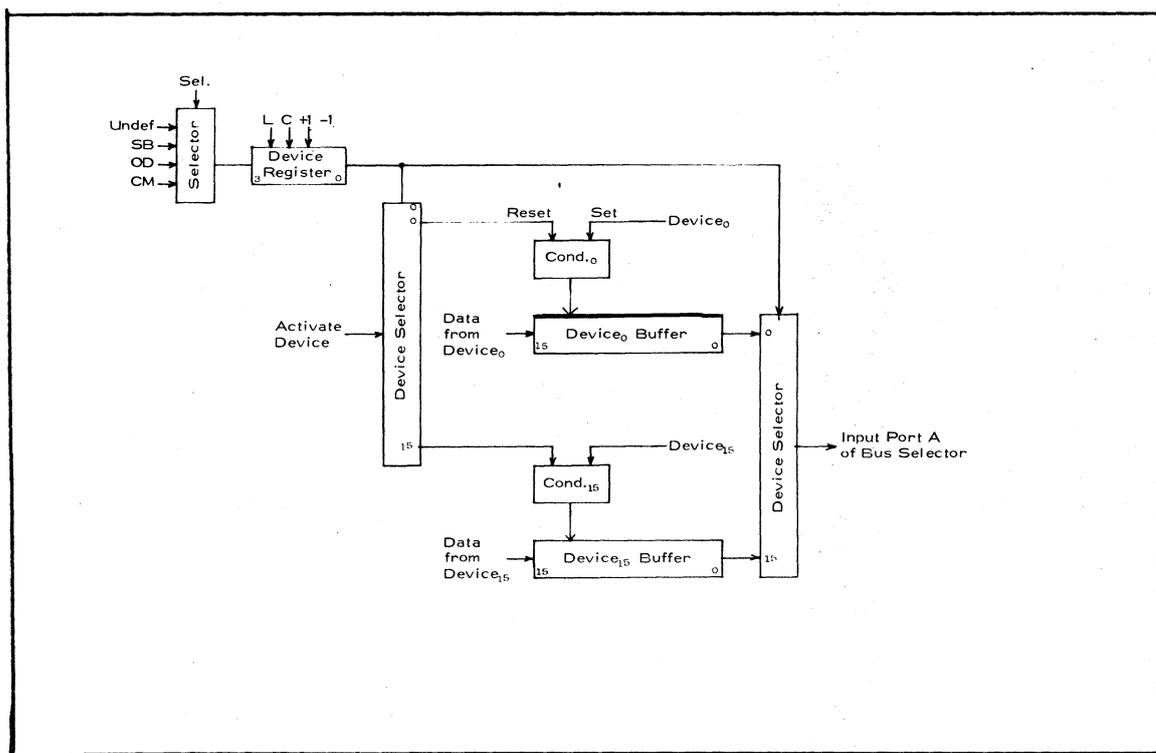
The particular device which is selected by the IAD register to be read is pointed to by a Device Register. There are two conditions associated with a selected device:
