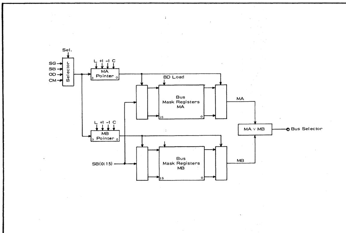
such that the "no mask", i. e., 15 1's, is in register 0 of MA and the "bus clear mask", i. e., 16 0's, is in register 1 of MA. We will assume this to be the case throughout normal operation of the system. One can
