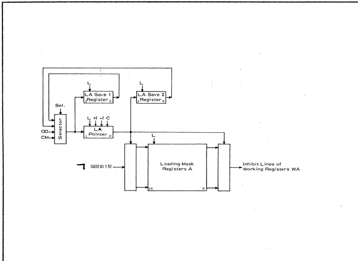
There are 7 microoperations shown in Figure 2. 22. associated with the use of LA. These are listed along with the corresponding microoperations for LB in symbolic form in Table 2. 18.
