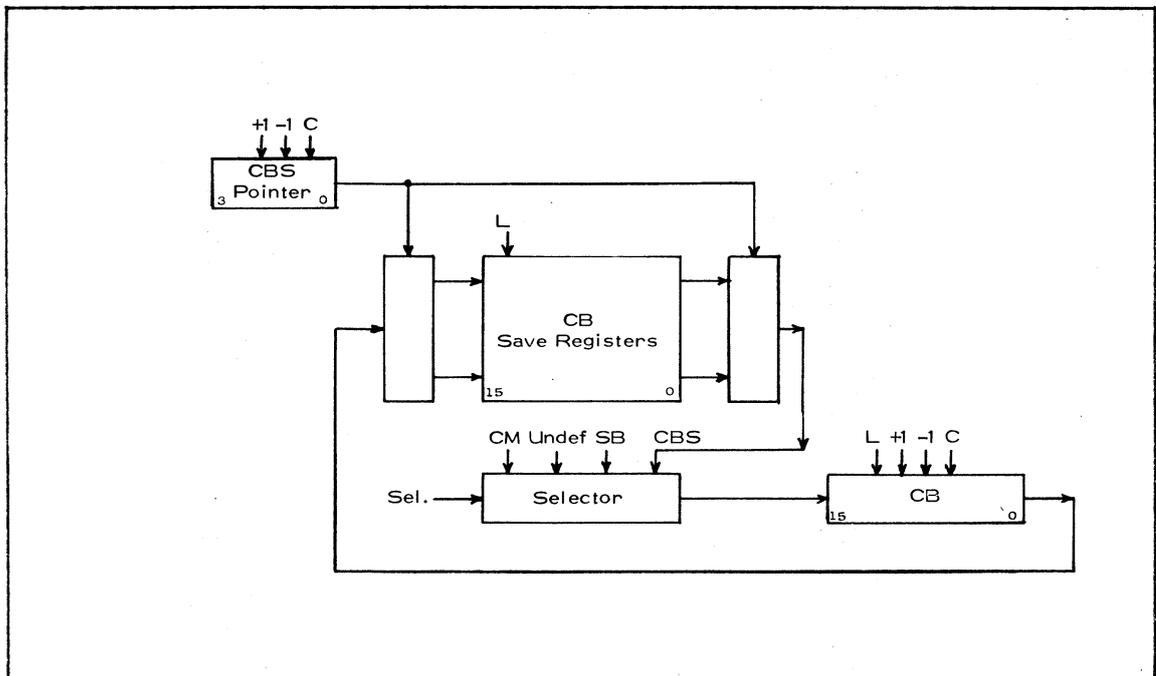
A comparison of this figure with Figure 2.3. which shows CA reveals that CB is identical with CA except that CA can be loaded from the OD register which is not the case with CB, i. e., we have
