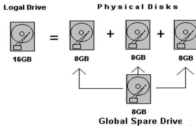
Global Spare Drive does not serve any particular logical drive. When a single drive fails from any of the logical drives, the Global Spare Drive will rebuild this particular logical drive automatically.
