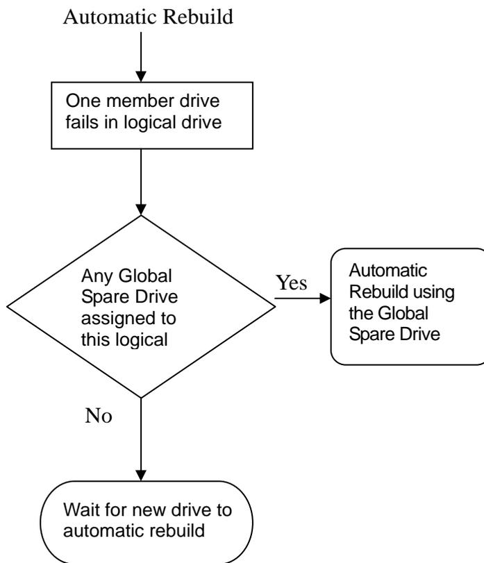
When one of the drive fails, the controller will check if there is any local spare drive assigned to this logical drive first; If yes, the controller will start to rebuild lost data automatically.
