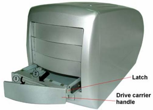
3. Place the disk drive at an angle in the drive carrier and connect the power connector to the disk drive
