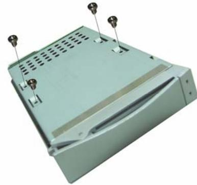
4. Lift the disk drive slightly out of the carrier and detach the power and IDE or SATA connectors.
