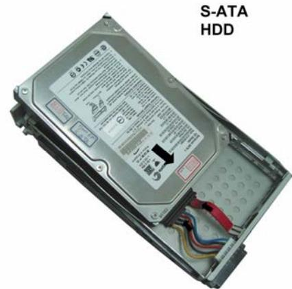
6. Turn the disk carrier upside down and secure the disk in the carrier with four screws.
