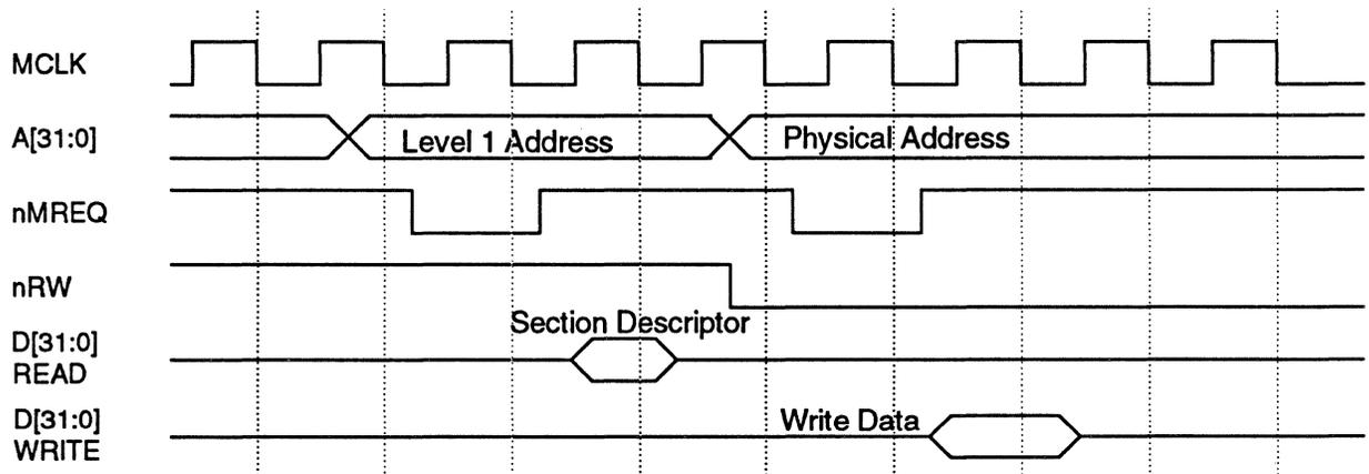
Figure 46: Translation Table-walking Sequence (write) For Section
