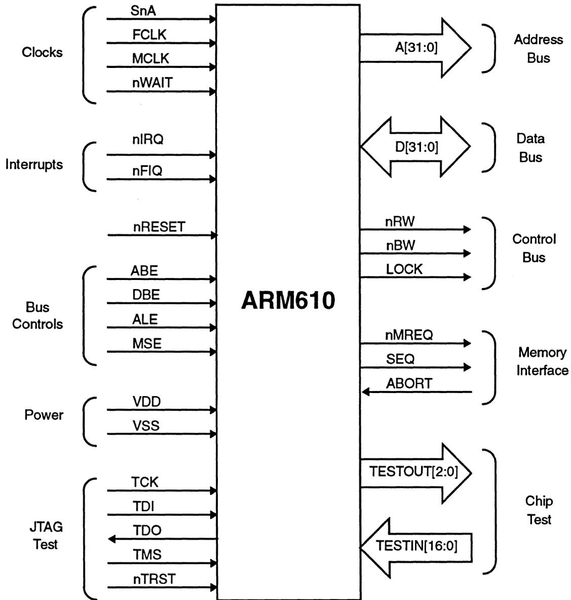
Figure 2: Functional Diagram
