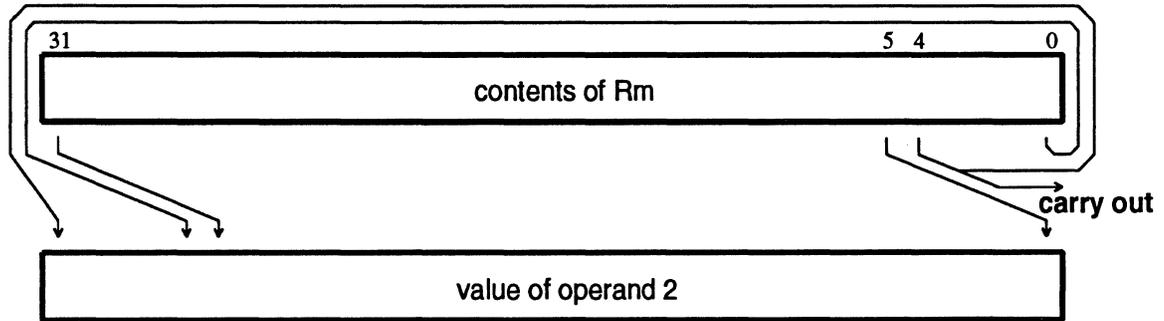
Figure 13: Rotate Right
