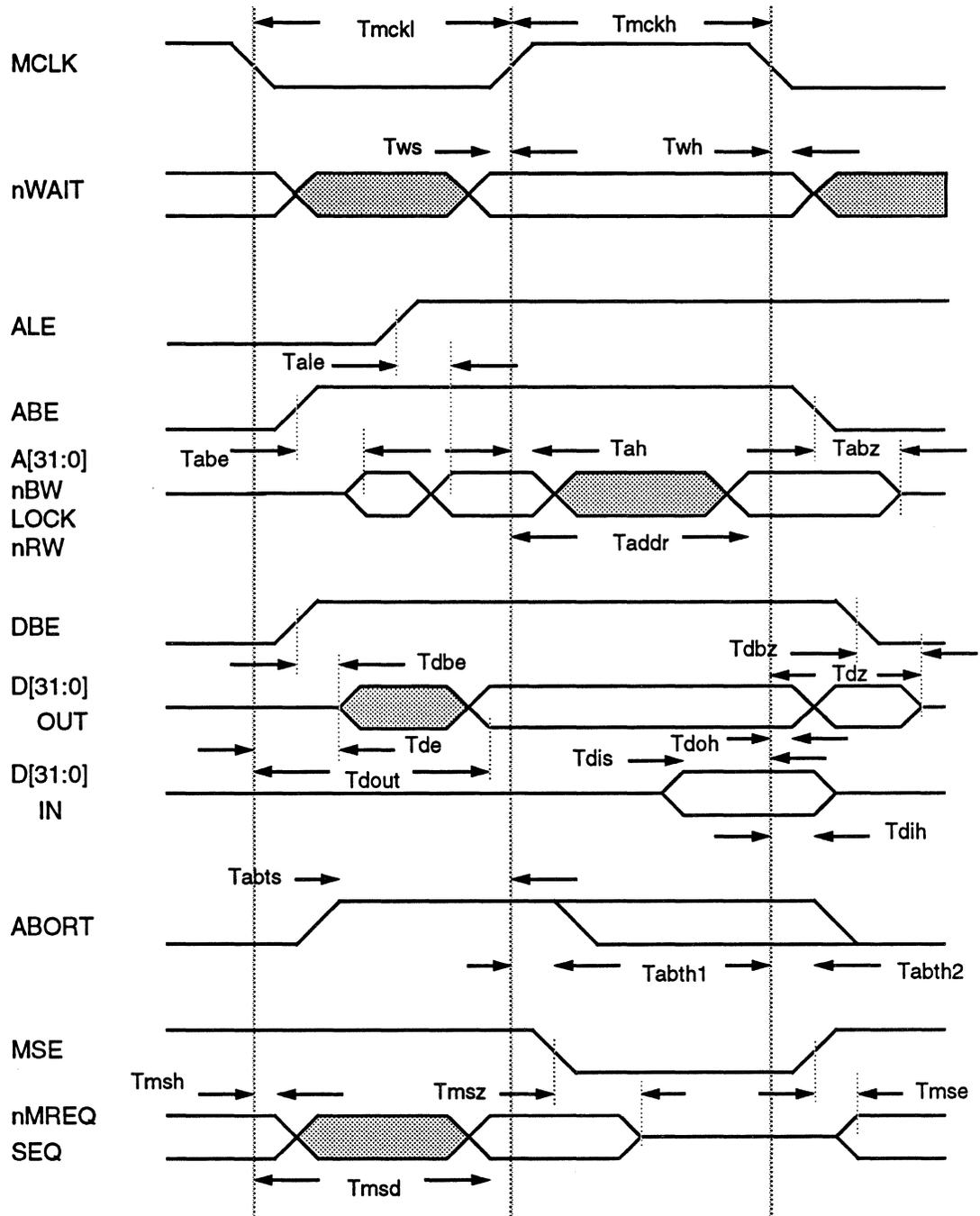
Figure 55: ARM610 Main Bus Timing
