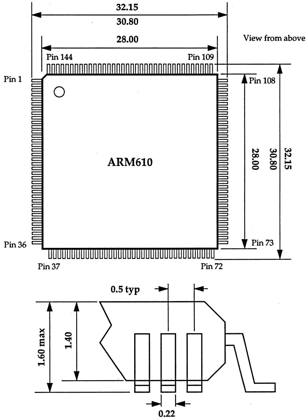
Figure 56: ARM610 144 Pin TQFP Mechanical Dimensions in mm
