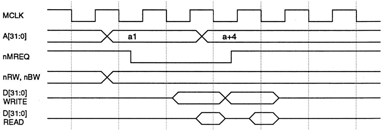
Figure 41: Two Word Sequential Read or Write
