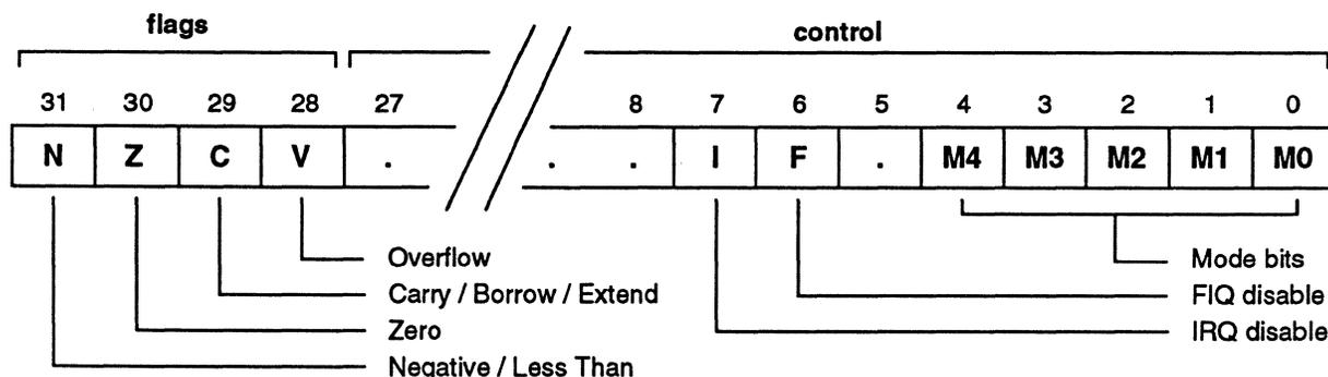
**Figure 4: Format of the Program Status Registers (PSRs)**
