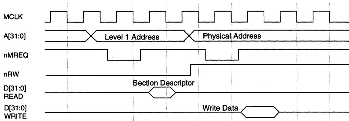
Figure 49: Translation Table-walking Sequence (write) For Section
