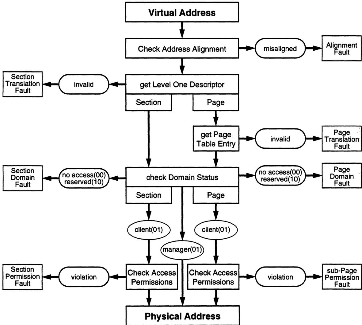
Figure 42: Sequence for Checking Faults
