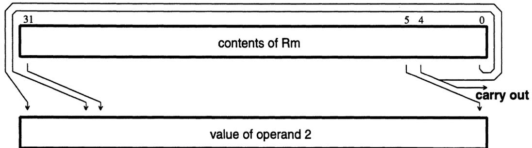
Figure 15: Rotate Right
