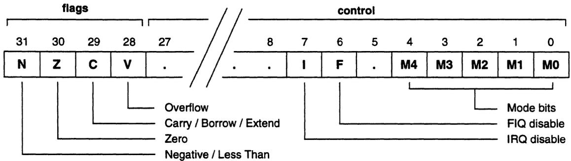
**Figure 6: Format of the Program Status Registers (PSRs)**
