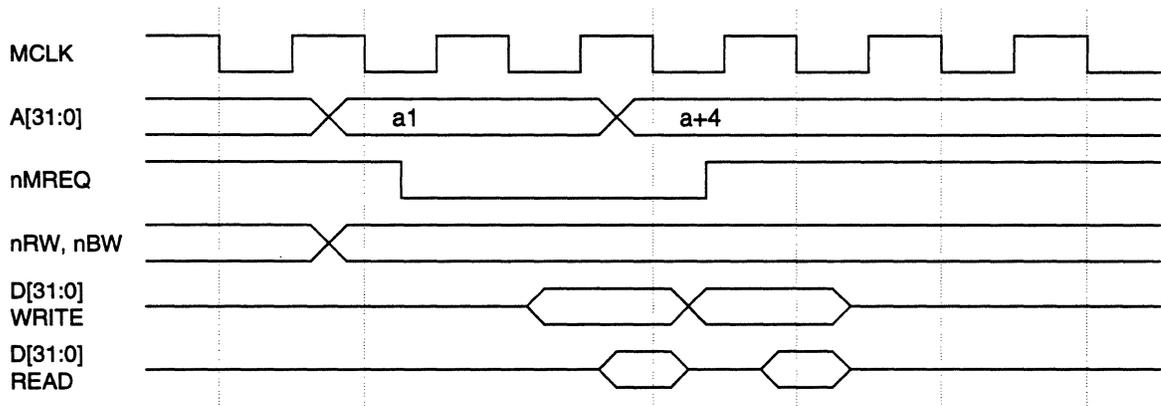
**Figure 44: Two Word Sequential Read or Write**
