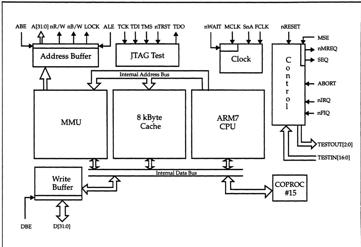
Figure 1: ARM710 Block Diagram
