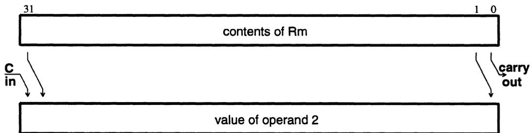
Figure 16: Rotate Right Extended
