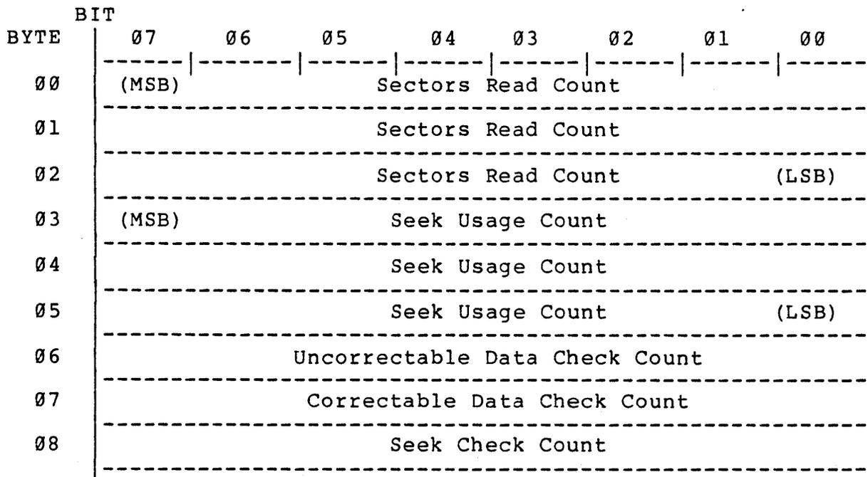
Figure 6-18. READ/RESET USAGE COUNTER Parameters
