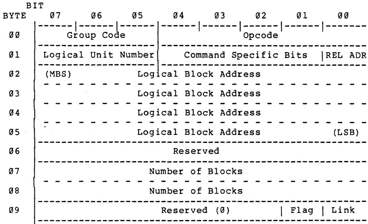
Figure 4-4. Group 1 Commands (10-Byte Extended Block Address)
