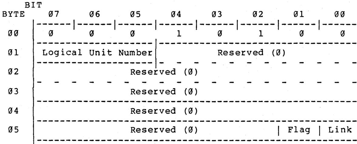
Figure 6-22. READ DATA BUFFER Command
