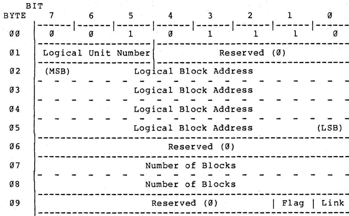
Figure 6-40. WRITE and VERIFY Command
