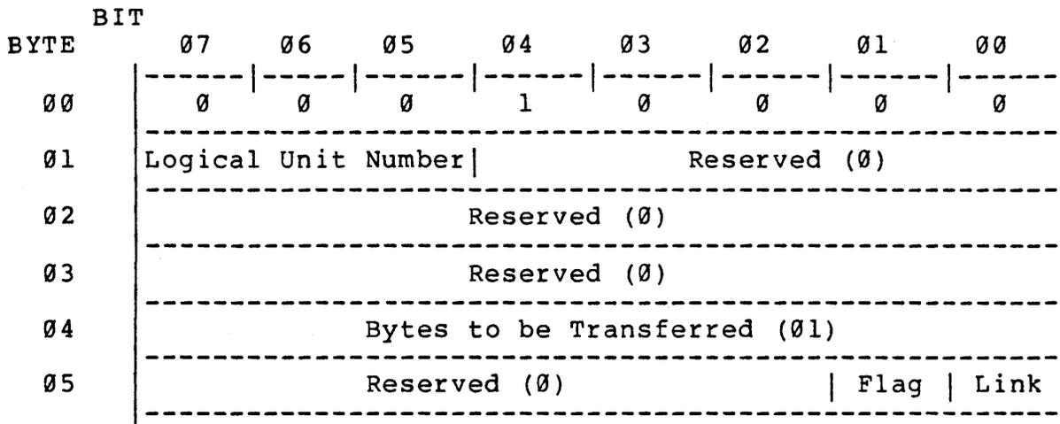
Figure 6-16. SET THRESHOLD Command
