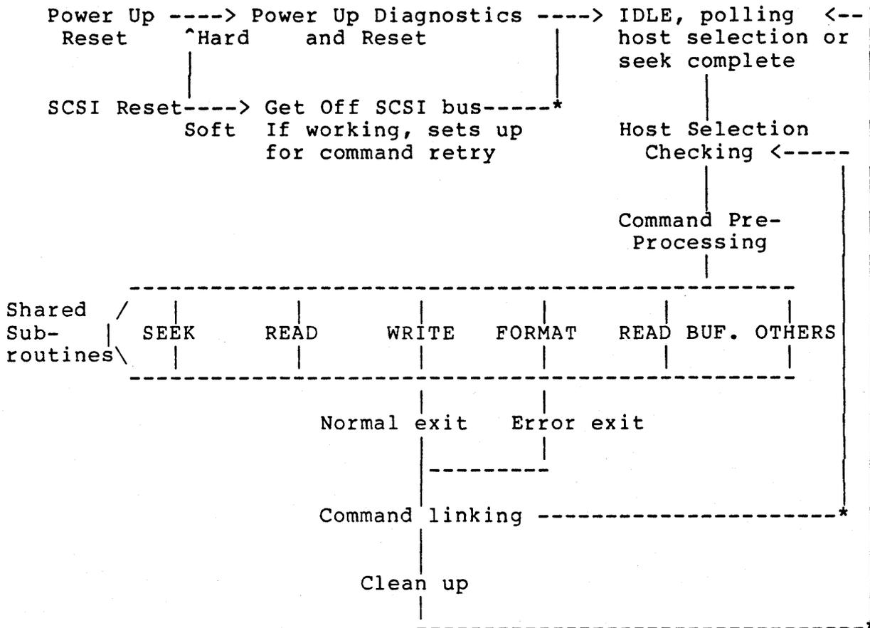
Figure 2-2. ACB-5500 Microcode Structure
