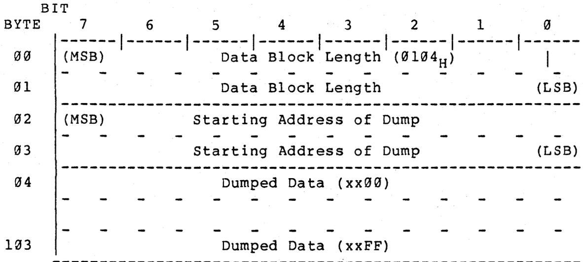
Figure 6-33. RECEIVE DIAGNOSTIC Data
