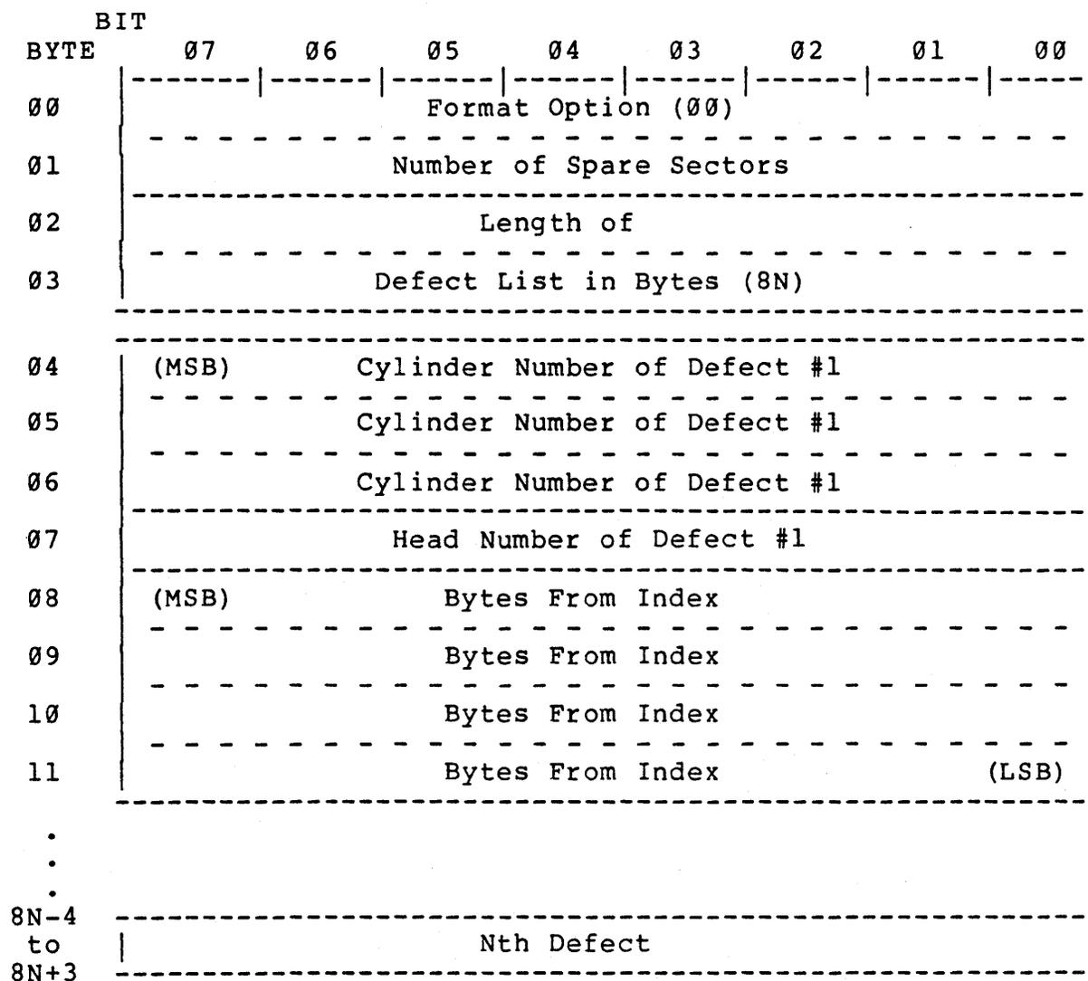
Figure 6-9. Format Unit Data Block (Drive Formatting)
