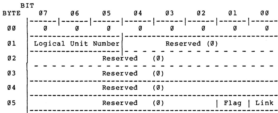
Figure 6-1. TEST UNIT READY Command
