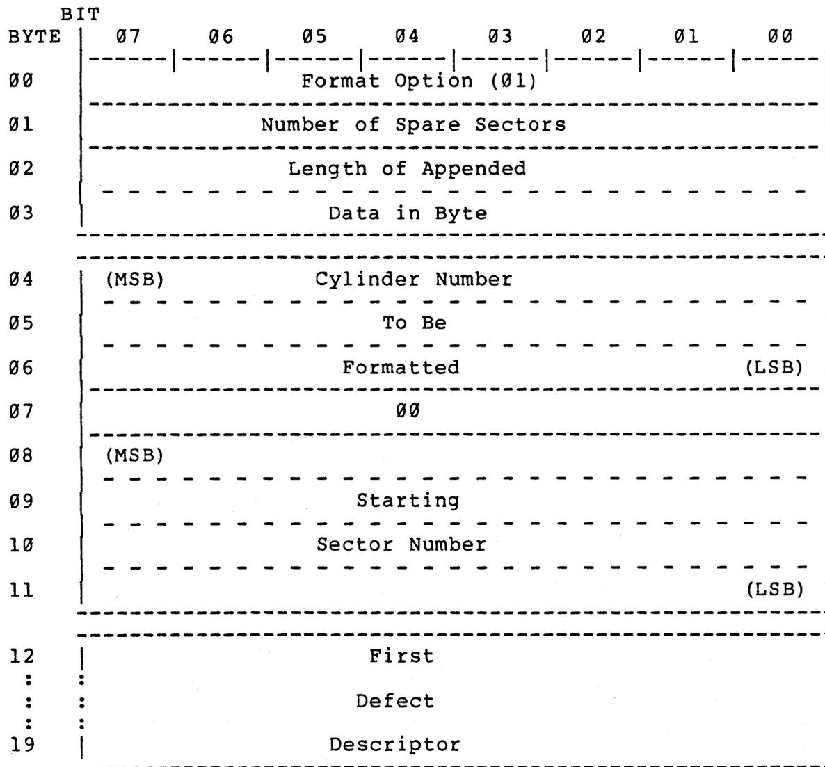
Figure 6-10. Format Unit Data Block
