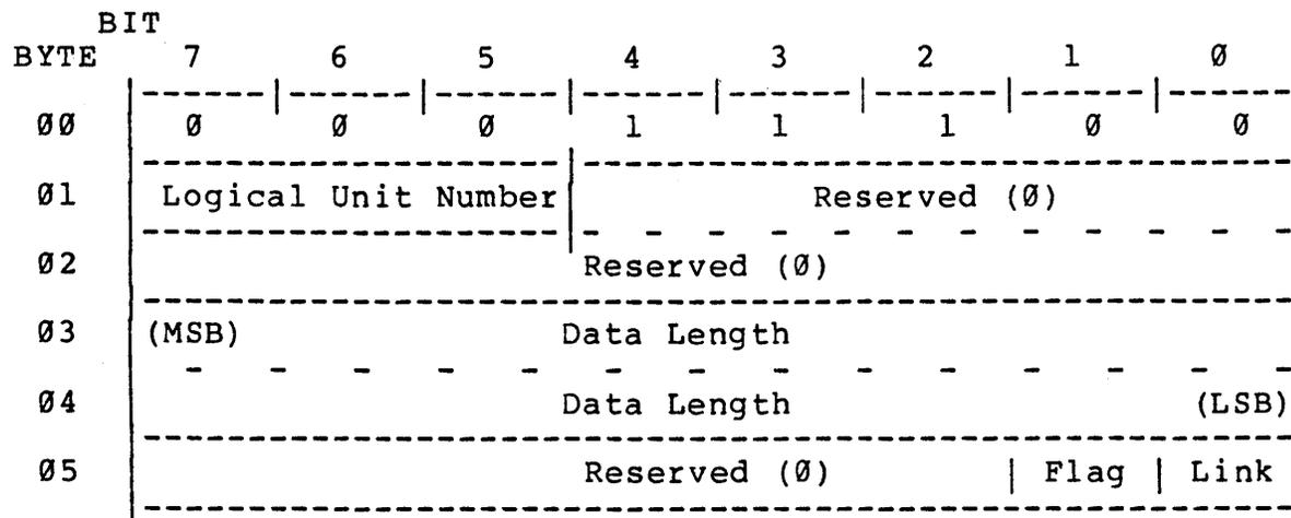
Figure 6-32. RECEIVE DIAGNOSTIC Command
