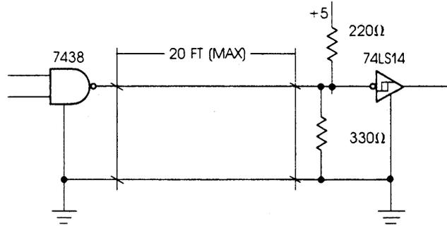
Figure 5-2. ST506 Control Signal Driver/Receiver Circuit
