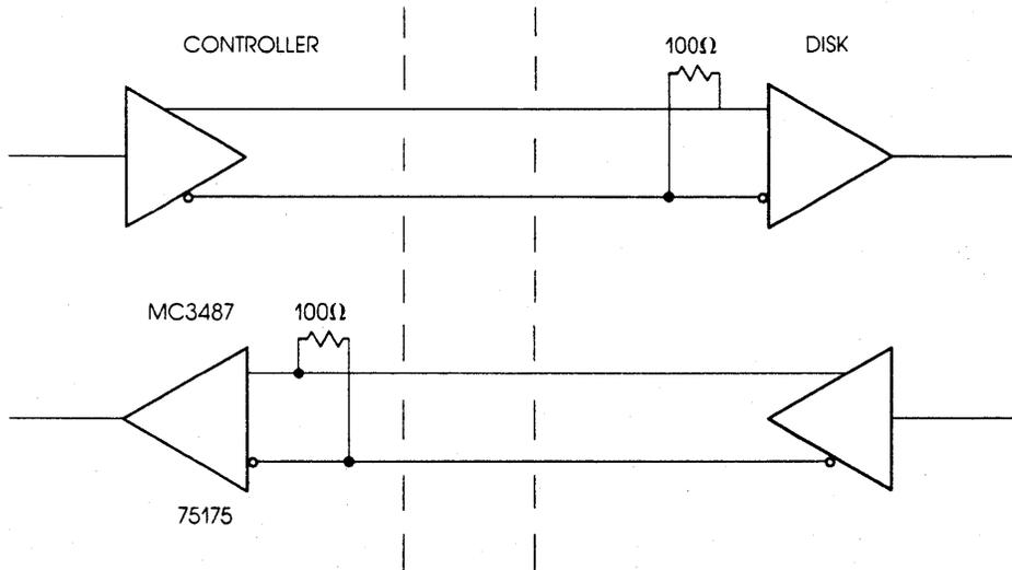
Figure 5-3. MFM Data Driver/Receiver Circuit
