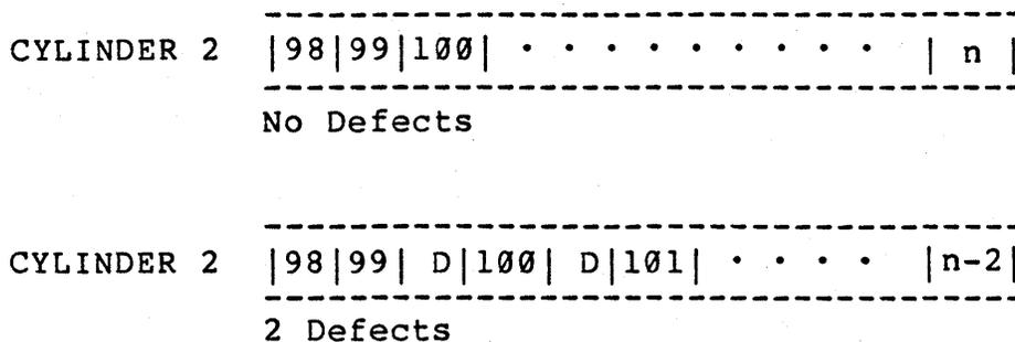
Figure 6-6. Sector Level Defect Skipping
