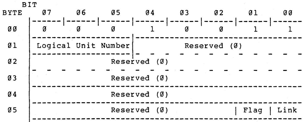
Figure 6-21. WRITE DATA BUFFER Command
