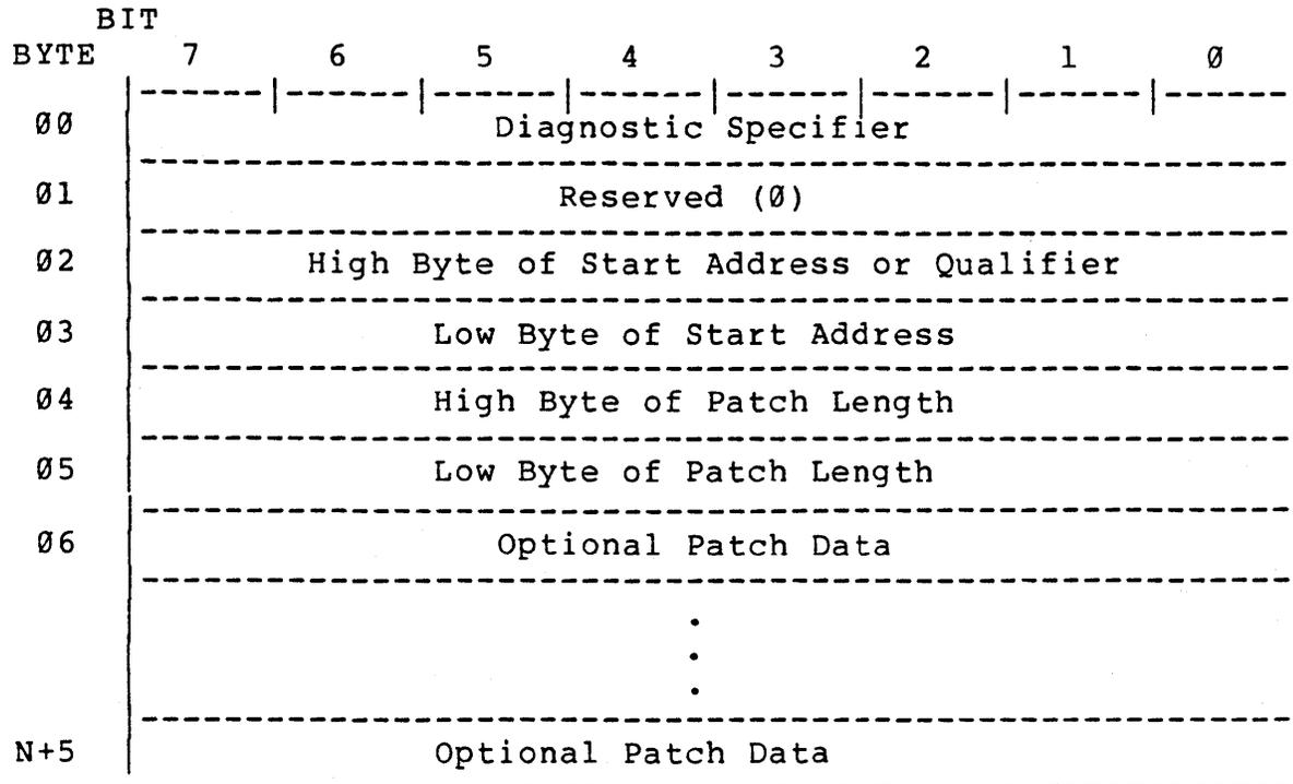
Figure 6-35. SEND DIAGNOSTIC Parameter Format
