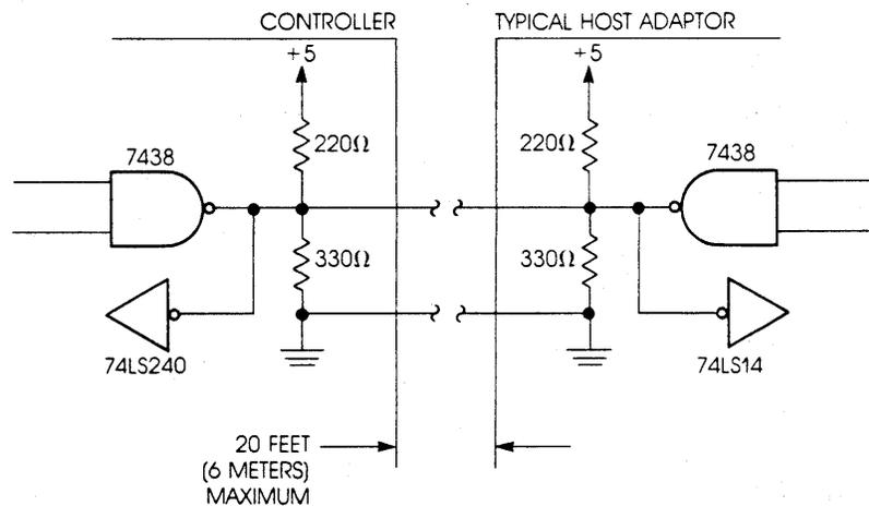
Figure 4-1. Host Adapter Bus Termination
