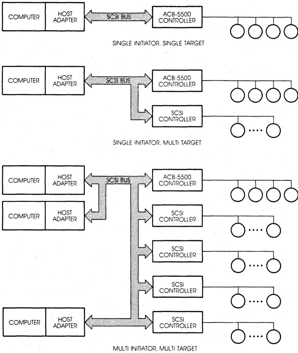
Figure 2-3. Typical SCSI Configurations
