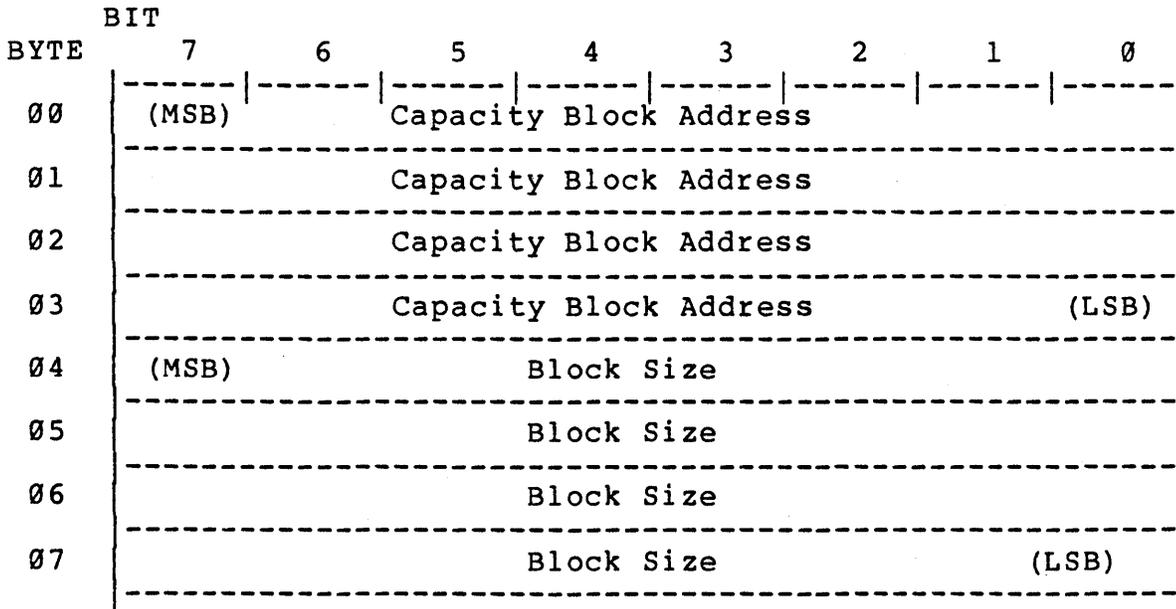
Figure 6-37. READ CAPACITY Parameters
