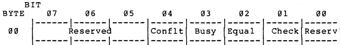
Figure 4-5. Completion Status Byte
