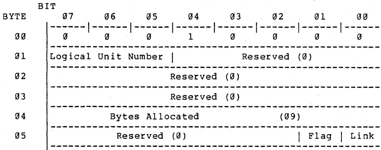
Figure 6-17. READ/RESET USAGE COUNTER Command
