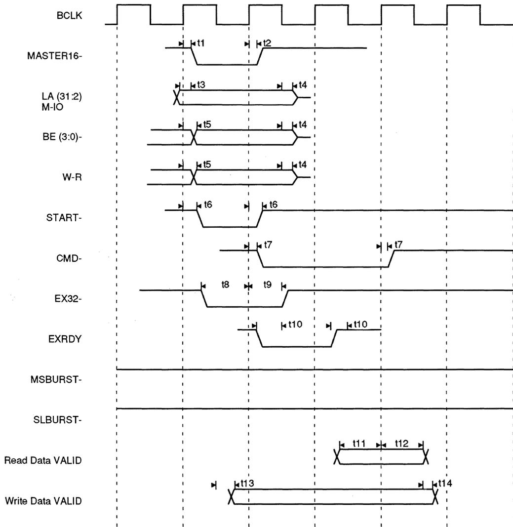
Figure 9-6. EISA Two Cycle Transfer – 32-bit
