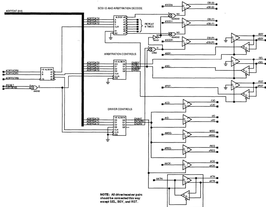
Figure 4-1. Differential Controls
