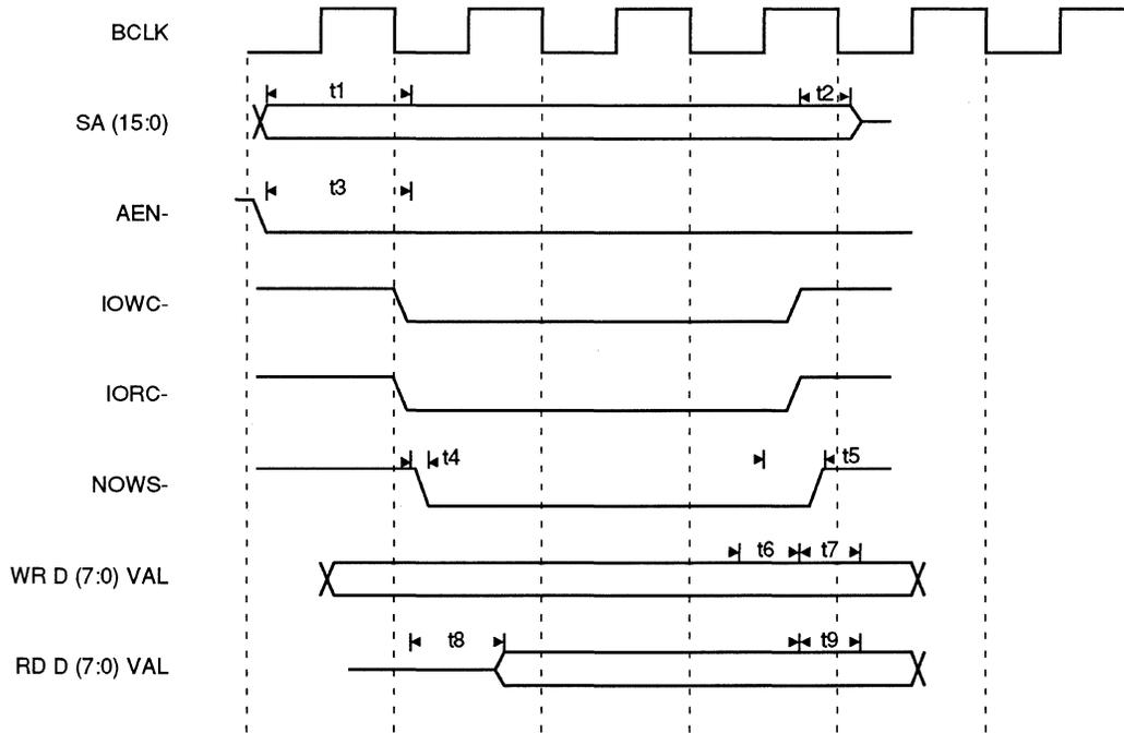
Figure 9-15. ISA I/O Slave – 8-bit Write/Read
