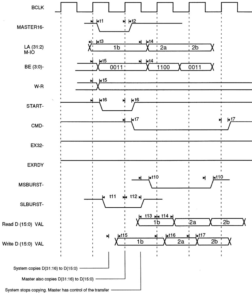
Figure 9-9. EISA Burst Transfer – 16-bit Downshift (System Copy)
