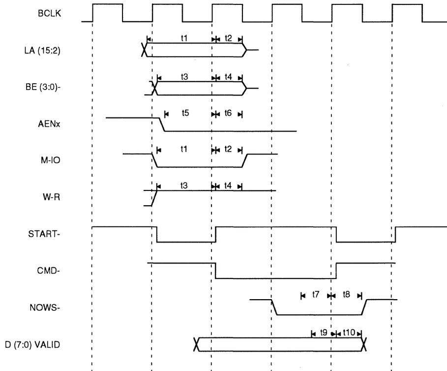
Figure 9-11. EISA I/O Slave – 8-bit Write
