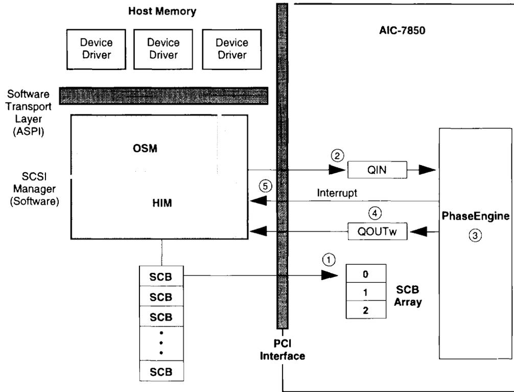
The typical sequence which the HIM uses to start a new SCB in the AIC-7850 is as follows:
