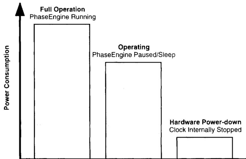
The PhaseEngine may place itself into Sleep Mode only when it is cycling in the idle portion of its instruction loop waiting for a SCSI phase change, a DMADONE status or a new SCB posting. When one of these occur, the PhaseEngine will wake up and begin processing the condition without interrupting the host driver.
