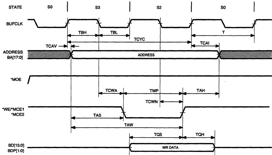
Figure 8-13 SRAM Timing (Write, 2T Access)
