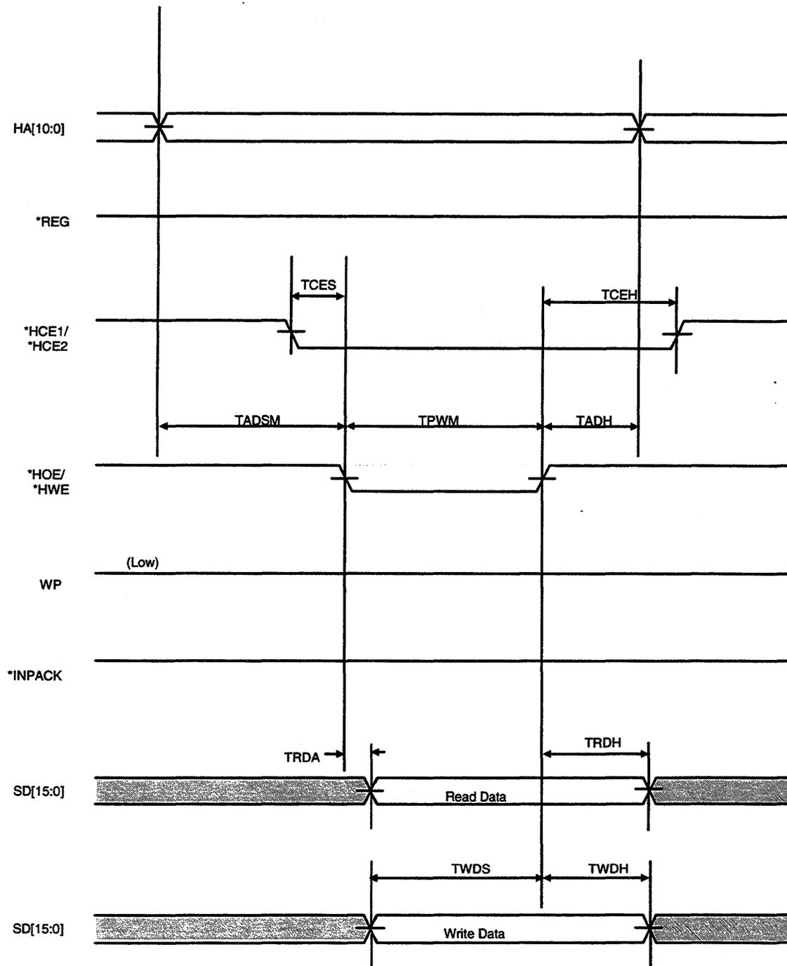
Figure 8-39 PCMCIA Block I/O Mode Timing
