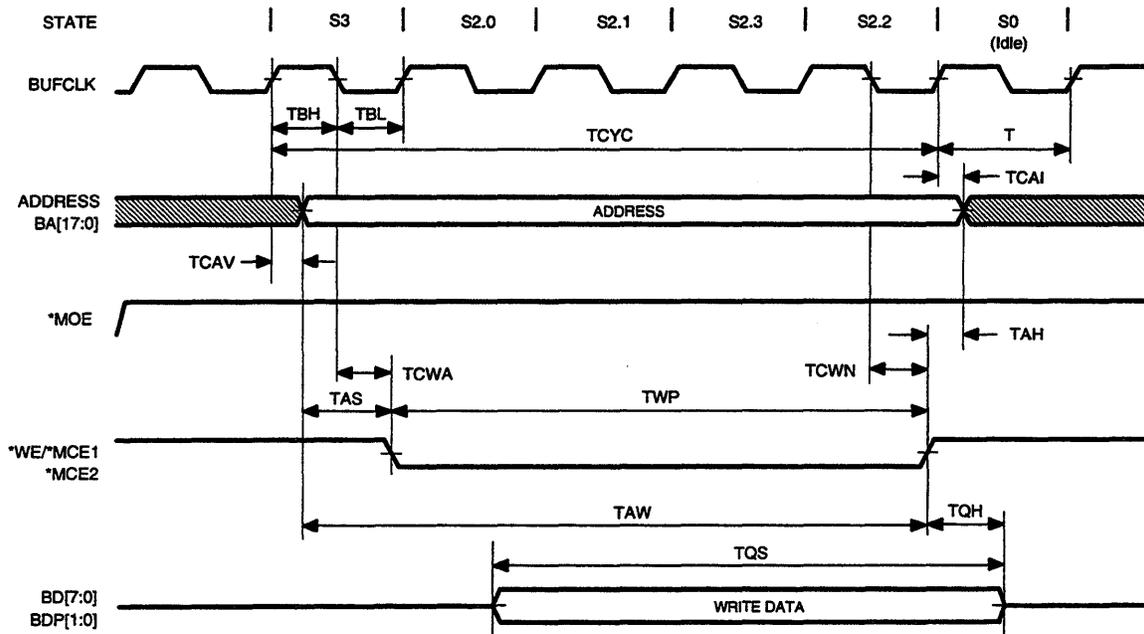
Figure 8-16 SRAM Timing (Write, 5T Access)
