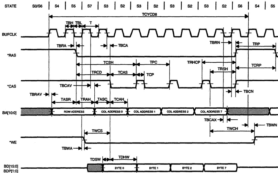
Figure 8-23 DRAM Timing (Page Mode, No Wait State, Write)
