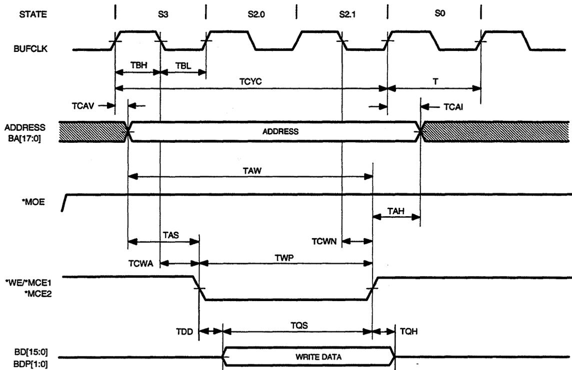
Figure 8-14 SRAM Timing (Write, 3T Access)
