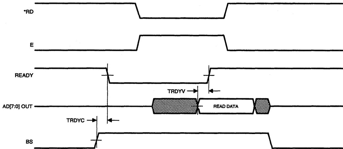
Figure 8-6 Microprocessor Ready Timing (Buffer RAM Read Cycle)
