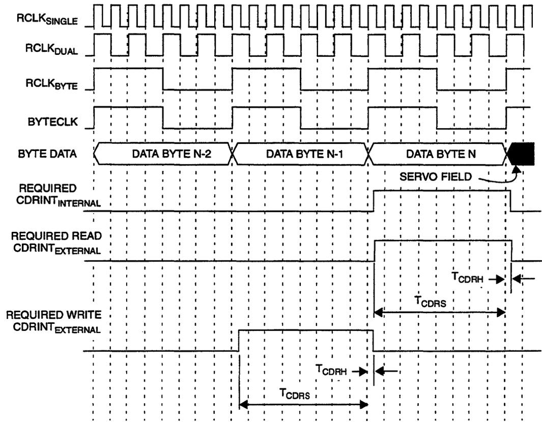
Figure 8-33 External CDR Interrupt Timing
