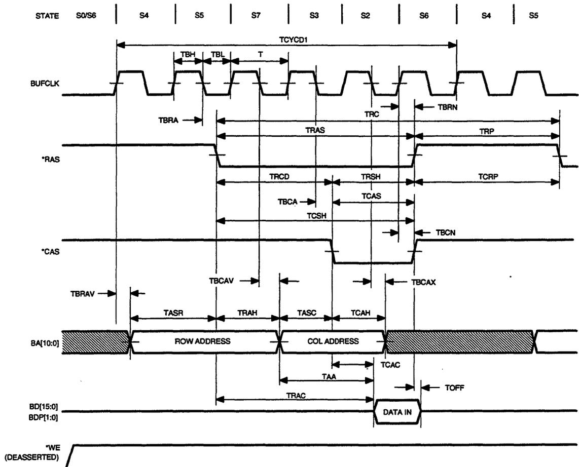
Figure 8-17 DRAM Timing (No Wait State, One Byte Read)
