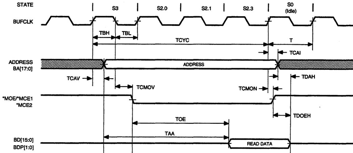
Figure 8-11 SRAM Timing (Read, 4T Access)
