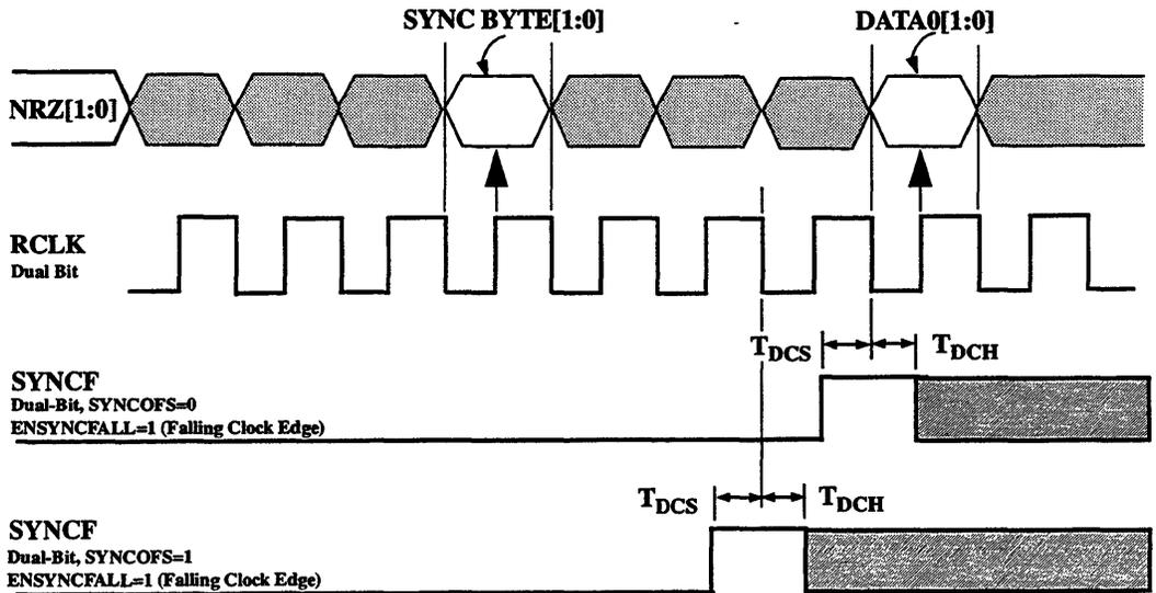
**NOTE:** SYNCF is shown for Sync Offset = 0 and =1. SYNCF can be internally delayed to get the alignment shown here. See DCTL1 Reg 61h, R/W, bits 2:0.
