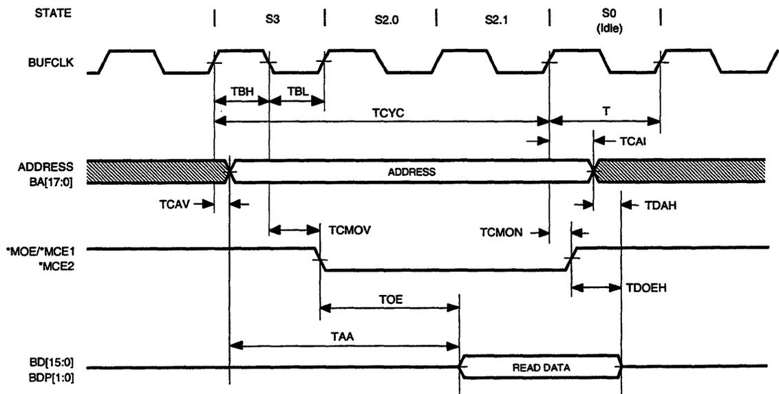
Figure 8-10 SRAM Timing (Read, 3T Access)
