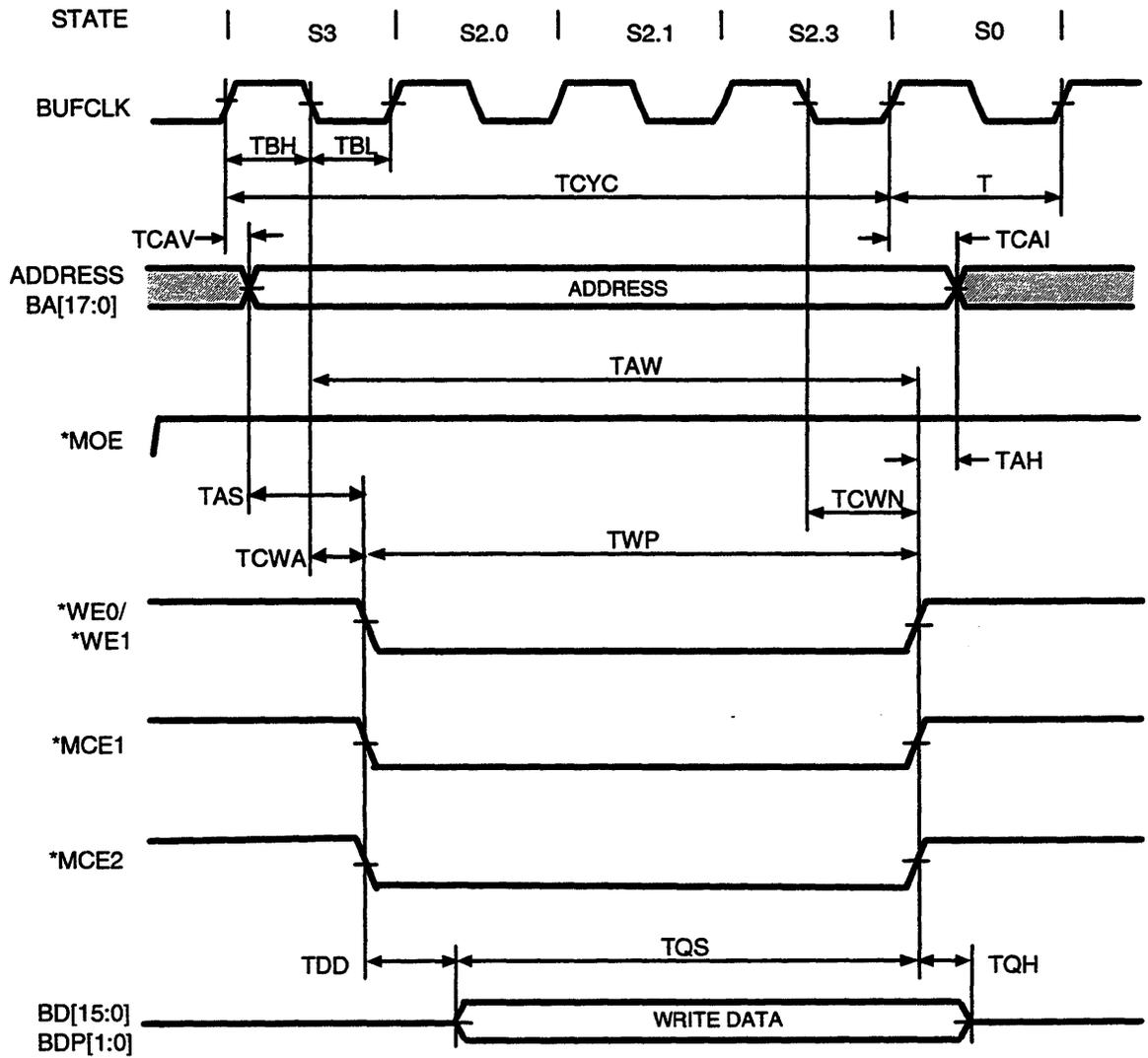
Figure 8-15 SRAM Timing (Write, 4T Access)
