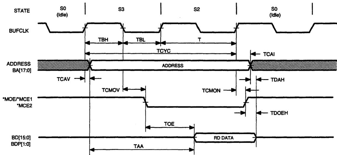
Figure 8-9 SRAM Timing (Read, 2T Access)
