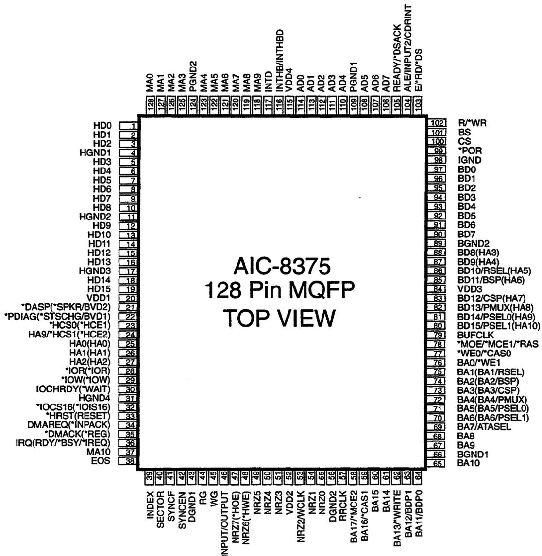
Figure 2-1 AIC-8375 MQFP Pin Assignments
