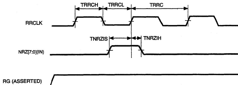
Figure 8-28 Eight-Bit: Disk Read Timing
