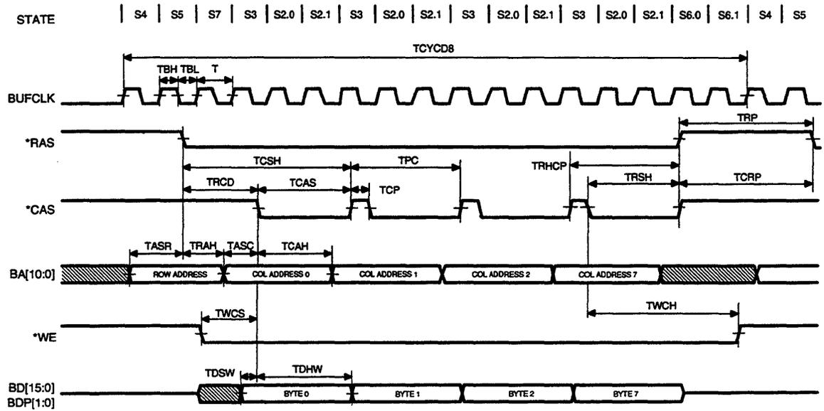
Figure 8-24 DRAM Timing (Page Mode, Wait State, Write)
