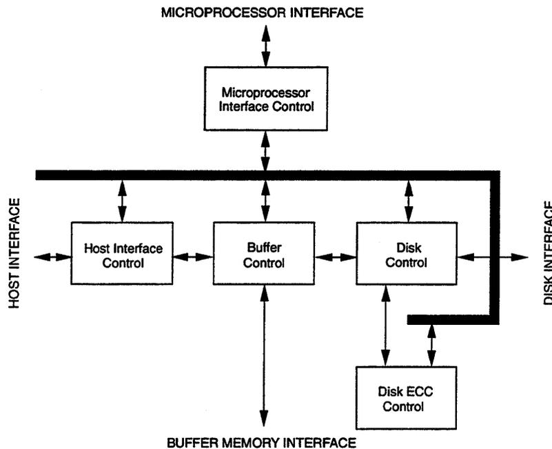
**Figure 1-1 AIC-8375 Block Diagram**
