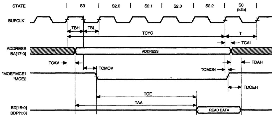
Figure 8-12 SRAM Timing (Read, 5T Access)
