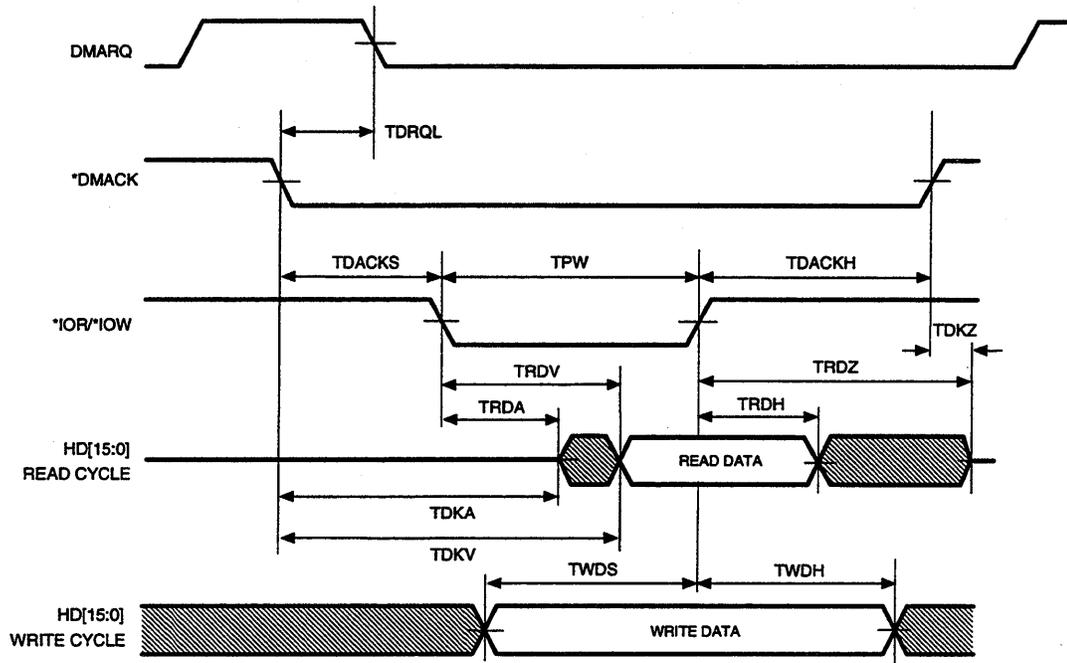
Figure 8-35 AT Single-Word DMA Timing
