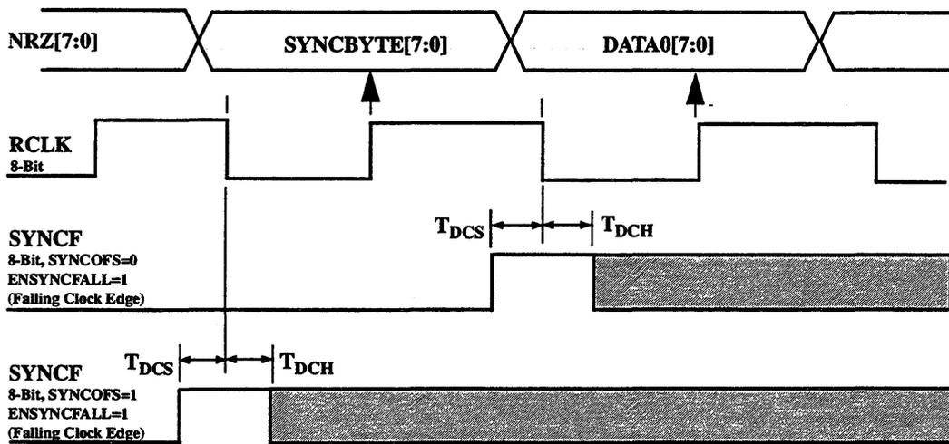
**NOTE:** SYNCF is shown for Sync Offset = 0 and =1. SYNCF can be internally delayed to get the alignment shown here. See DCTL1 Reg 61h, R/W, bits 2:0.
