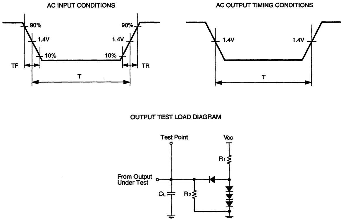
**Figure 8-1 AC Input/Output Timing**
