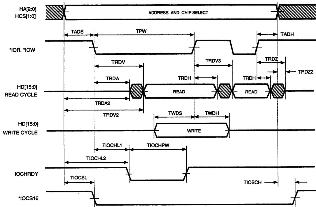
Figure 8-34 AT PIO Timing
