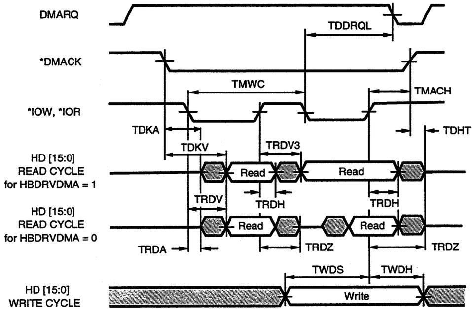
Figure 8-36 AT Multi-Word DMA Timing
