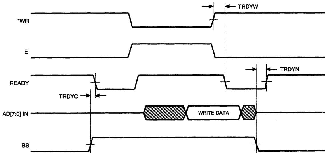
Figure 8-7 Microprocessor Ready Timing (Buffer RAM Write Cycle)
