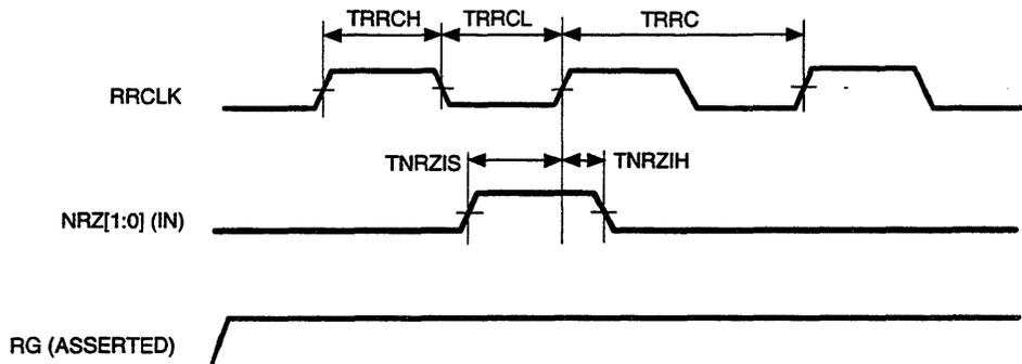
Figure 8-27 Single- and Dual-Bit: Disk Read Timing
