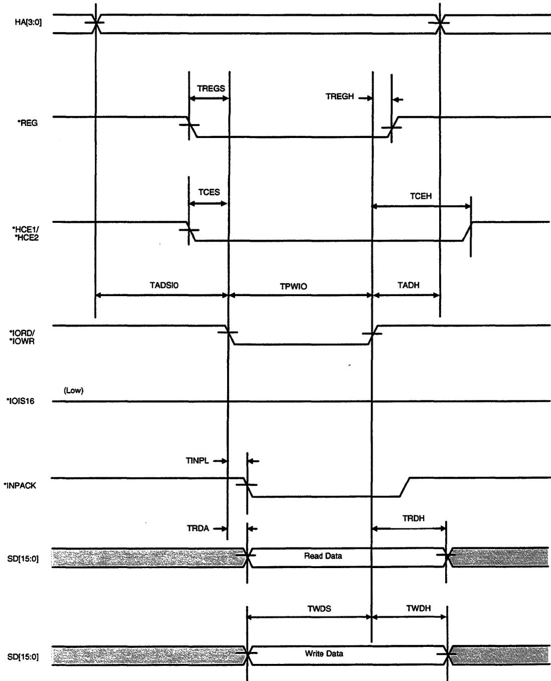
Figure 8-38 PCMCIA Primary/Secondary I/O Mode Timing
