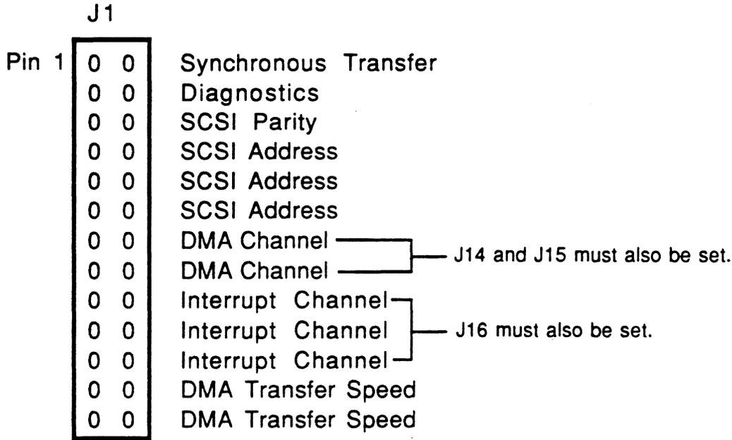
Jumper block J1 is the large vertically oriented block of jumpers located near the center of the host adapter. Pin pair 1 is the topmost pair of pins.
