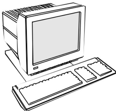
This terminal can emulate a number of ASCII and ANSI terminals, including PC-Term. The keyboards supported by the terminal are the 101/102 key Extended-PC (EPC), the 106/107 PC/+, and the ASCII keyboards.
