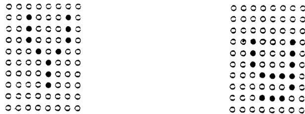
Figure 3-3 Detail of Character Dot Matrix Construction
