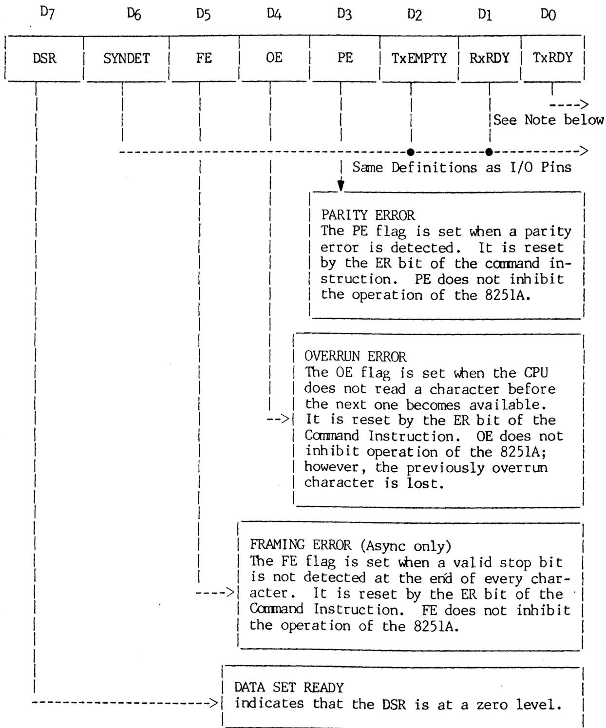
Note: TxRDY status bit has different meanings from the TxRDY output pin. The former is not conditioned by  $\overline{CTS}$  and TxEN; the latter is conditioned by both  $\overline{CTS}$  and TxEN.
