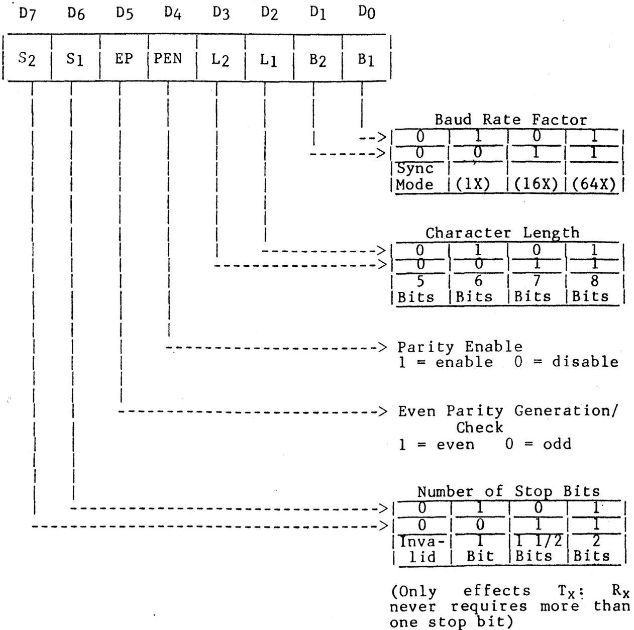
Figure 2-2. Mode Instruction Format - Asynchronous
