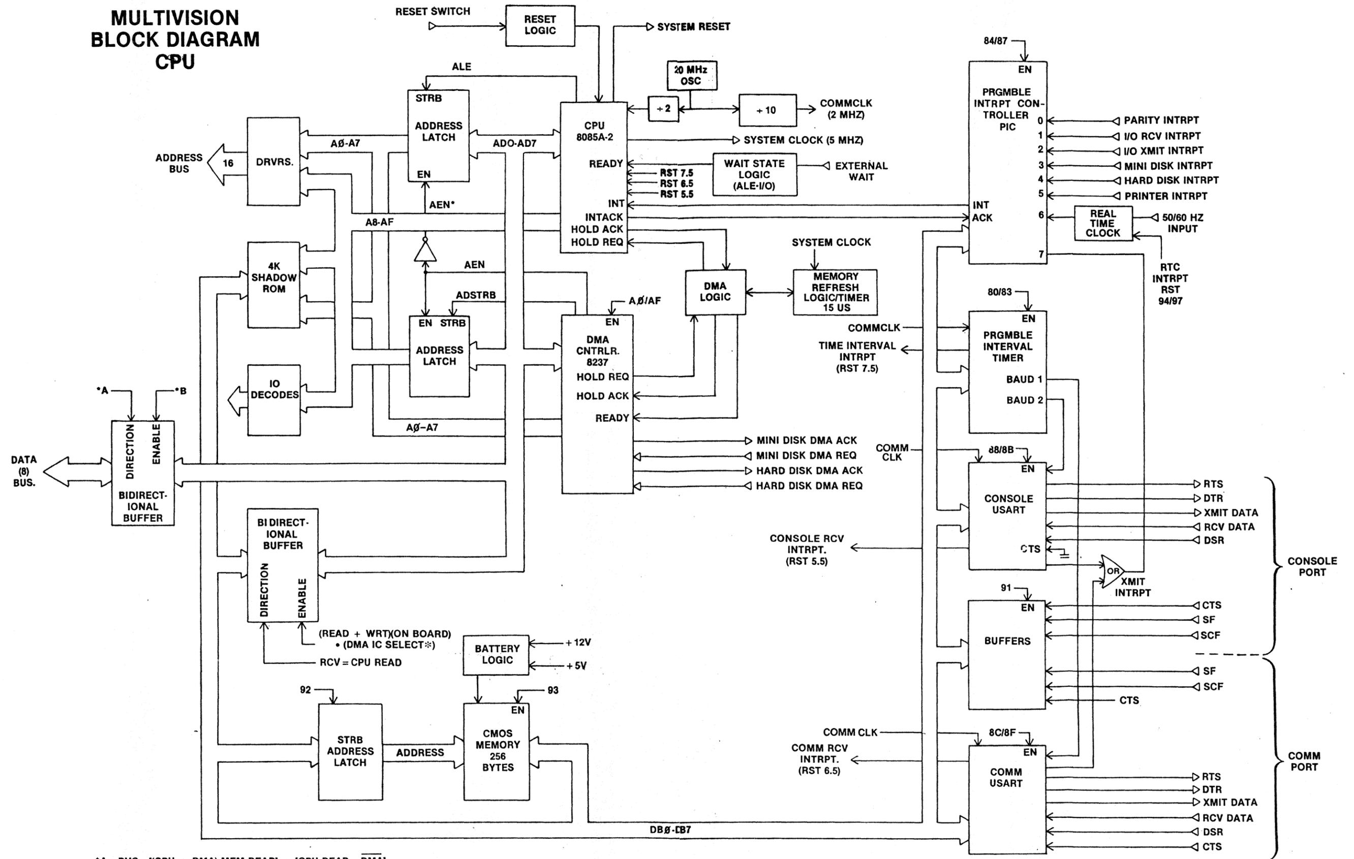
\*A  $RVC = [(CPU + DMA) MEM READ] + [CPU READ \cdot \overline{DMA}]$
