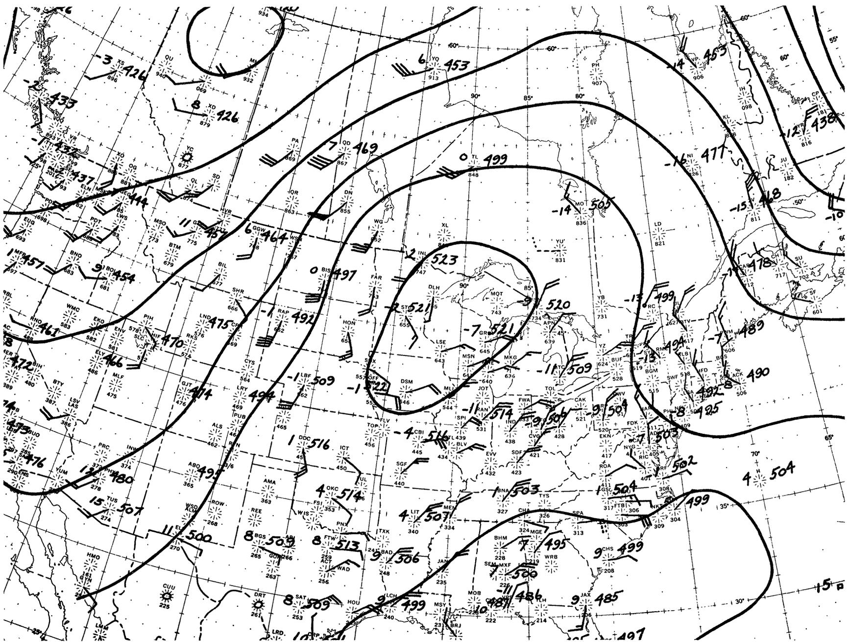
Fig. 2—Typical plot and conventional analysis of meteorological data. The plotted data refer to wind, temperature, and height of the 850 mb surface for 1500 Greenwich Meridian Time, November 5, 1953; the "analysis" consists of smoothed height contours of the 850 mb surface. (Turn to read)
