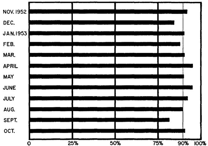
Fig. 7—Monthly reliability coefficients for Project Cyclone Simulation Laboratory (average for first year 90.6 per cent).
