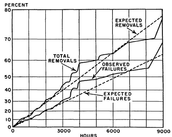
Fig. 11—Tube mortality with time, shipborne equipments.
