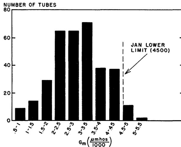
Fig. 2— $G_m$  distribution of 12AT7 removals from land-based teletype equipment.
