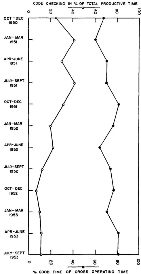
Fig. 1—Graph of operating efficiency of SEAC from October, 1950 to March, 1953.
