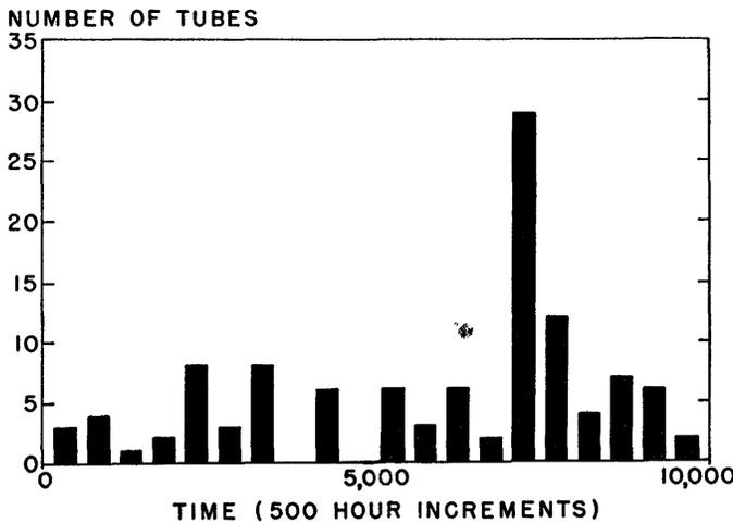
Fig. 8—6SK7 removals from land-based receivers by 500-hour periods.
