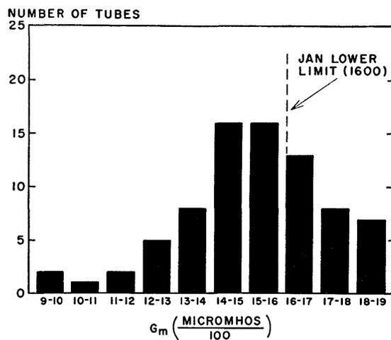
Fig. 3— $G_m$  distribution of 6SK7 removals from land-based communications receivers.
