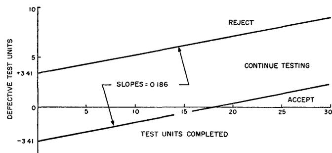
Fig. 1—Chart for controlling the sequential test. Slopes and intercepts are determined by the specified probabilities.
