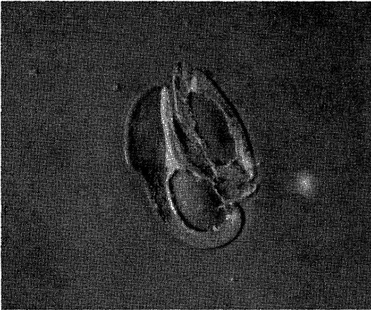
Fig. 5—This photomicrograph (magnified 25 times) illustrates appearance of a defect in acetate backing of magnetic tape. This irregularity is reflected in magnetic coating and gives rise to an error.
