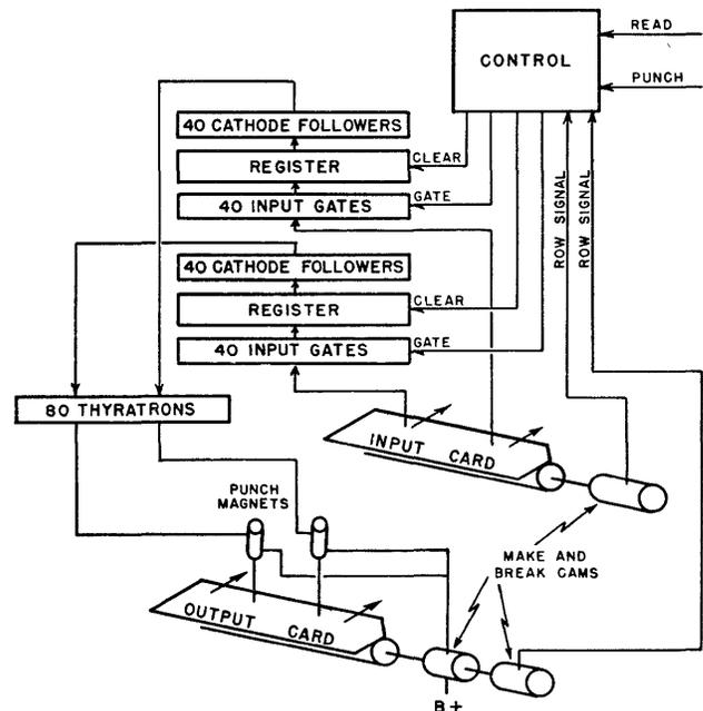
Fig. 3—Block diagram of the card input-output system.
