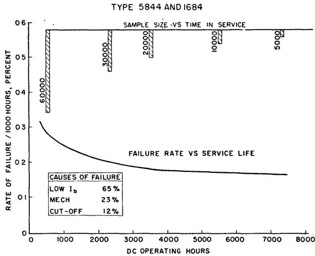
Fig. 7—Failure rate vs service life for tube types 5844 and 1684.
