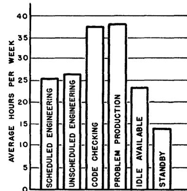
Fig. 2—Machine-time classification chart for an average week.
