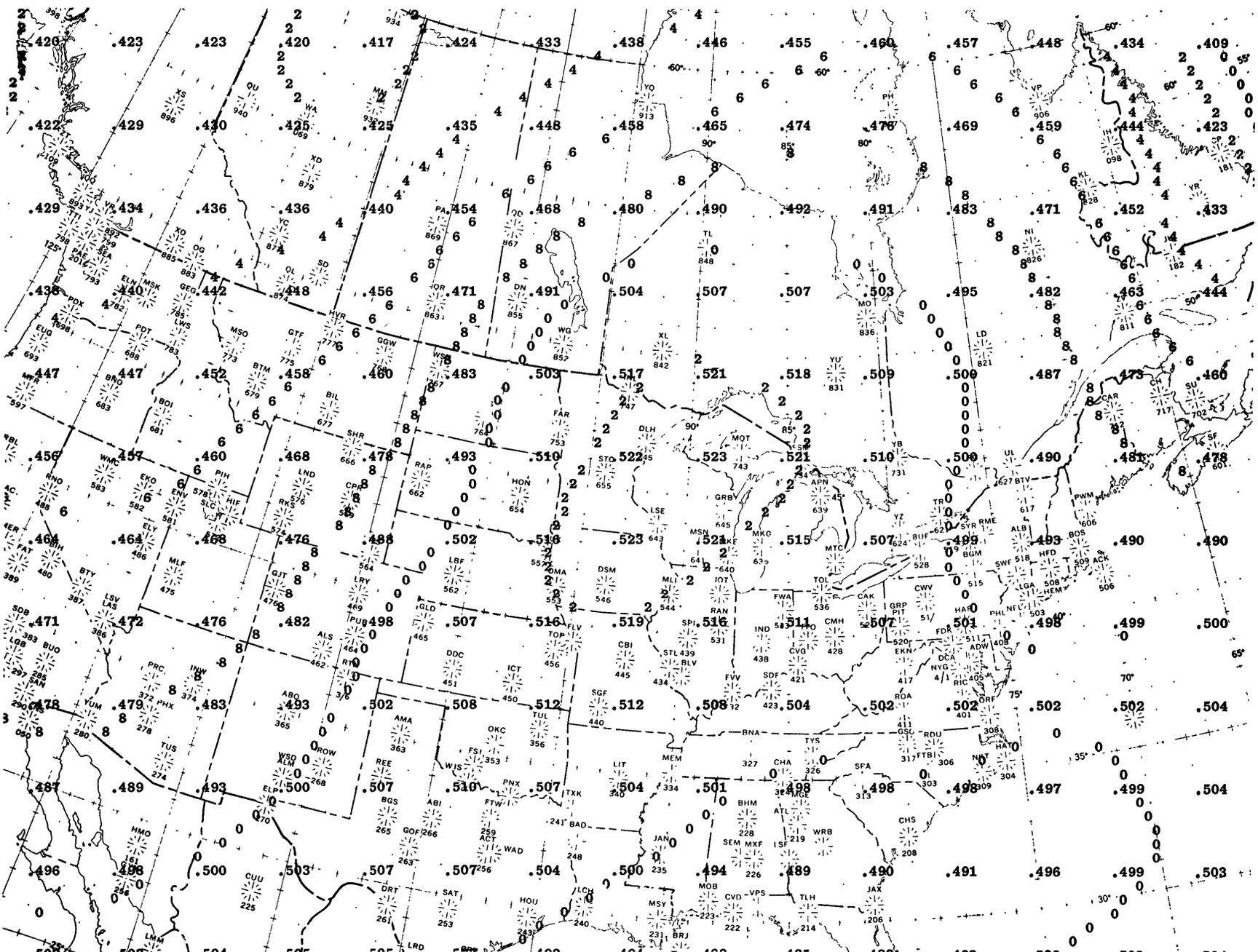
Fig. 3—Appearance of a computer controlled printing of an objective analysis of the data in Fig. 2. Shown are smoothed heights interpolated at grid points of a typical numerical prediction mesh, and contour lines. (Turn to read)
