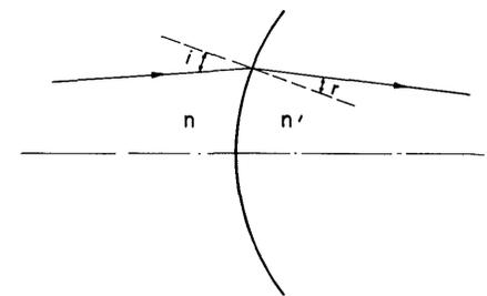
Fig. 6. Snell's law of refraction at a surface
