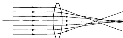
Fig. 5. Ray traces illustrating spherical aberration
