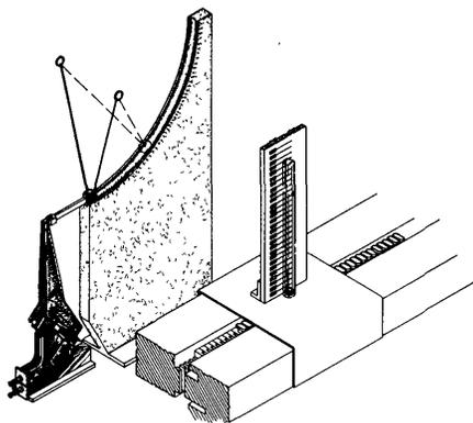
**Fig. 9. A ballistic pendulum was used to measure the actuator-hammer efficiency**
