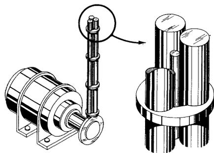
**Fig. 7. A test setup employing three brass rods as guides for various weights of hammers dropped against a rotating motor-driven typewheel**
