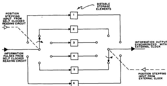
Fig. 10. Block diagram of synchronizer for use with self-clocked cancellation method of reading
