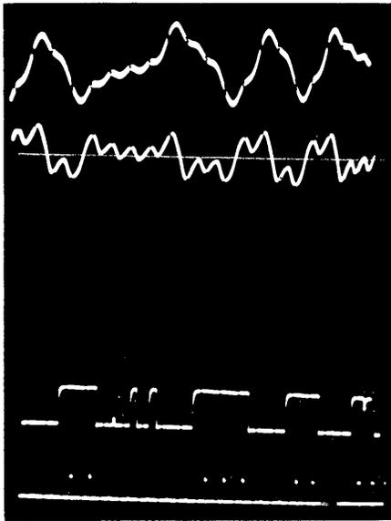
Fig. 5. Waveforms occurring in externally clocked, cancellation reading system. Relative packing density of 6m, absolute packing density of 880 bits per inch with head in contact with medium
