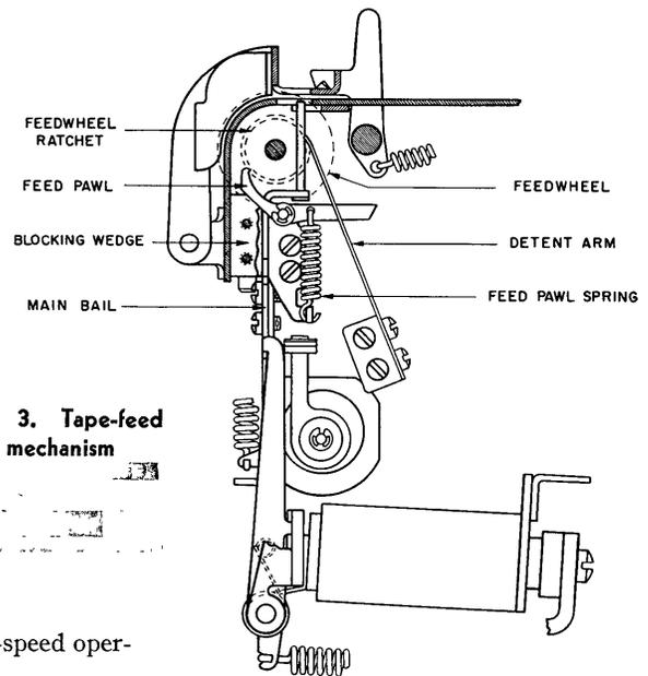
Fig. 3. Tape-feed mechanism
