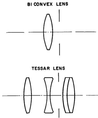
Fig. 3. Optical schematics of simple biconvex lens and Tessar lens
