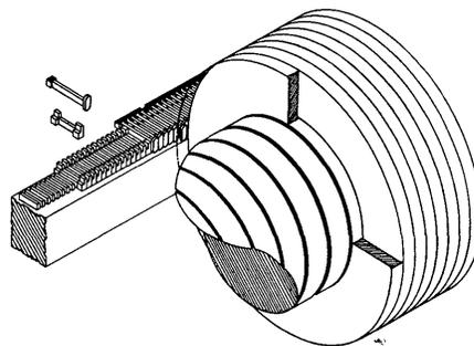
**Fig. 11. The shaft in which the typewheels are stacked is grooved so that a snap-ring can hold each pair of typewheels together. Nylon inserts provide bearing surface for the hammers**
