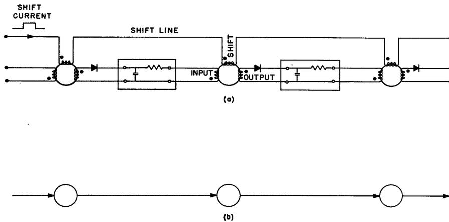
Fig. 3. Single-line shift register
