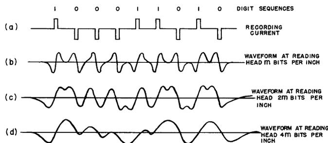
Fig. 1. RZ recording current, and waveforms at reading head for three different relative packing densities
