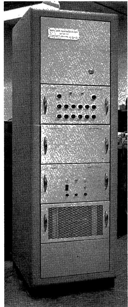
Fig. 3. Tape-to-card conversion unit (storage register)
