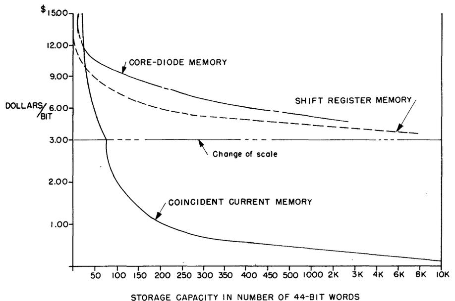
Fig. 2. Production cost of memory versus storage capacity
