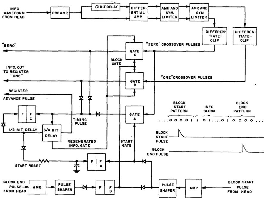
Fig. 9. Block diagram of test circuit for self-clocked cancellation method of reading
