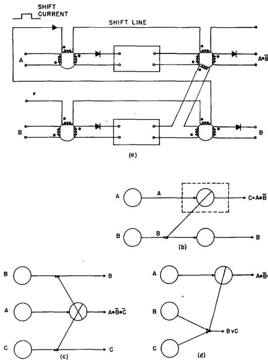
Fig. 5 (left). Inhibit circuits
