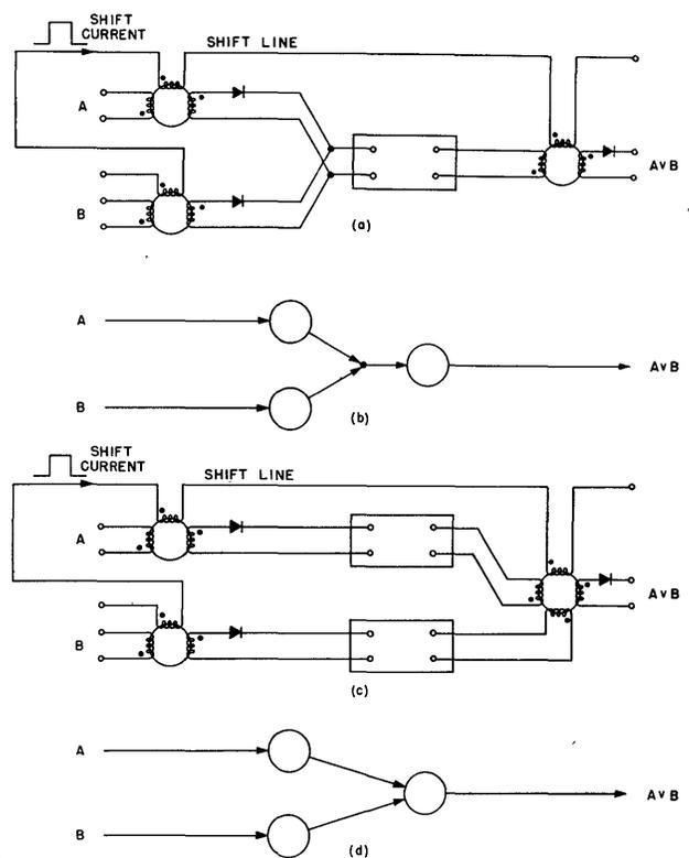
Fig. 6 (right). Mixing or buffer circuits
