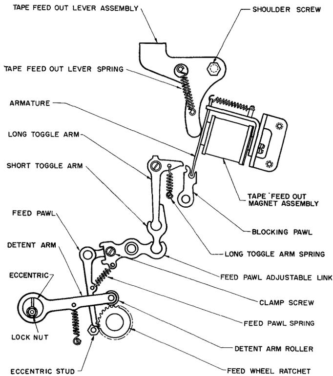
Fig. 6. Tape-feed mechanism
