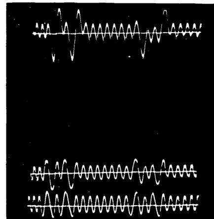
Fig. 7. Comparison between RZ (left) and double-pulse RZ (right) recording methods. Reading head waveforms, cancelled waveforms, and waveforms after a second cancellation operation. Relative packing density of 6m, absolute packing density of 880 bits per inch with head in contact with medium
