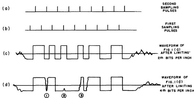
As a result, the waveform is frequently not of the correct polarity to be successfully sampled by a periodic sampling pulse.
