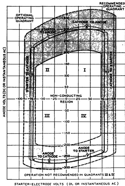
Fig. 3. Breakdown characteristics for type 5823 tube
