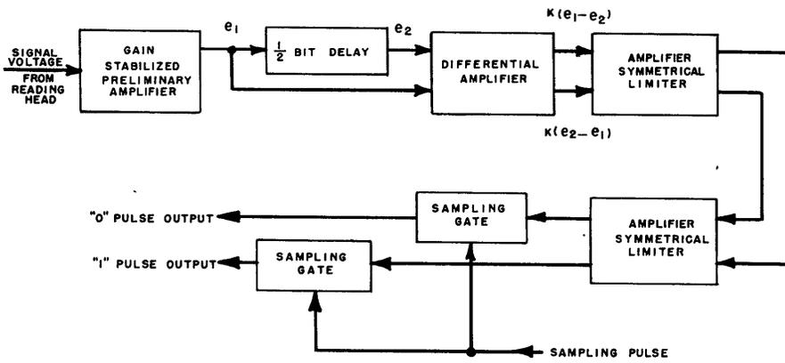
Fig. 4. Block diagram of externally clocked, cancellation reading system
