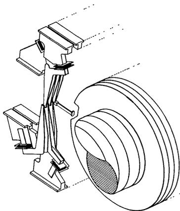
**Fig. 10. A cross section of the actuator assembly showing how the actuators are arranged in an 8-way interlace**
