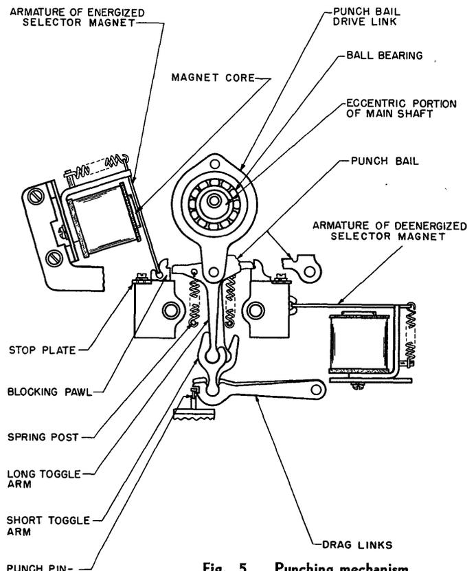
Fig. 5. Punching mechanism
