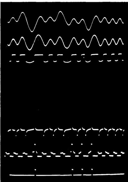
Fig. 8. Waveforms occurring in self-clocked, cancellation method of reading. Relative packing density of 6m, absolute packing density of 880 bits per inch
