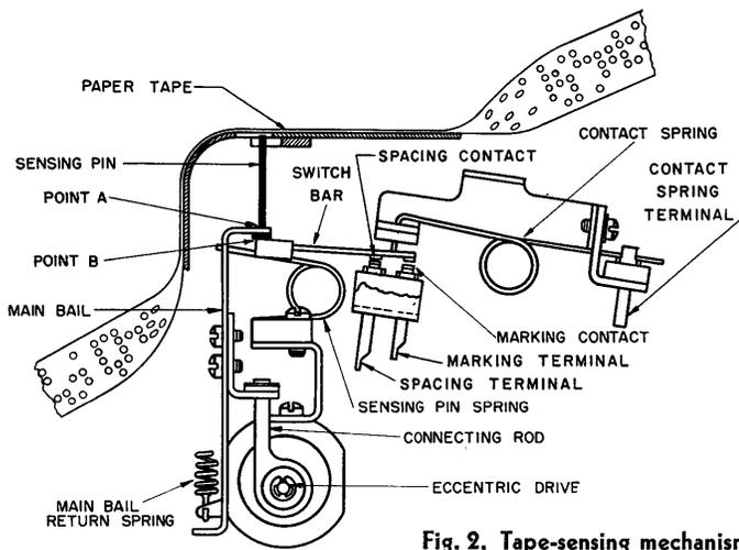
Fig. 2. Tape-sensing mechanism
