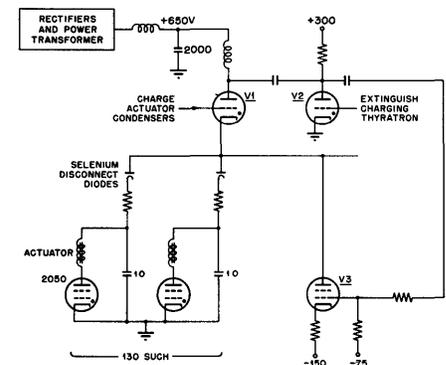
Fig. 5. Simplified schematic of the print circuits
