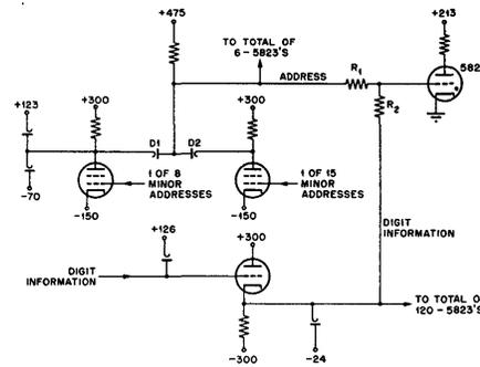
Fig. 4. Simplified schematic of read-in circuits
