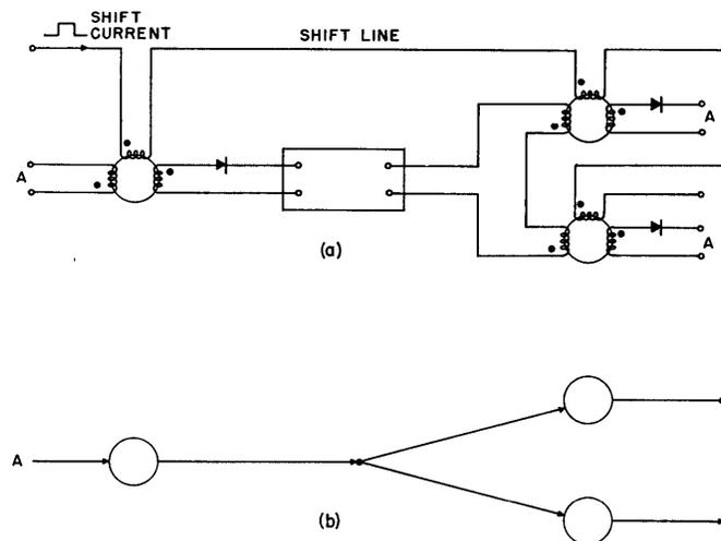
Fig. 4. Amplifier or branch circuit
