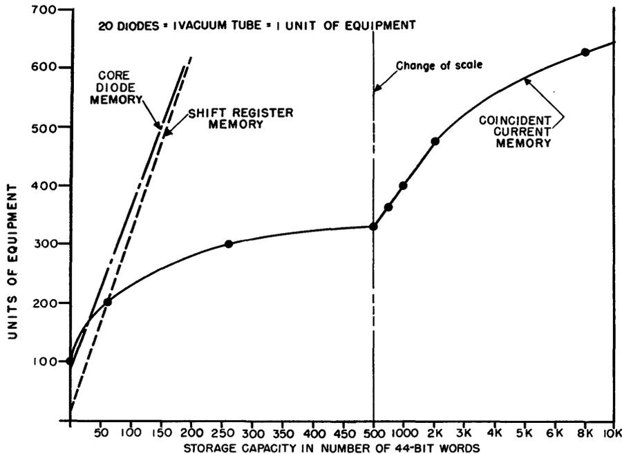
Fig. 1. Amount of equipment versus storage capacity
