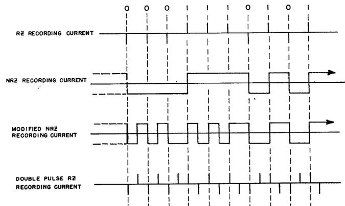
Fig. 6. Head-current waveforms for four methods of magnetic recording
