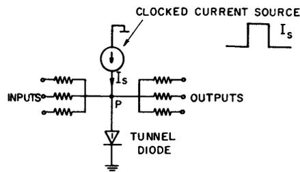
Fig. 16—Tunnel diode bistable logic element (single diode type).
