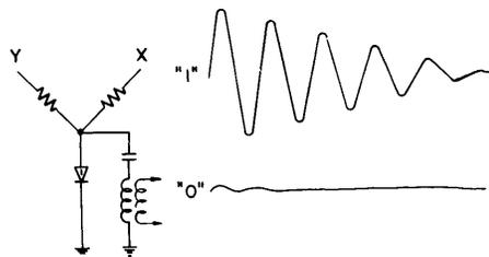
Fig. 21—Read out by sensing ringing.
