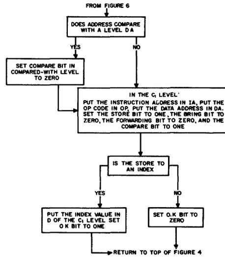
Fig. 6(b)—Logical conditions for store type operations.
