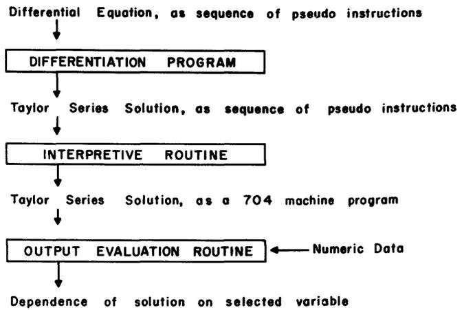
Fig. 7—Data flow for solution of differential equation.
