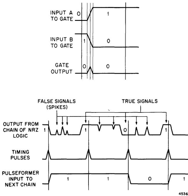
Fig. 5(a)—“Spike” formed due to overlap of gating signals. 5(b)—Discrimination against “spikes” occurring in a NRZ system using clocking methods.
