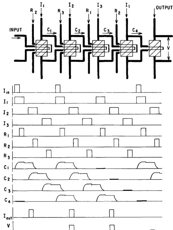
Fig. 8—Calculated waveforms for shift register.
