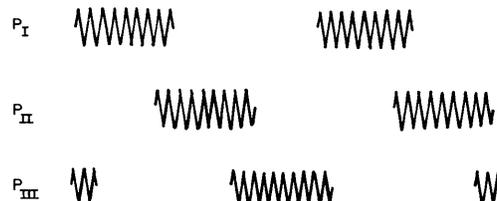
Fig. 3—Shift register with three-phase pump system.
