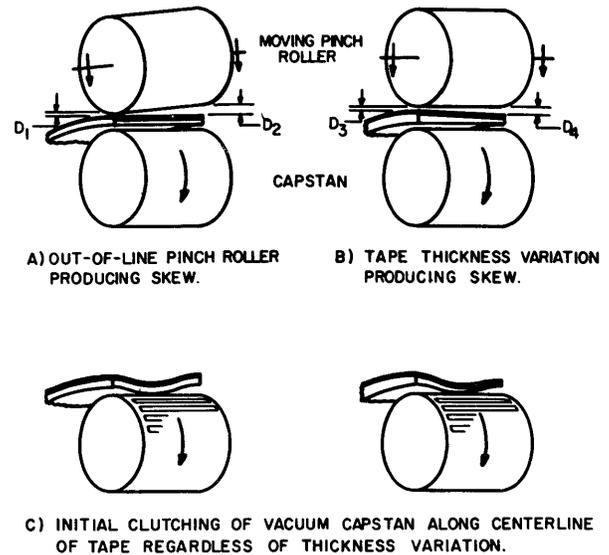
Fig. 6—Skew considerations for pinch rollers and vacuum capstans.
