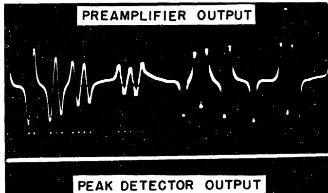
Fig. 11—Read system waveforms, including deliberate recorded dropout due to loose cotton lint.
