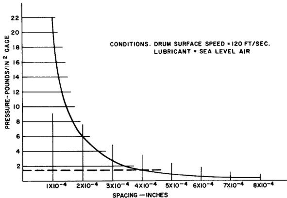
Fig. 13—Mean pressure *vs.* trailing edge to drum space.
