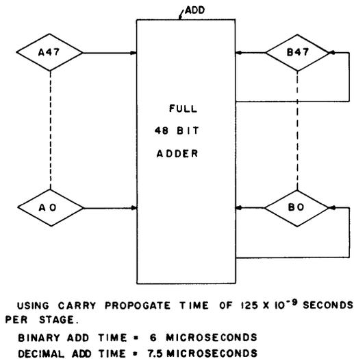
Fig. 4—48-bit parallel accumulator.
