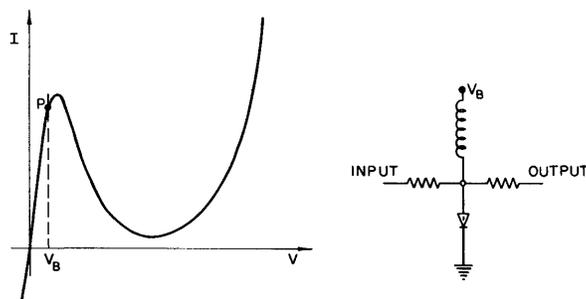
Fig. 18—Tunnel diode monostable logic element.
