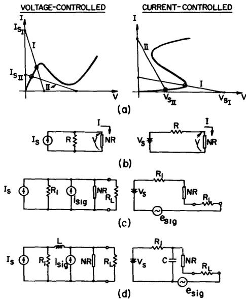
Fig. 1—(a) Load-lines for monostable operation. (b) Equivalent circuits. (c) Load and signal source included. (d) Addition of reactive element.
