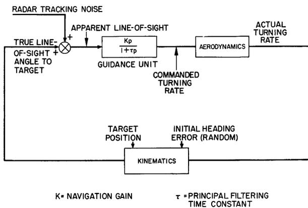
Fig. 1—Radar homing missile navigating in a plane.
