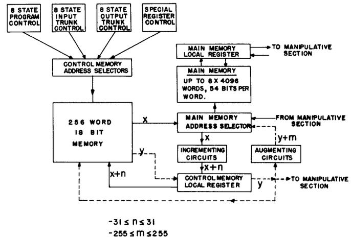
Fig. 1—Control memory in a multiprogram computer.
