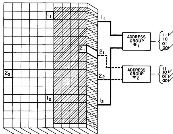
Fig. 1(d)—The system learning the letter I in a third position. The check marks to the right show all possible combinations of these two photocoil pairs for the letter I.
