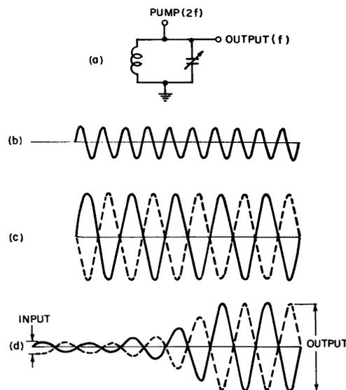
Fig. 1—Principle of parametric phase-locked oscillator.
