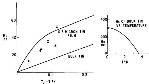
Fig. 1—Critical field of gate film as a function of temperature. Solid line: measured directly. Points: calculated from cryotron characteristics and grid widths, using Eq. 4. Grid widths:  $\blacktriangle$  16 microns (unshielded),  $\square$  65 microns (shielded),  $\circ$  40 microns (shielded).
