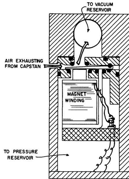
Fig. 7—Schematic of electro-pneumatic valve.
