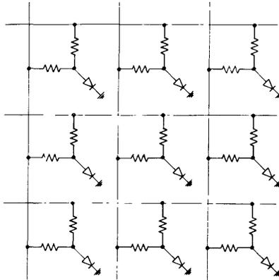
Fig. 20—Tunnel diode memory array.
