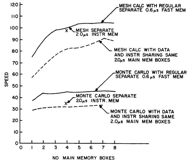
Fig. 14—Computer speed vs. number of main memory boxes: 4 level LA;  $0.6 \mu\text{s}$  I AU time;  $0.64 \mu\text{s}$  AU time.
