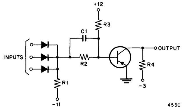
Fig. 2—Basic high-speed circuit.
