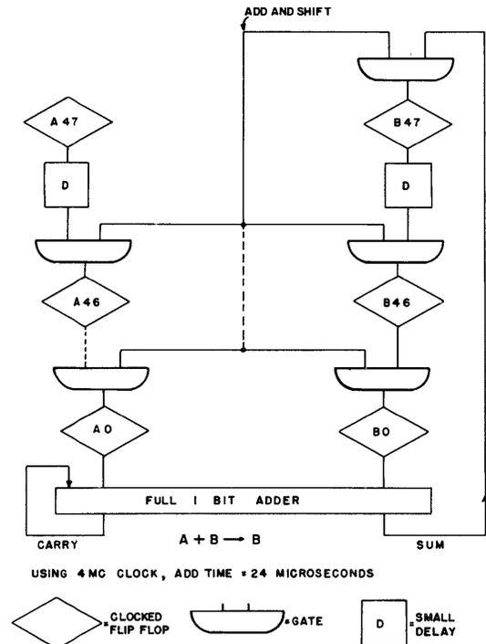
Fig. 2—48-bit serial accumulator.
