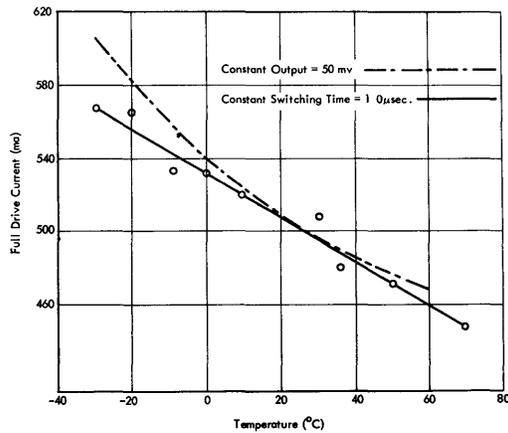
Fig. 2—Core current required vs. temperature.
