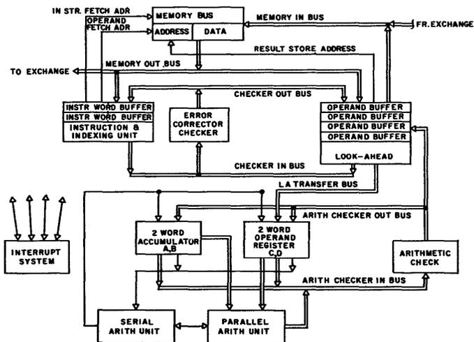
Fig. 5—Stretch Computer — units and dataflow.
