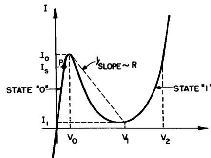
Fig. 15—Tunnel diode characteristics.
