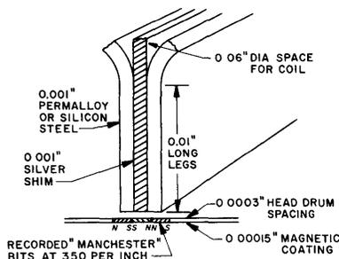
Fig. 7—Practical geometry for recording.
