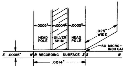
Fig. 6—Ideal geometry for recording 350 bits/inch.
