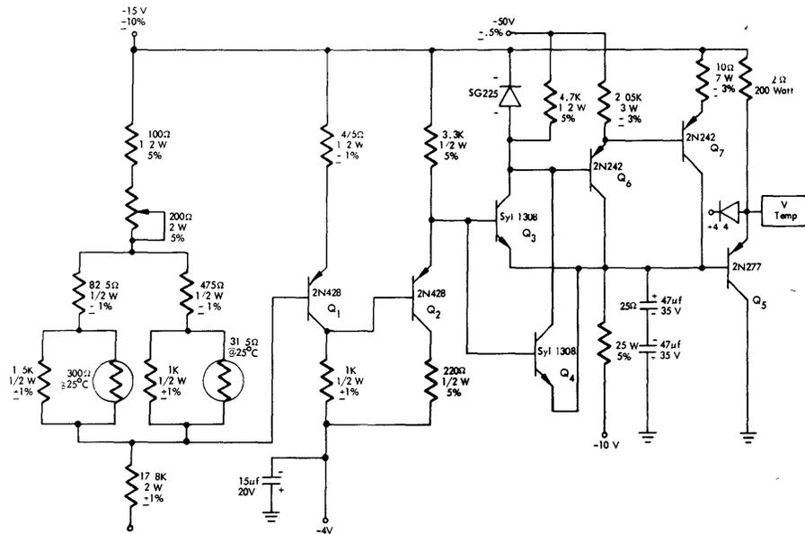
Fig. 7—Temperature controlled voltage source.
