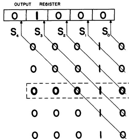
Fig. 7—Functional array for left-shifting a word.
