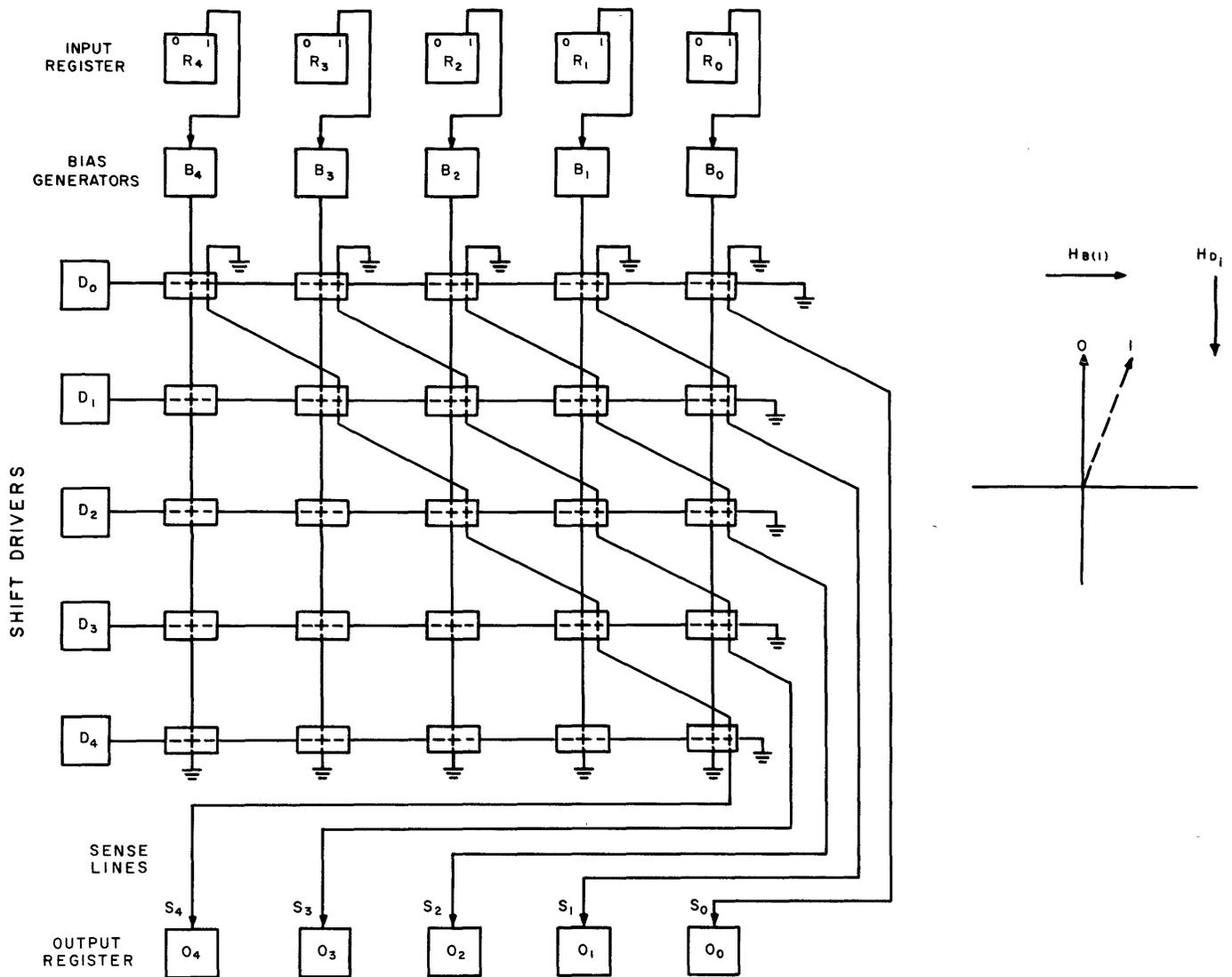
Fig. 8—(a) Film magnetization directions. (b) Network for left-shifting operation.
