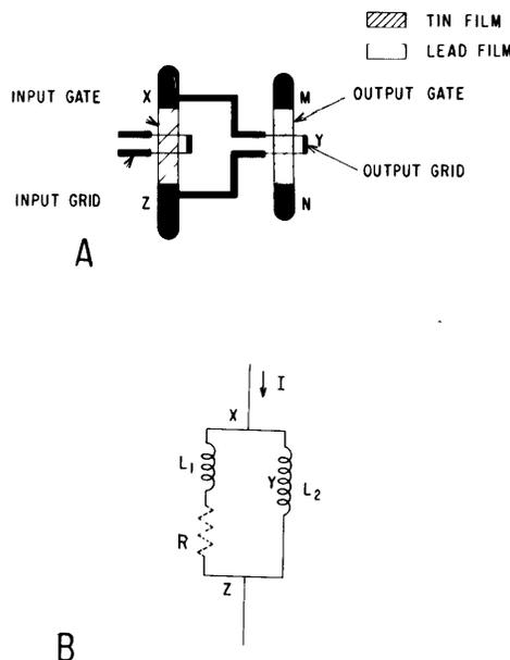
Fig. 5—(a) Cryotron storage cell. (b) Equivalent circuit.
