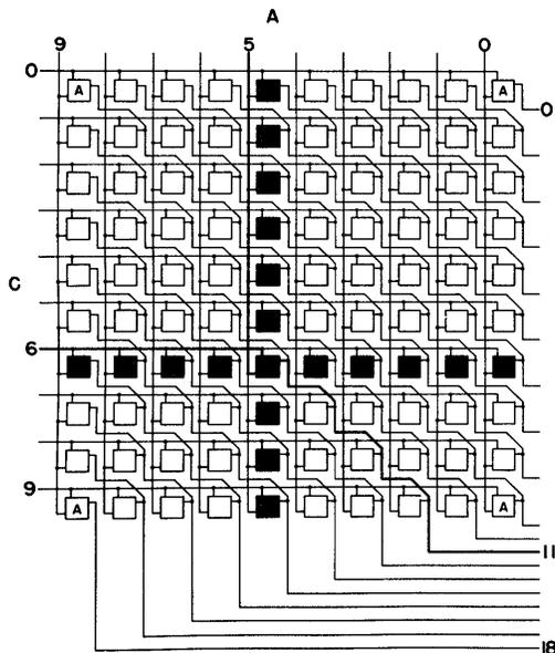
Fig. 6—Matrix utilizing standardized "Boolean" circuits.
