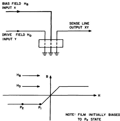
Fig. 2—AND logic (saturable-transformer mode)
