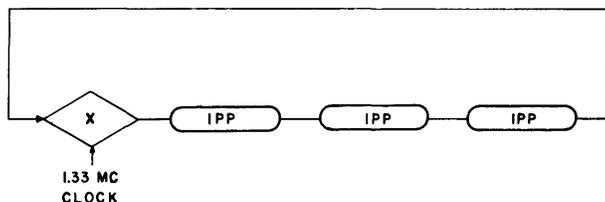
Fig. 7—Use of one flip-flop and 3 pulses of delay to store 4 bits.
