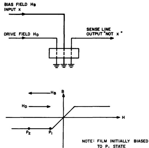
Fig. 3—Inverter logic (saturable-transformer mode).
