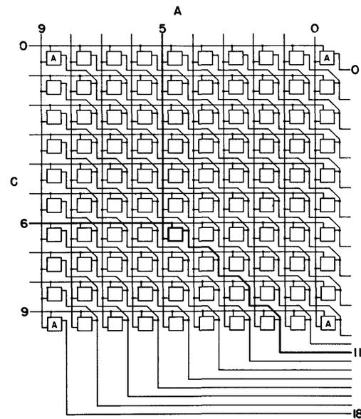
Fig. 5—Matrix utilizing standardized "Boolean" circuits.
