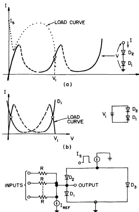
Fig. 5—(a) Characteristic of two tunnel diodes in series and load-curve formed by  $D_3$  and  $I_s$ . (b) Bistable operation. (c) Balanced threshold gate.
