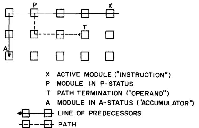
Fig. 3—Modules used in the execution of an instruction.
