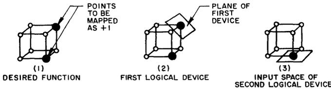
Fig. 5—Synthesis with two logical devices.
