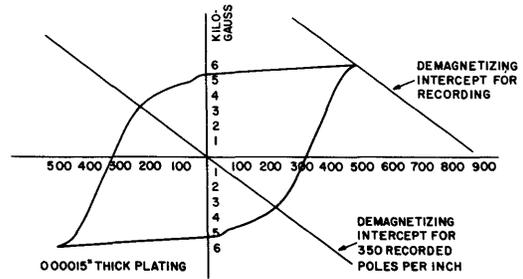
Fig. 4(b)—Actual  $B-H$  loop for heat treated electroless nickel-cobalt.
