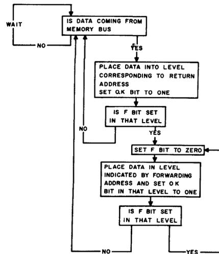
Fig. 9—Procedure for placing data into virtual memory.
