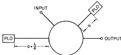
Fig. 11—Circuit for separating input and output of PLO's.
