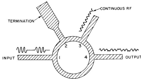
Fig. 10—Hybrid circuit for translating amplitude-to-phase scripts.
