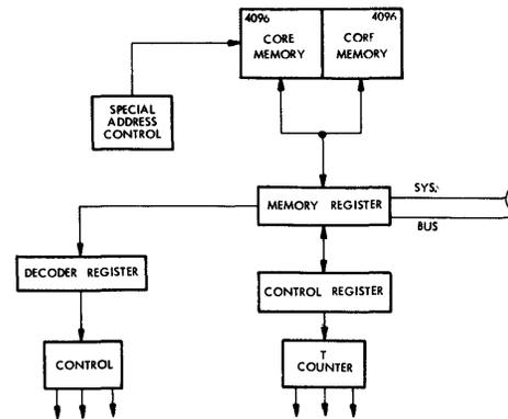
Fig. 3—MOBIDIC B processor.
