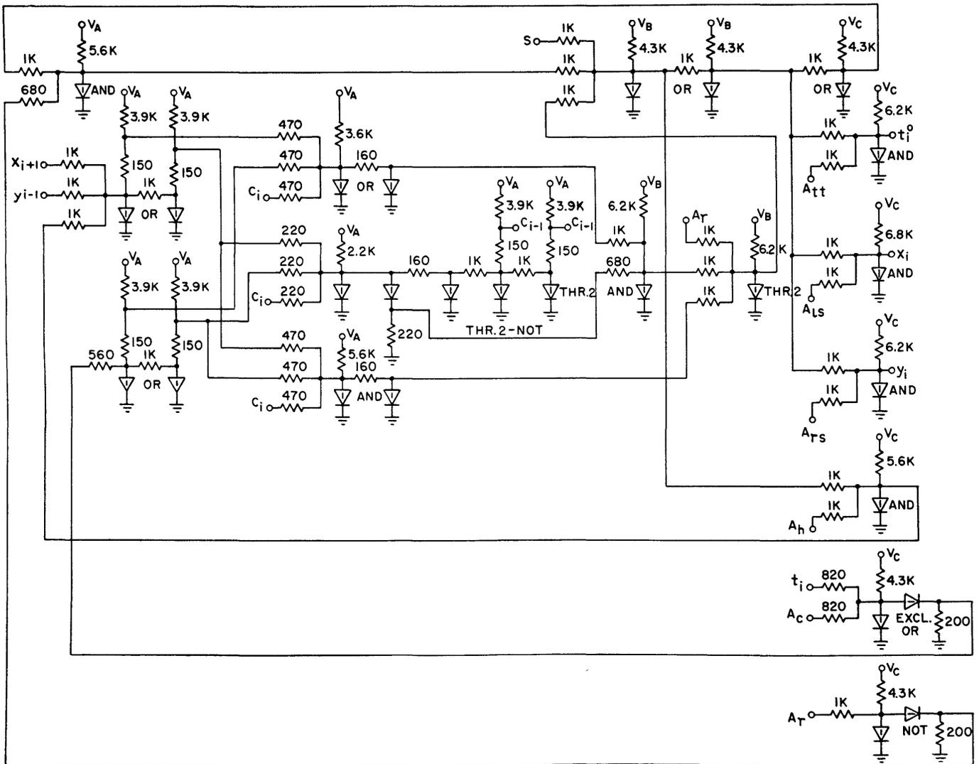
Fig. 12—Schematic diagram of experimental circuit.
