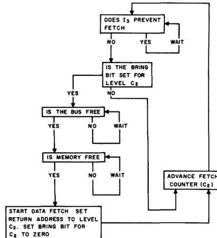
Fig. 7—Data fetch procedure.
