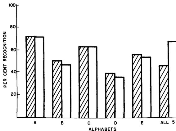
Fig. 6—Comparisons of the percent recognized for hand-block print read with different *n*-tuplings: *n* = 1 (hatched bars) and *n* = 2 (solid bars). Note that when all five alphabets are learned together, the percent for *n*=2 improves. In other words, for *n* = 2, the ability to read improves with additional learning in the memory matrix.
