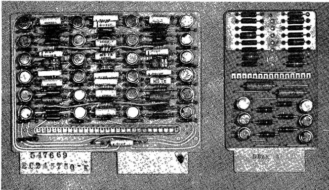
Fig. 14—The circuit package.
