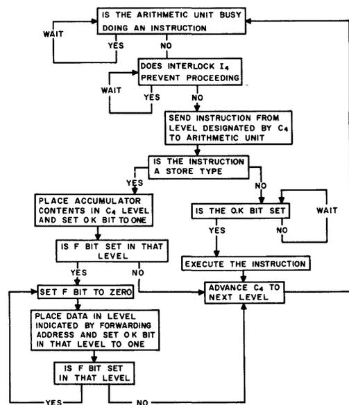
Fig. 10—Procedure for removing instructions from virtual memory.
