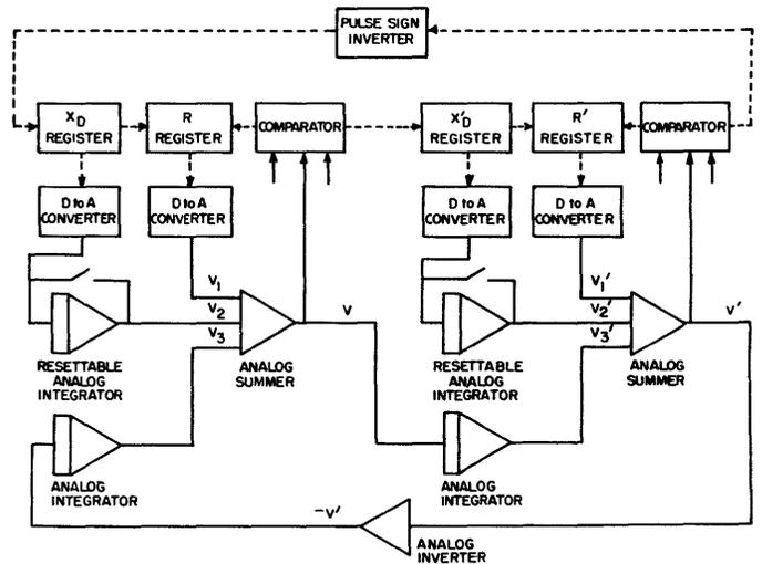
Fig. 6—Two integrators interconnected to solve:  $\dot{x} = x$ ,  $\dot{x} = -x'$ .
