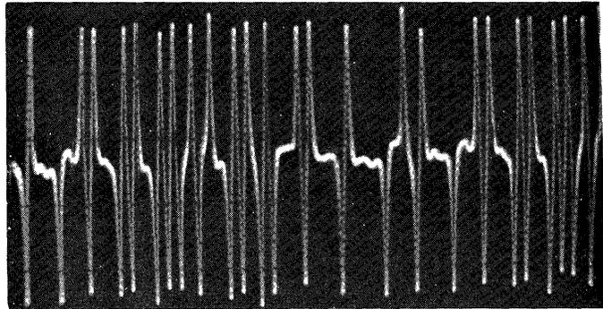
Fig. 10—Normal preamplifier output of read system.
