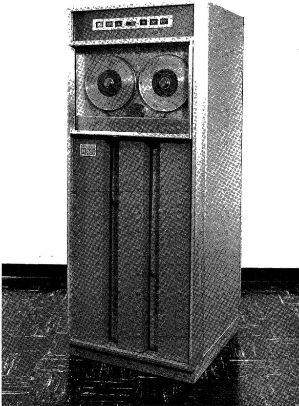
Fig. 1—Type 804 magnetic tape mechanisms.
