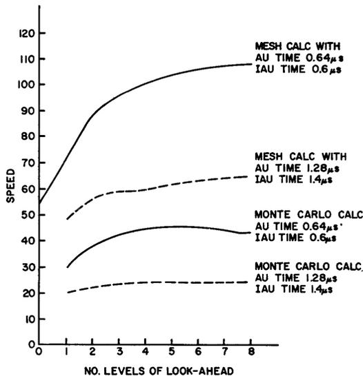
Fig. 13—Computer speed vs. no. of levels of look-ahead registers; 4 main mems.  $2.0 \mu\text{s}$ ; 2 fast mems.  $0.6 \mu\text{s}$  for two sets of arith. speeds.
