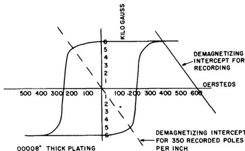
Fig. 4(a)—Actual  $B-H$  loop for electroplated nickel-cobalt.
