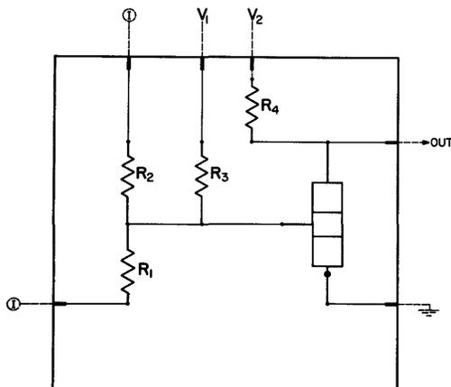
Fig. 4—Standard "and-inverter" circuit (TRL).
