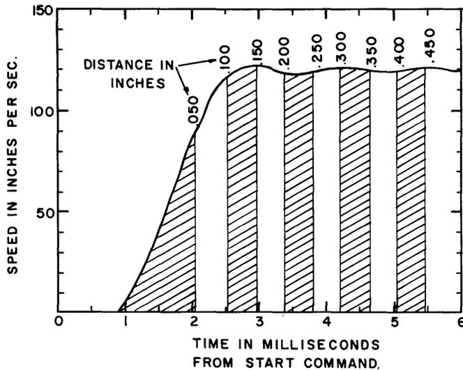
Fig. 8—Typical curve of velocity and distance vs. time during tape acceleration.
