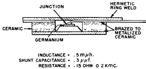
Fig. 13—Cross-section of variable capacity diode.
