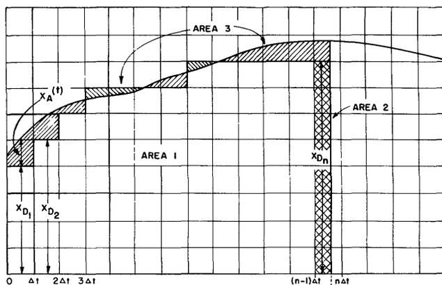
Fig. 1—Diagram of integration method.
