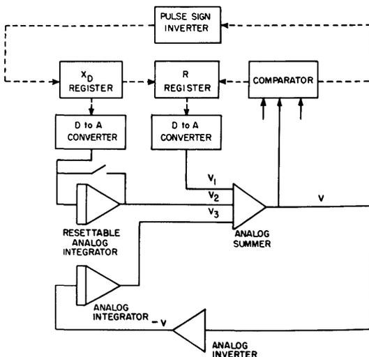
Fig. 4—Integrator used to solve:  $\dot{x} = -x$ .
