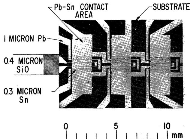
Fig. 7—Portion of experimental shift register. Note the insulator film separating the grids from the underlying gate films.
