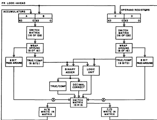
Fig. 7—Serial arithmetic unit.
