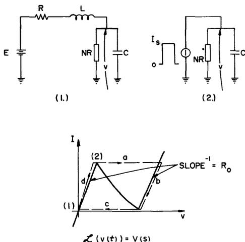
Fig. 16—Comparison of monostable and bistable-with-reset modes. Assumed path of operation.
