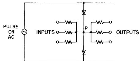
Fig. 17—Tunnel diode bistable logic element (symmetric type).
