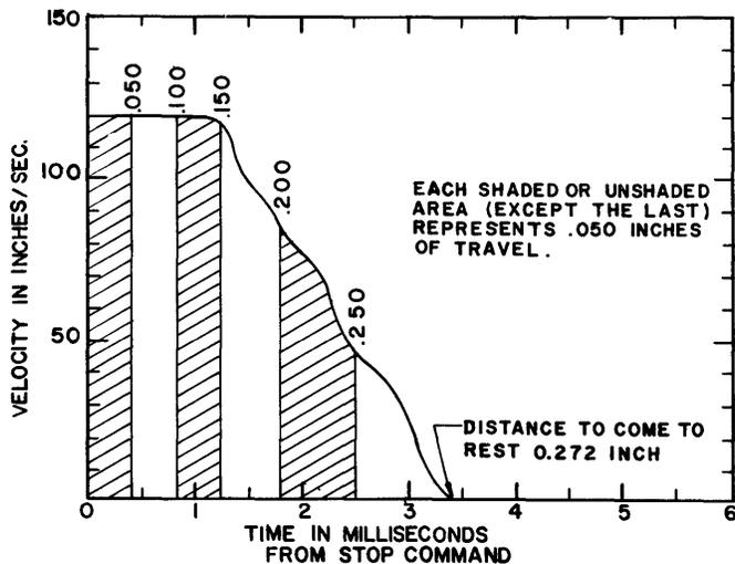
Fig. 9—Typical curve of velocity and distance vs. time during tape deceleration.
