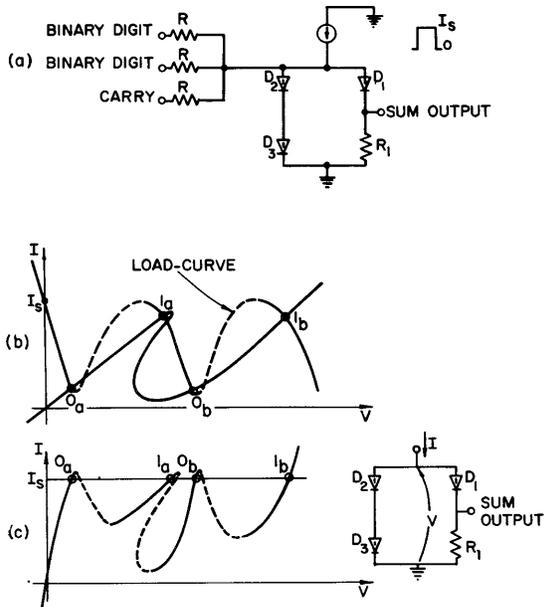
Fig. 7—(a) SUM output circuit for full adder. (b) Determination of operating points. (c) Composite characteristic.
