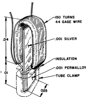
Fig. 9—Essential details of the magnetic head.
