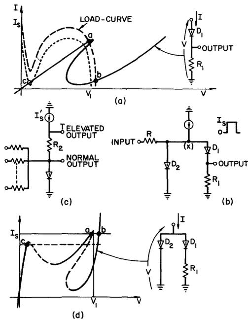
Fig. 6—(a) Characteristic of tunnel diode and resistor in series and load-curves formed by  $D_2$  and  $I_s$ . (b) Inverter circuit. (c) Provision for obtaining elevated output. (d) Composite characteristic of  $D_1$ ,  $D_2$  and  $R_1$ .
