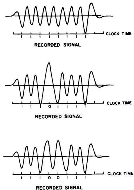
Fig. 3—Read signals with clock times indicated.
