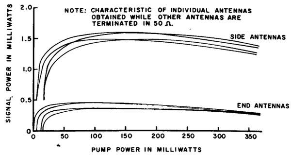
Fig. 8—Characteristic of four antenna PLO.
