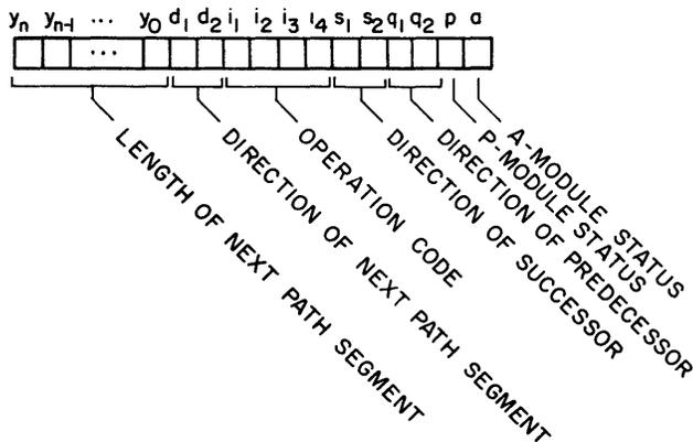
Fig. 4—Control of module by storage register.
