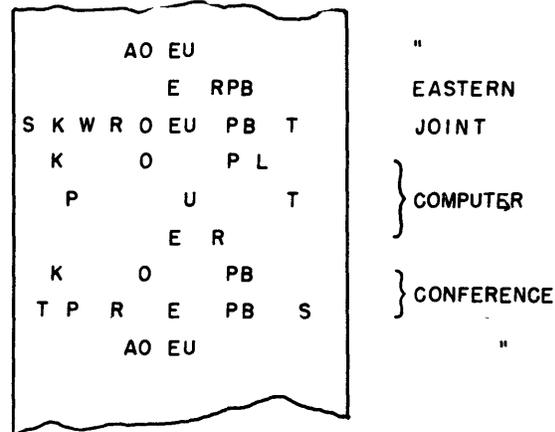
Fig. 1—Sample stenotype tape.
