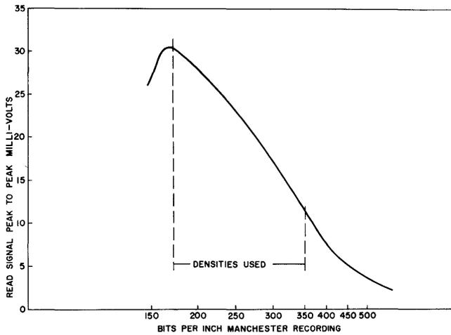
Fig. 8—Typical response for magnetic read-record head.
