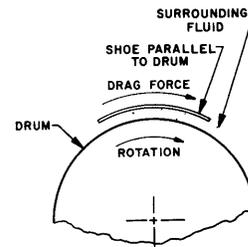
Fig. 11—Schematic view of drum with shoe in parallel position.
