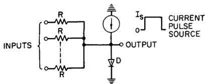
Fig. 4—Single-ended threshold gate.
