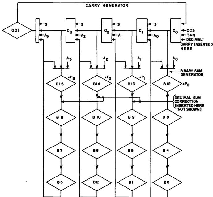
Fig. 6—Logical organization for major character 1 of parallel serial parallel accumulator.
