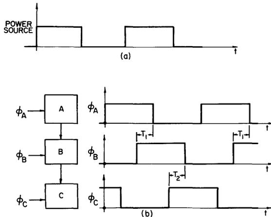
Fig. 2—(a) Power supply waveform.
