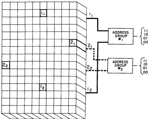
Fig. 1(a)—The photomosaic and two of the randomly chosen photocoil pairs. The four digital groups to the right are the four possible states of each photocoil pair.
