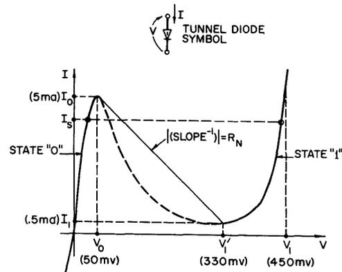
Fig. 3—Tunnel diode static characteristic. (Number indicated for typical Germanium unit.)
