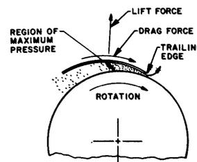
Fig. 12—Schematic view of drum with shoe at angle to develop wedge of lubricant.
