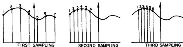
Fig. 7—Successive sampling of the performance curve.
