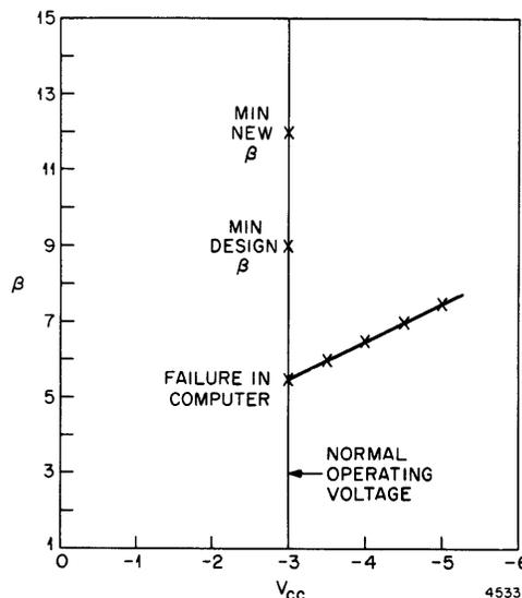
Fig. 11—Circuit failure as a function of  $V_{cc}$  and  $\beta$ .
