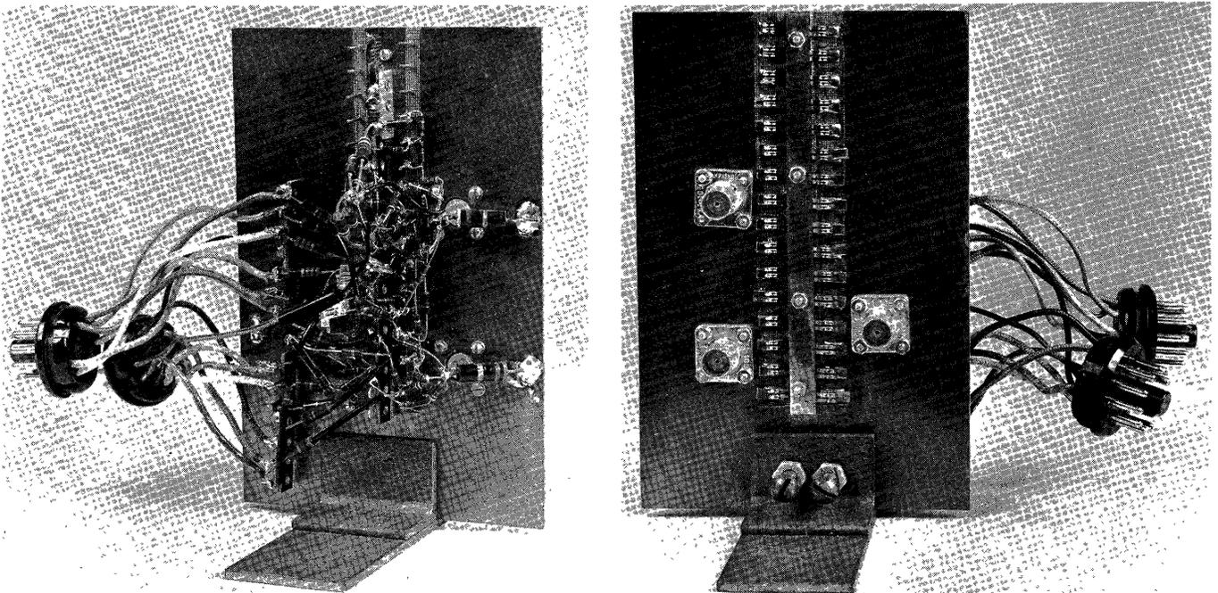
Fig. 13—Front and rear views of experimental cell. (Tunnel diodes are mounted under finger contacts.)
