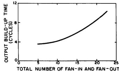
Fig. 9—Number of cycles of build-up as a function of logic gain.
