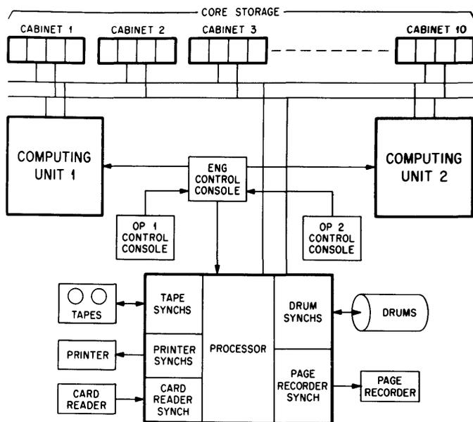
Fig. 2—Block diagram of a LARC system.
