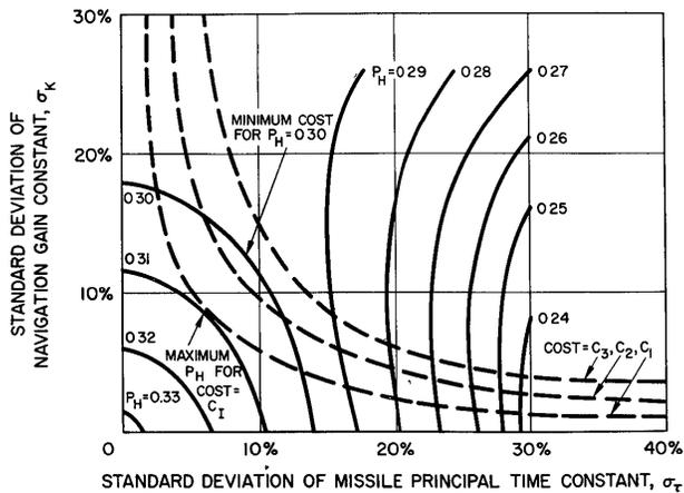
Fig. 5—Optimization of tolerances for minimum cost or maximum performance.
