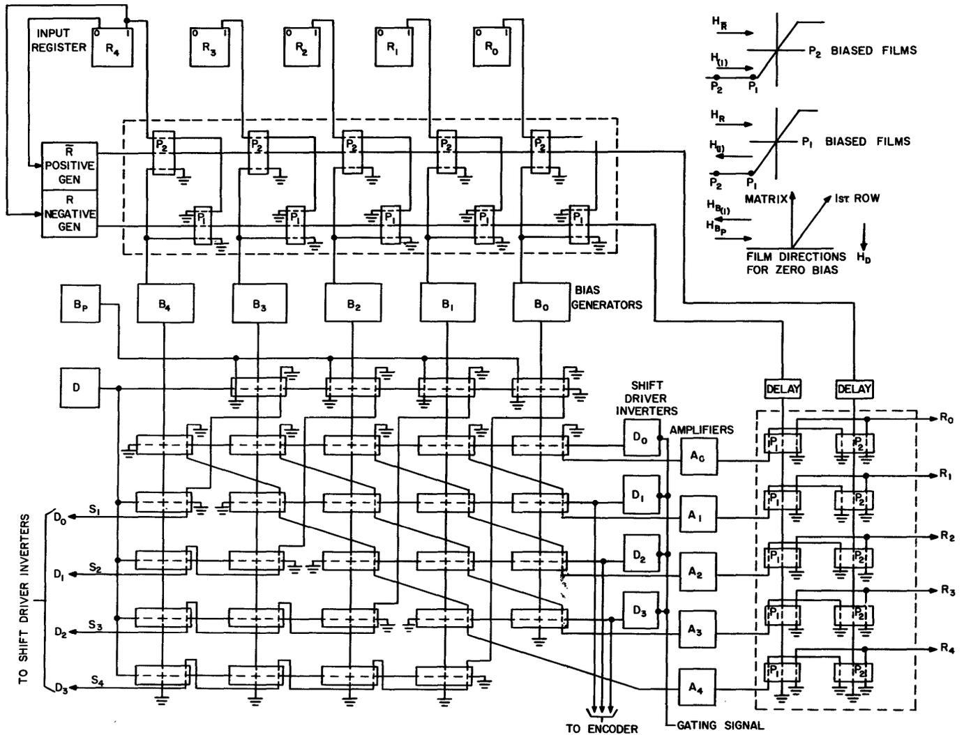
Fig. 10—Scale-factor network.
