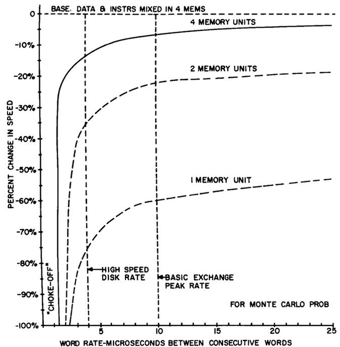
Fig. 17—Internal computing speed. Percentage reduction in speed caused by input-output devices referencing memory at different rates while the calculation is proceeding.
