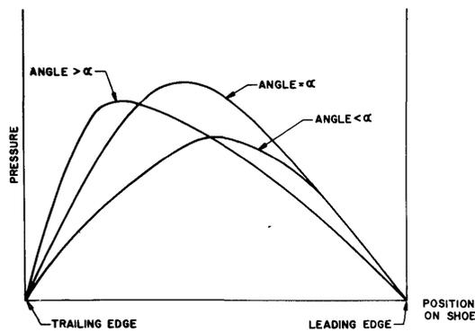
Fig. 14—Typical pressure distribution vs. change in attack angle  $\alpha$ .
