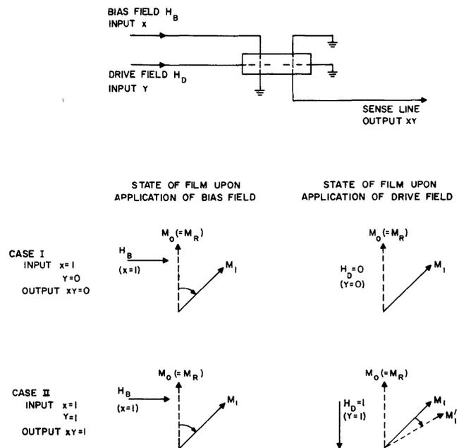
Fig. 1—AND logic (reversible-rotation mode).
