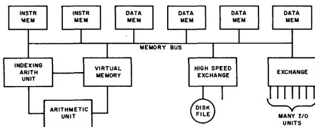
Fig. 1—Schematic of Stretch computer.
