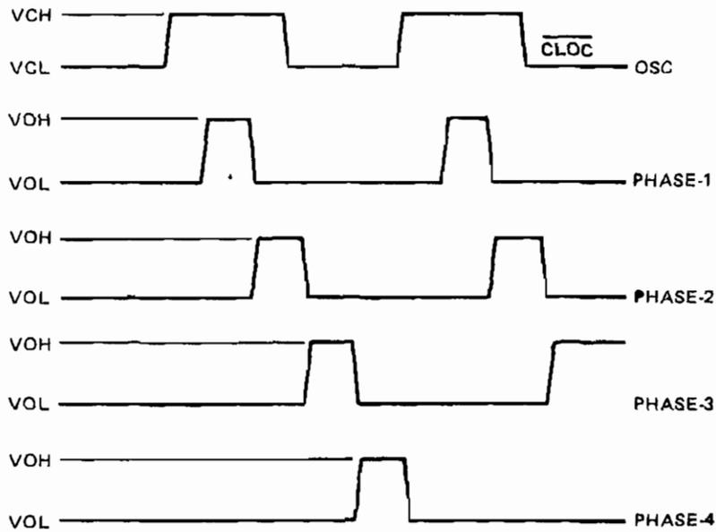
Figure 4-55. Four-phase Clock Logic and Timing
