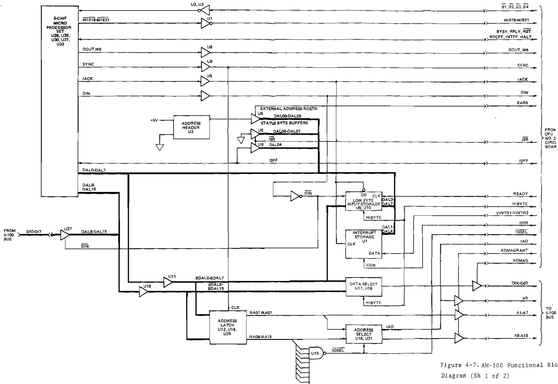
Figure 4-7. AM-100 Functional Block Diagram (Sh 1 of 2)
