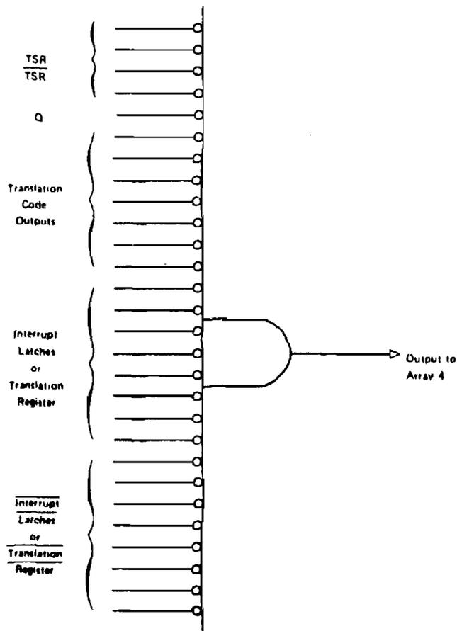
Figure 4-35. Typical Gate of Array No. 3
