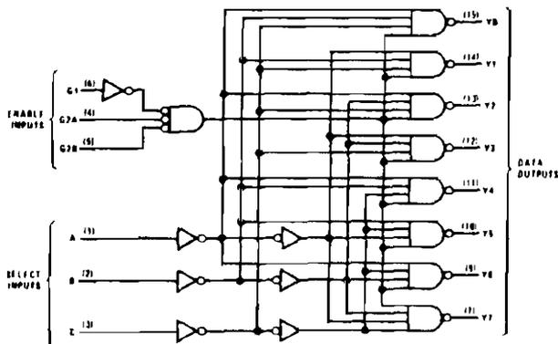
Figure 4-67. Decoder Connections
