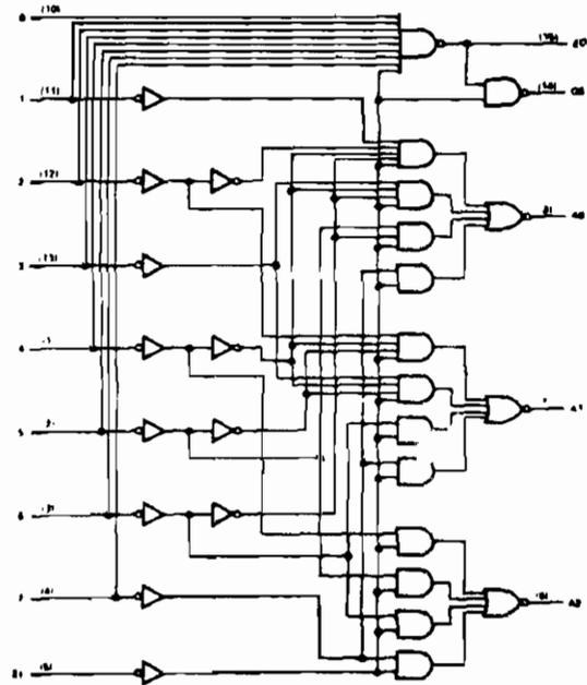
Figure 4-60. Eight-Line to Three-Line Encoder Connections
