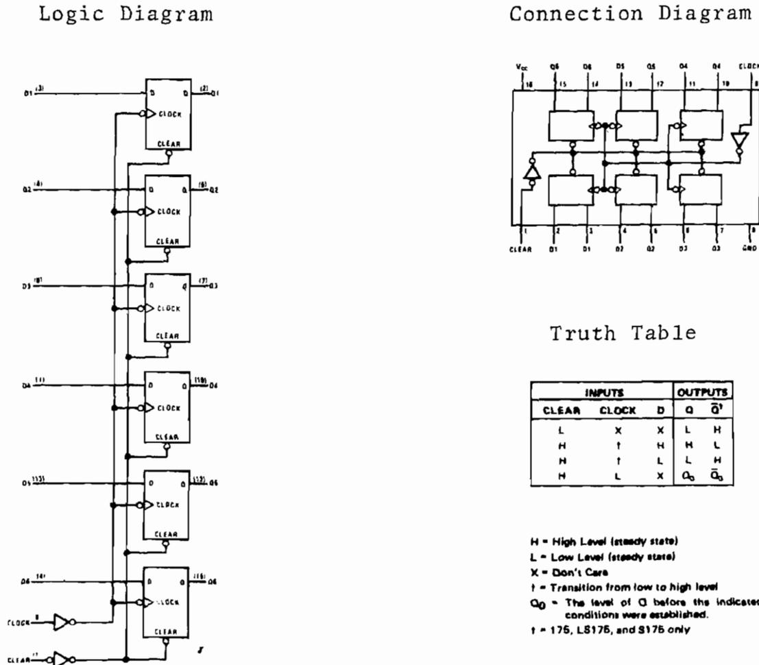
Figure 4-68. D Flip-Flop Connections
