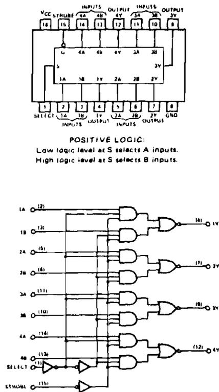
Figure 4-61. Data Selector/Multiplexer Connections
