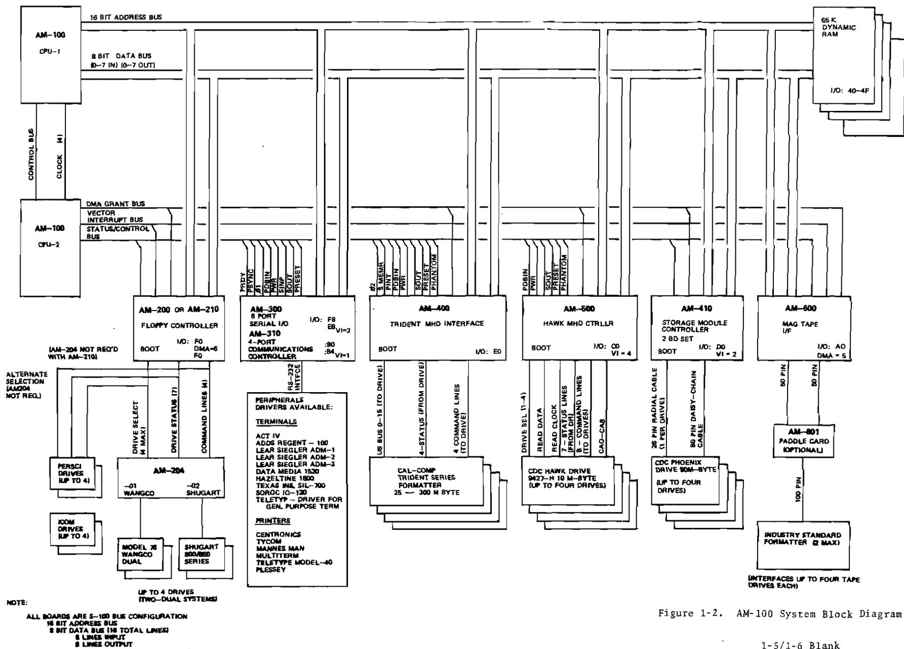
Figure 1-2. AM-100 System Block Diagram
