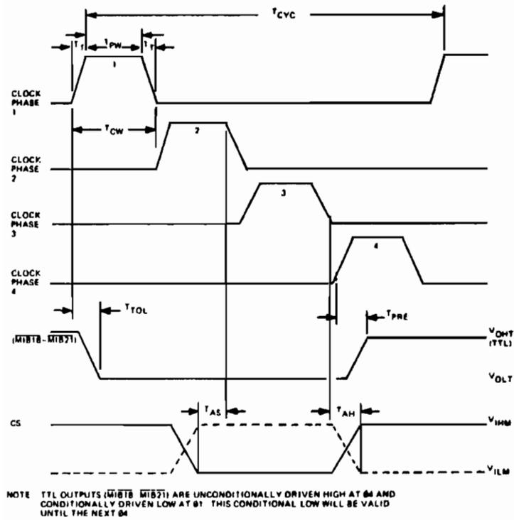
Figure 4-42. TTL Output Timing CP1631B
