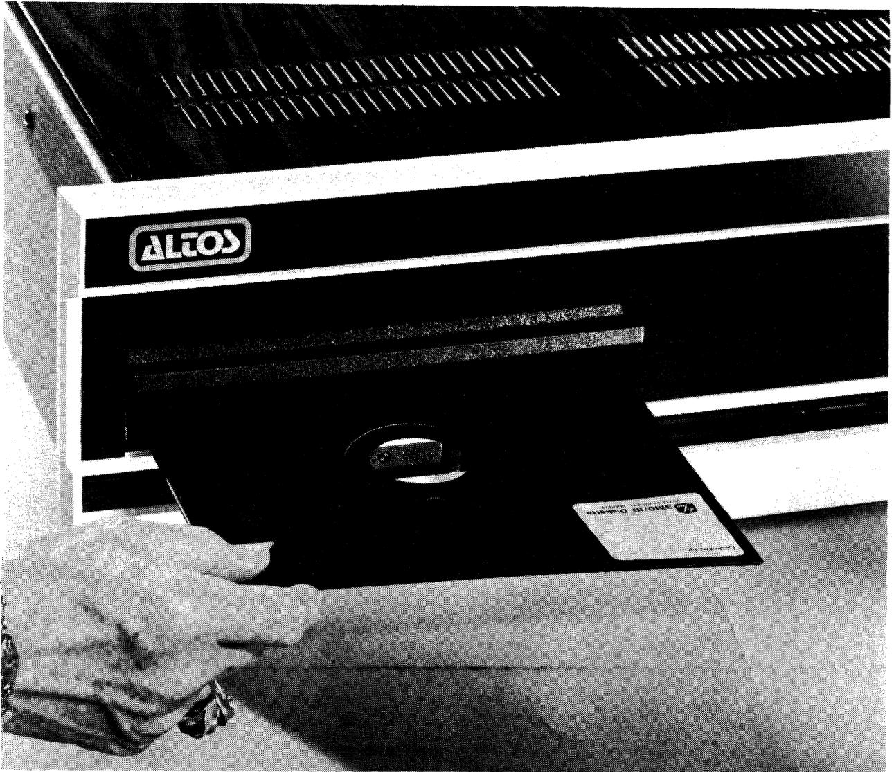
Figure 1-4. Disk Insertion on the ACS8000-10 Computer
