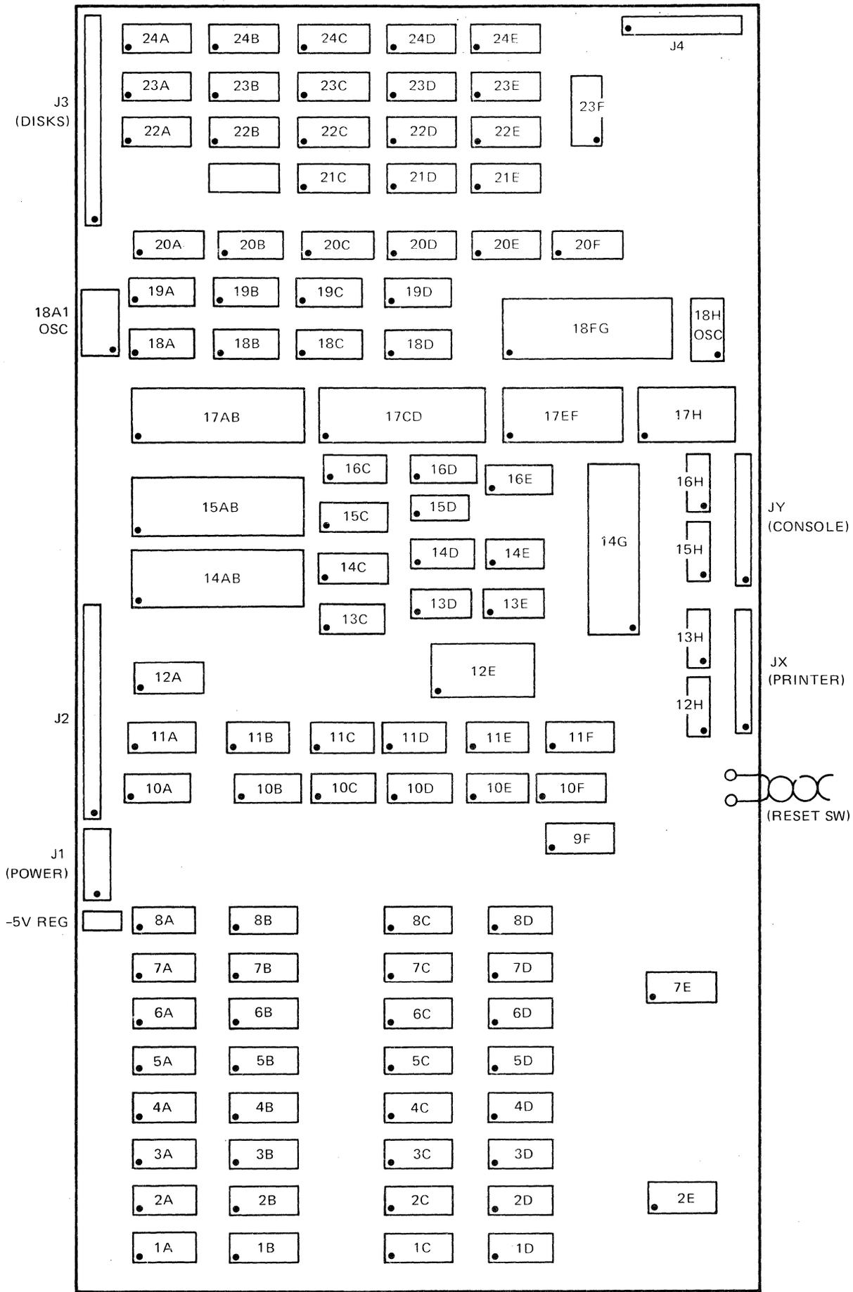
FIGURE 7 OVERALL INTEGRATED CIRCUIT LOCATION DIAGRAM - DOUBLE DENSITY
