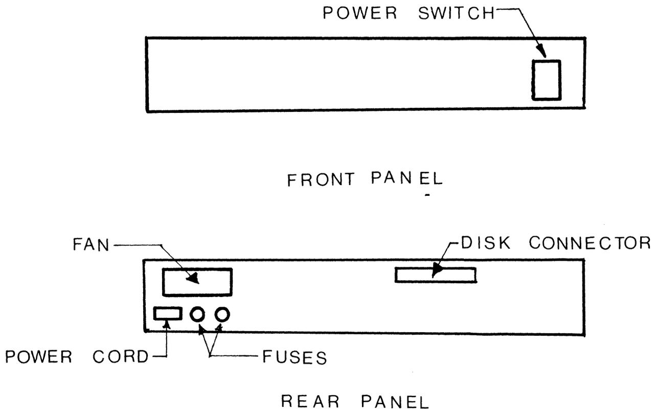
FIGURE 10; WINCHESTER DISK CONNECTION
