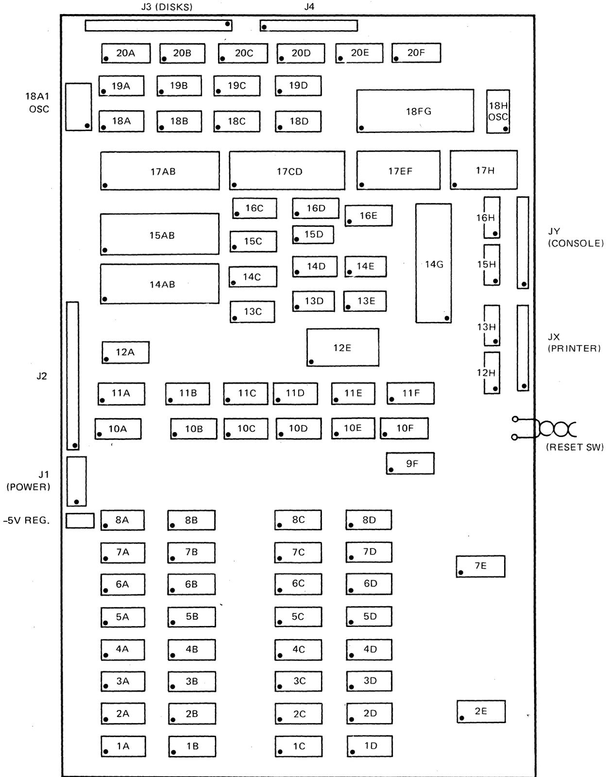
FIGURE 7 OVERALL INTEGRATED CIRCUIT LOCATION DIAGRAM - SINGLE DENSITY
