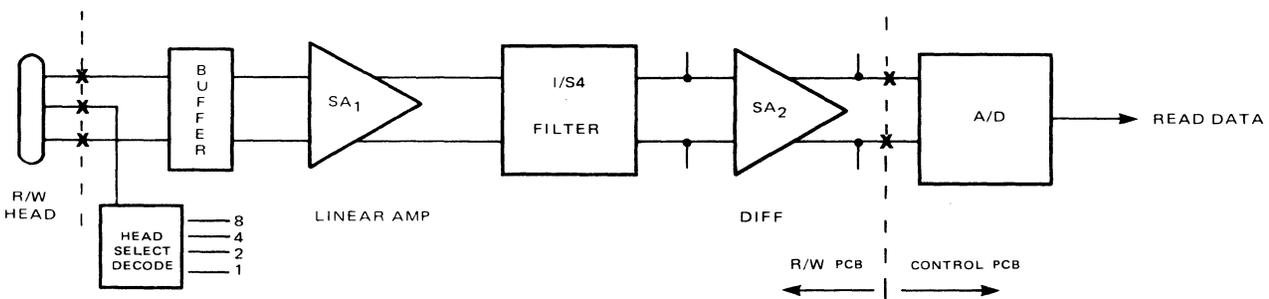
Figure 2. Block Diagram
