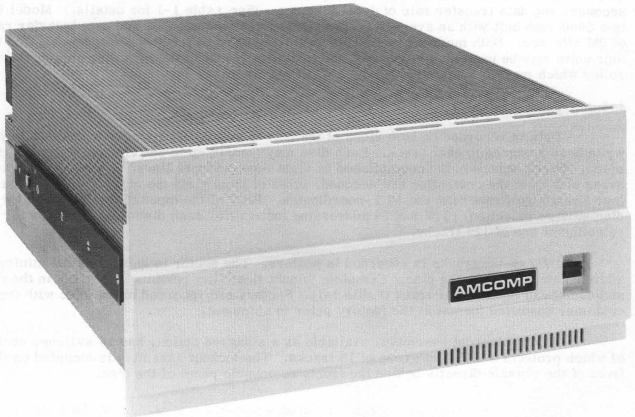
Figure 1-1. 8500 Series Disc Memory Unit
