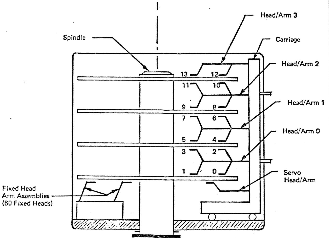
Fig 1a - Head/Disk Assembly (HDA)
