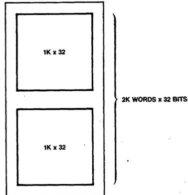
Note: Other configurations (wider and deeper) can be supported by additional boards and combinations.
