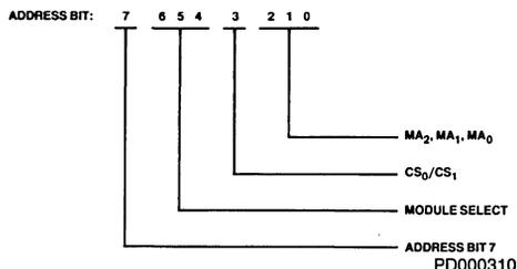
CS<sub>0</sub>/CS<sub>1</sub>, MA<sub>0</sub>, MA<sub>1</sub>, MA<sub>2</sub> are sent to the SBX module and used as needed.
