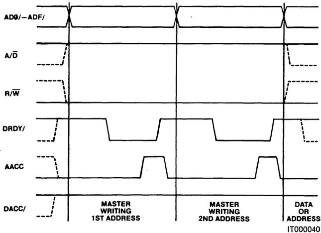
Figure 6. MULTICHANNEL™ Bus Data Transfer Sequence
