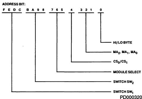
Address bit 0 is used to choose between the high and low byte of a 16-bit module. A jumper is provided to invert bit zero to provide for the requirements of the microprocessor.
