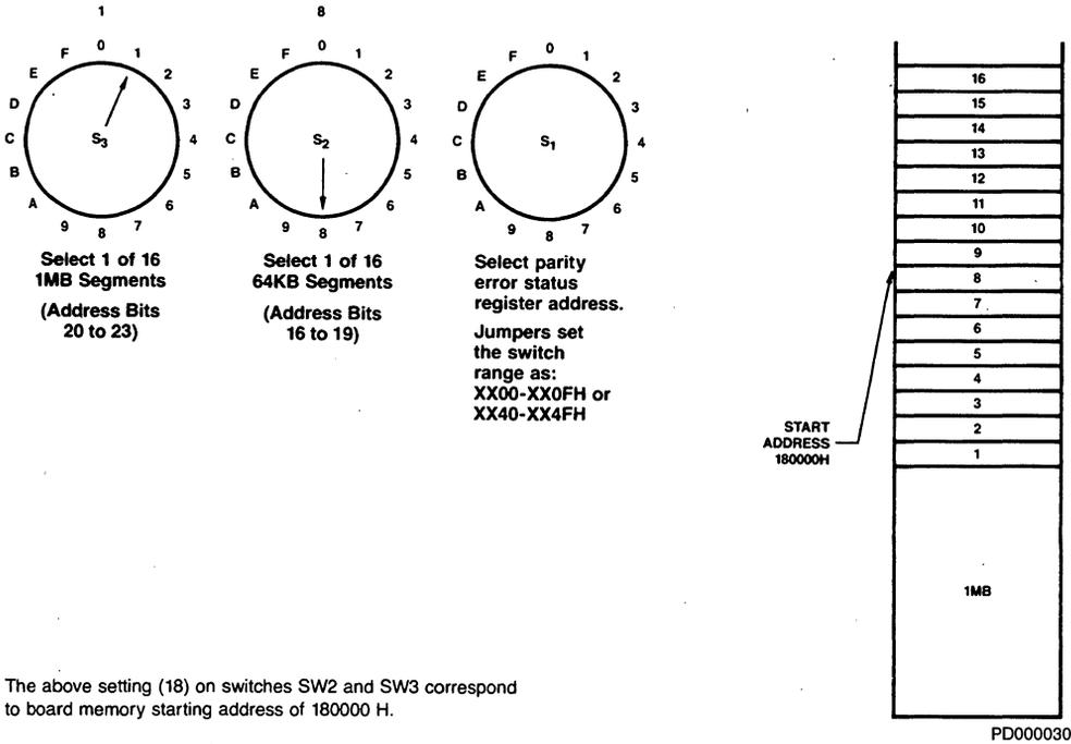
The above setting (18) on switches SW2 and SW3 correspond to board memory starting address of 180000 H.
