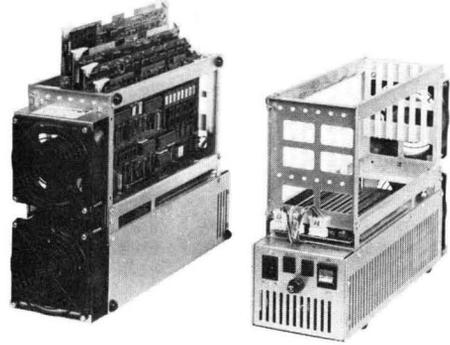
supply. It furnishes  $\pm 5$  and  $\pm 12$ VDC (regulated) MULTIBUS voltage requirements. The power supply module, MULTIBUS backplane, input panel, cooling fans, and metal frame are integrated into a compact trim design for use in industrial chassis and for benchtop use (see Figure 2).
