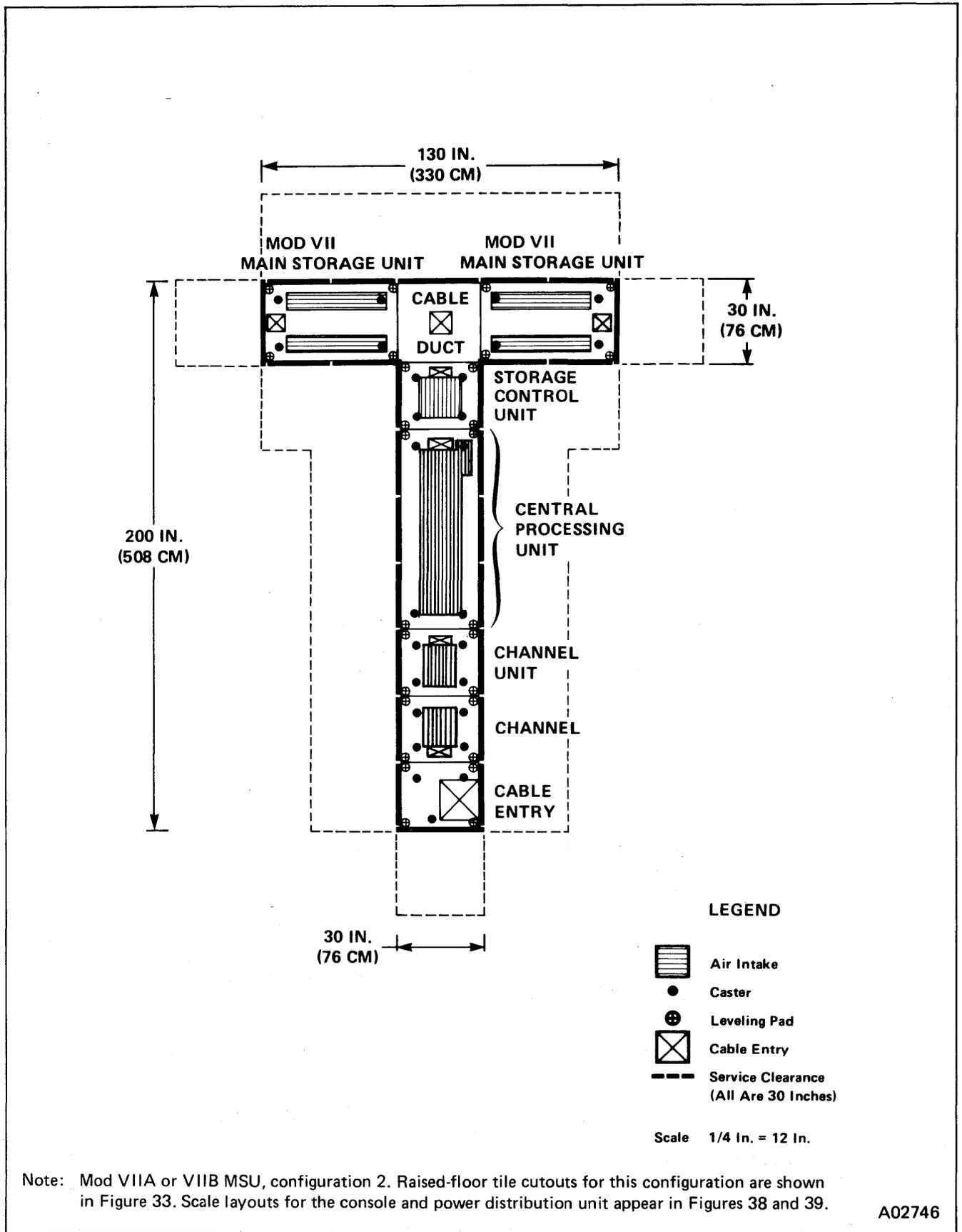
Note: Mod VIIA or VIIB MSU, configuration 2. Raised-floor tile cutouts for this configuration are shown in Figure 33. Scale layouts for the console and power distribution unit appear in Figures 38 and 39.
