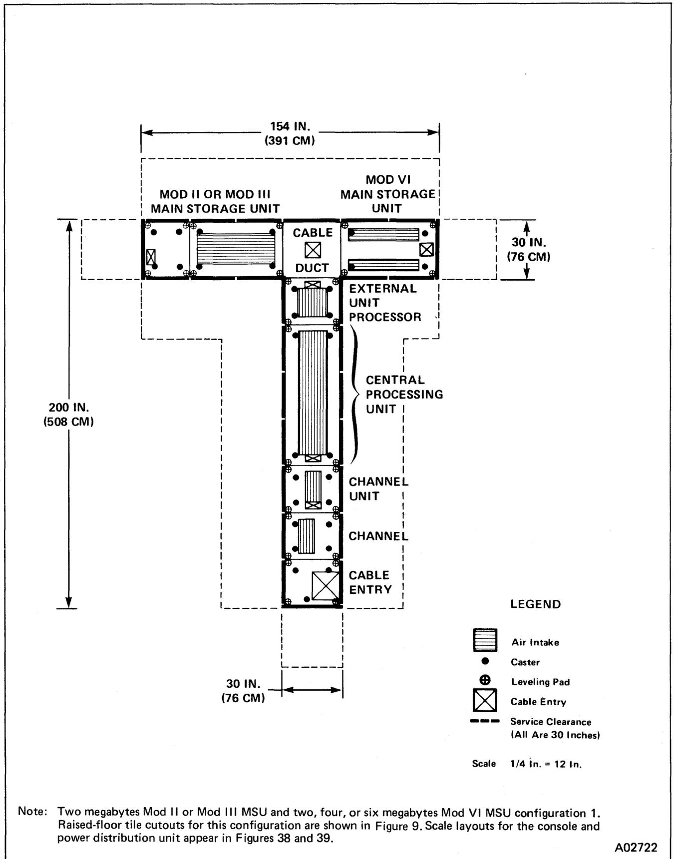
Figure 8. V/5 and V/6 Scale Layout Showing "Long-Left-T," Configuration 1
