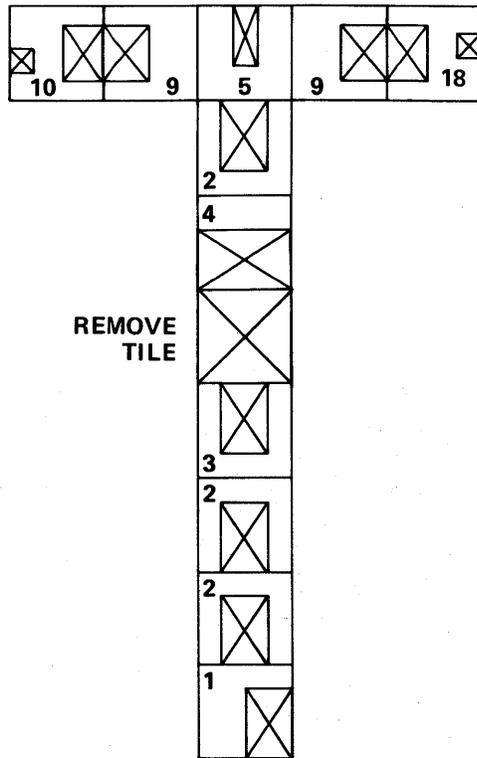
THE CONSOLE REQUIRES A SPECIAL CABLE ENTRY TILE CUTOUT, THE LOCATION OF WHICH DEPENDS ON CONSOLE POSITIONING. THE CUT-OUT DIMENSIONS MUST BE MINIMIZED TO REDUCE AIR LOSS.
