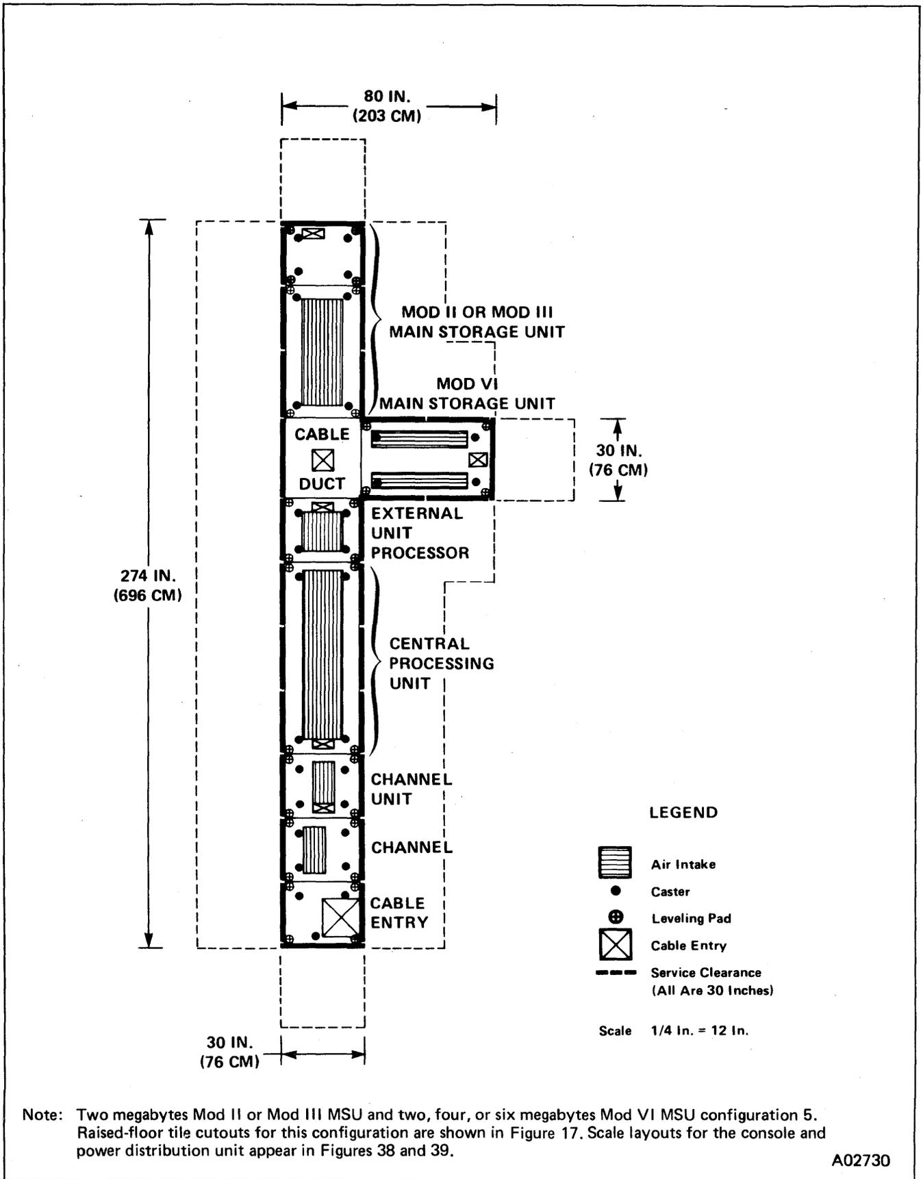
Figure 16. V/5 and V/6 Scale Layout Showing "Short-Right-L", Configuration 5
