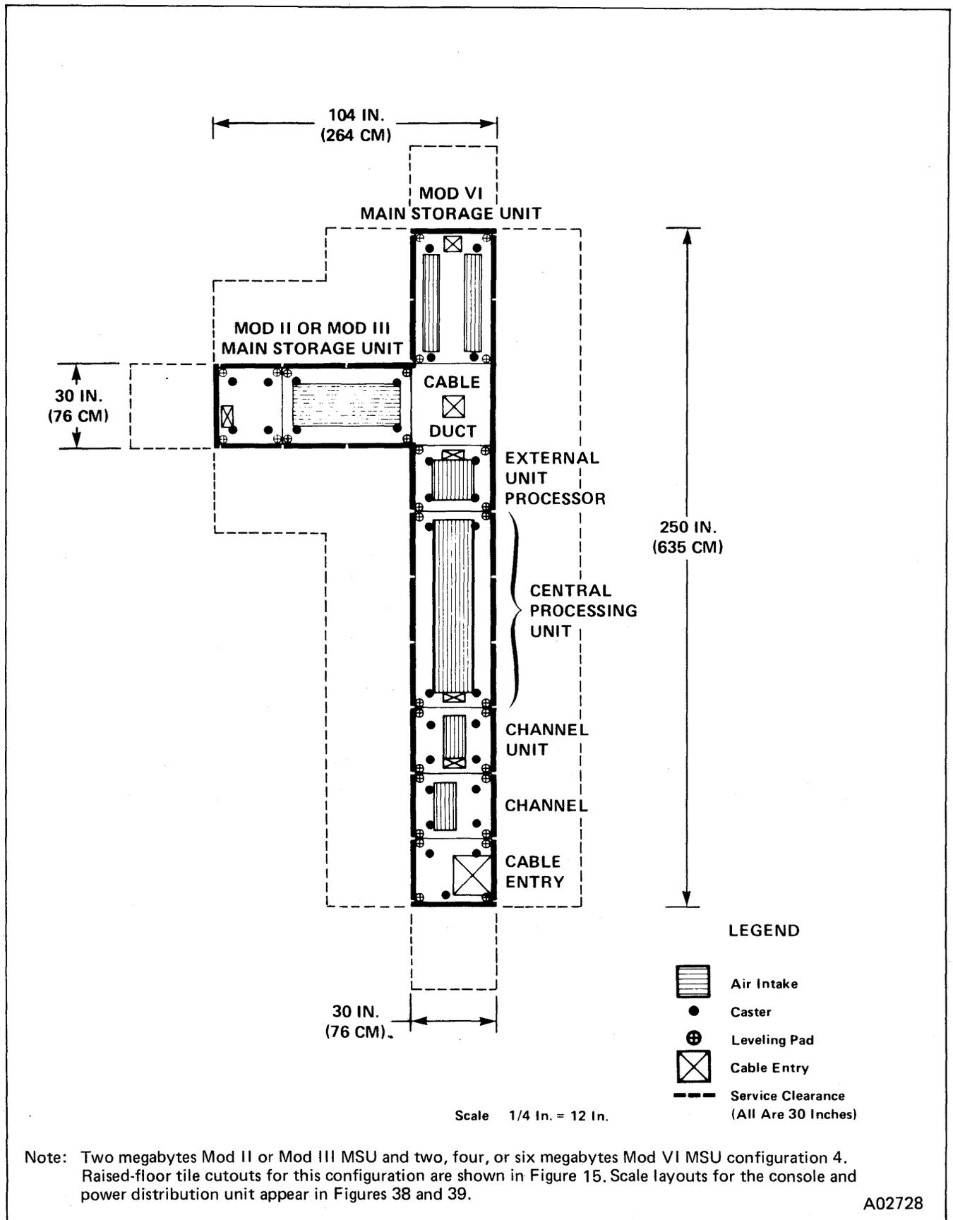
Figure 14. V/5 and V/6 Scale Layout Showing "Long-Left-L", Configuration 4
