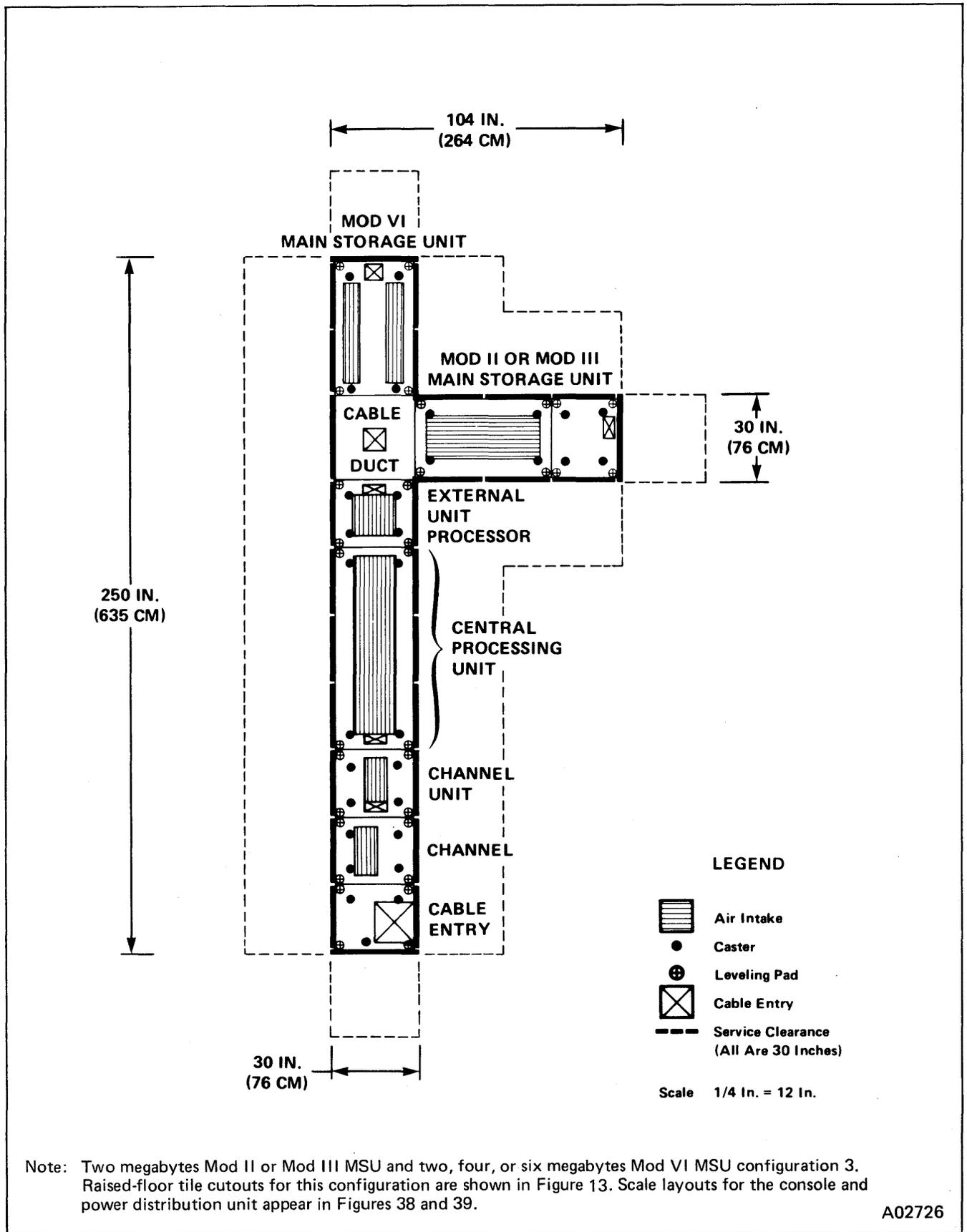
Figure 12. V/5 and V/6 Scale Layout Showing "Long-Right-L", Configuration 3
