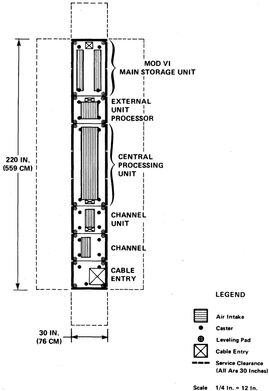
Note: Two, four, six, or eight megabytes Mod VI MSU only. Raised-floor tile cutouts for this configuration are shown in Figure 27. Scale layouts for the console and power distribution unit appear in Figures 38 and 39.
