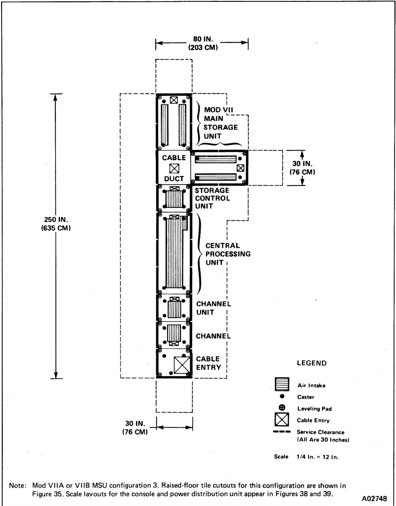
Figure 34. V/7 and V/8 Scale Layout Showing "Inverted-L", Configuration 3
