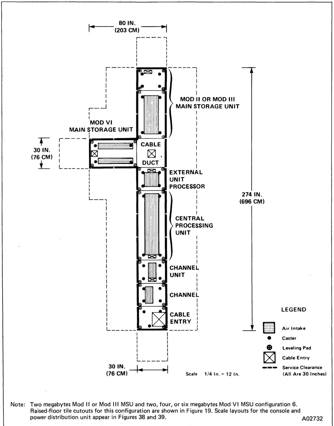
Figure 18. V/5 and V/6 Scale Layout Showing "Short-Left-L", Configuration 6
