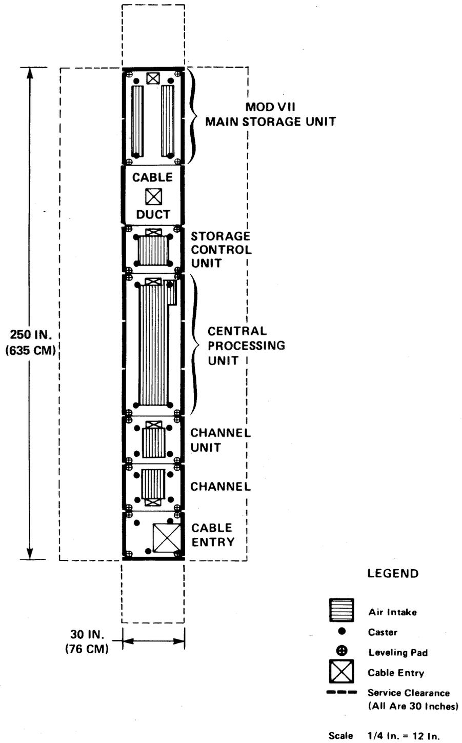
Note: Mod VIIA or VIIB MSU. Raised-floor tile cutouts for this configuration are shown in Figure 31. Scale layouts for the console and power distribution unit appear in Figures 38 and 39.
