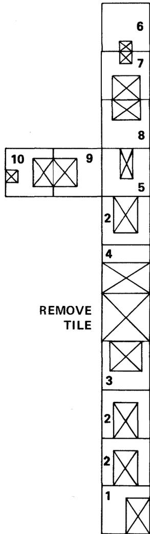
THE CONSOLE REQUIRES A SPECIAL CABLE ENTRY TILE CUTOUT, THE LOCATION OF WHICH DEPENDS ON CONSOLE POSITIONING. THE CUT-OUT DIMENSIONS MUST BE MINIMIZED TO REDUCE AIR LOSS.
