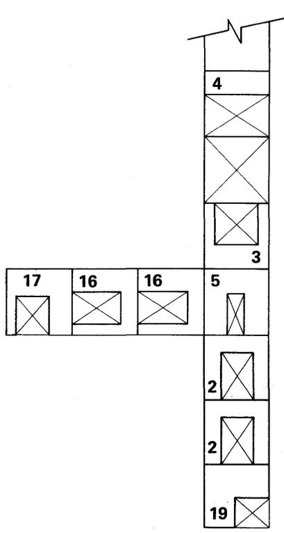
THE CONSOLE REQUIRES A SPECIAL CABLE ENTRY TILE CUTOUT, THE LOCATION OF WHICH DEPENDS ON CONSOLE POSITIONING. THE CUT-OUT DIMENSIONS MUST BE MINIMIZED TO REDUCE AIR LOSS.
