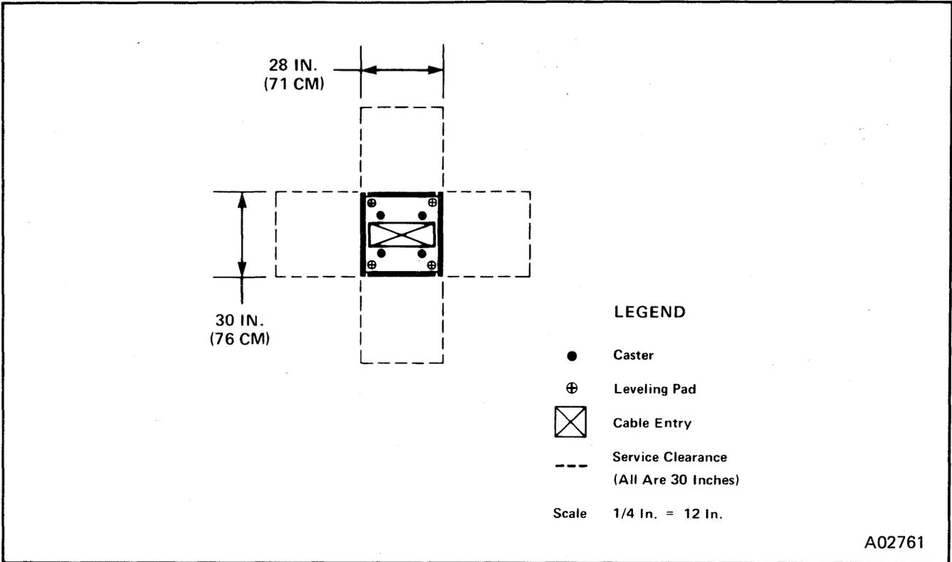
Figure 47. V/7, V/8 HMI (Option) Scale Layout
