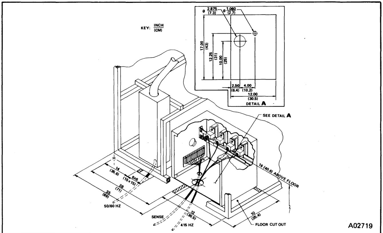
Figure 5. PDU Mod I, Interconnection Wiring Block
