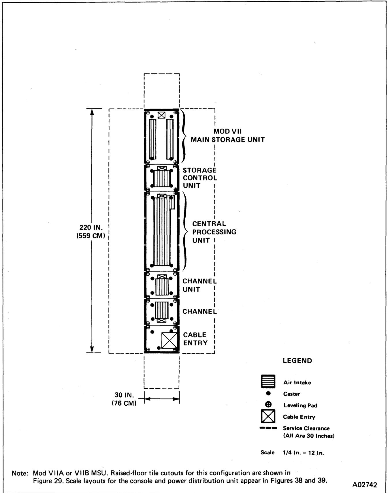
Figure 28. V/7 and V/8 Scale Layout Showing "Basic-I", Configuration 1 (Without Cable Duct)
