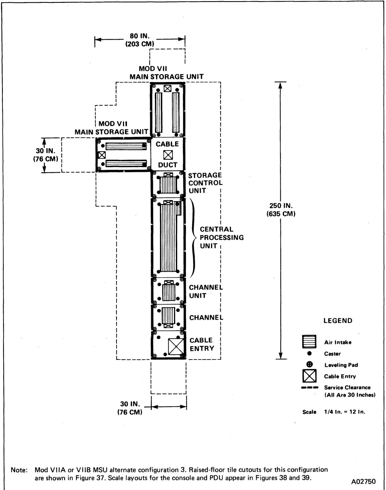
Figure 36. V/7 and V/8 Scale Layout Showing "Standard L", Alternate Configuration 3
