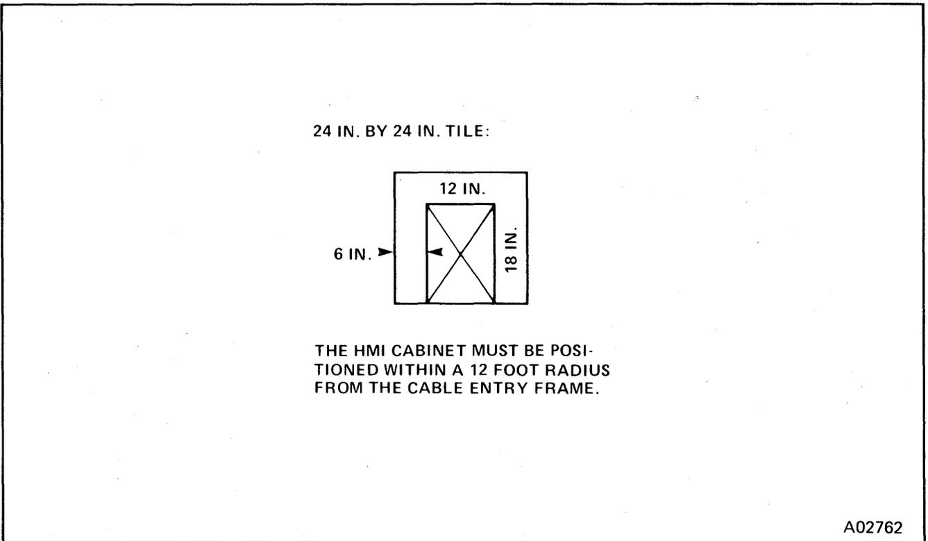
Figure 48. HMI (Option), Raised-Floor Tile Cutout
