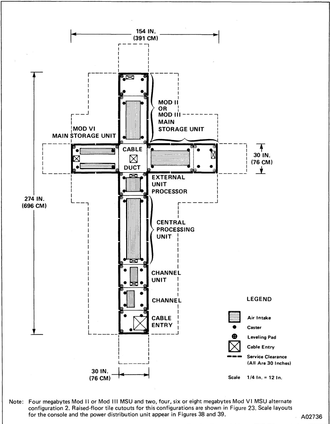
Figure 22. V/5 and V/6 Scale Layout Showing "Long-Right-L", Alternate Configuration 2
