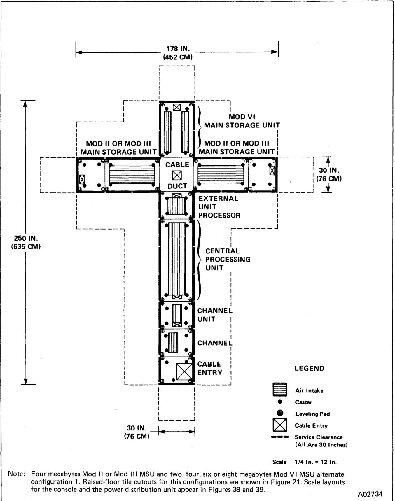
Figure 20. V/5 and V/6 Scale Layout Showing "Balanced-L", Alternate Configuration 1
