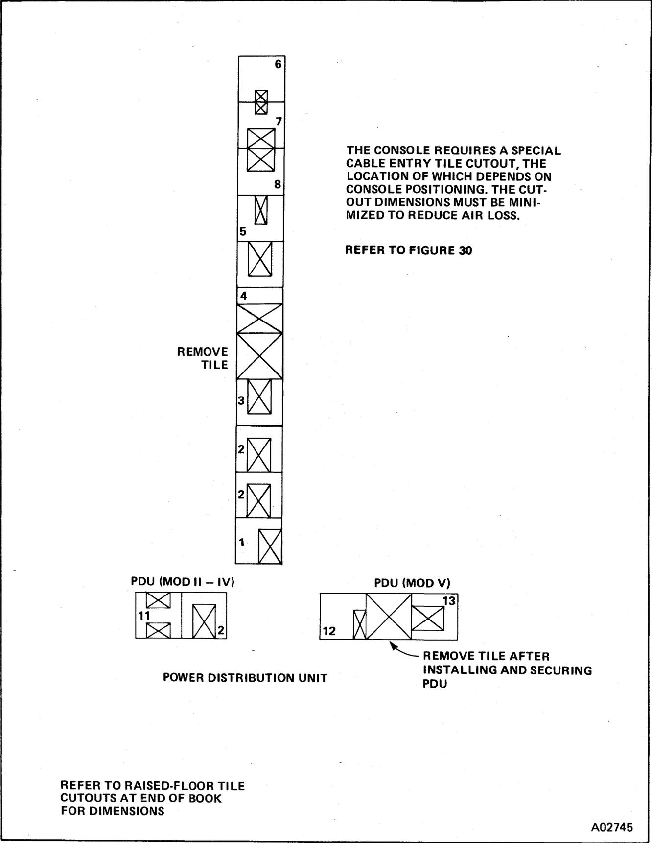
Figure 31. V/7 and V/8 Configuration 1, (With Cable Ducts). Raised-Floor Tile Installation Pattern.
