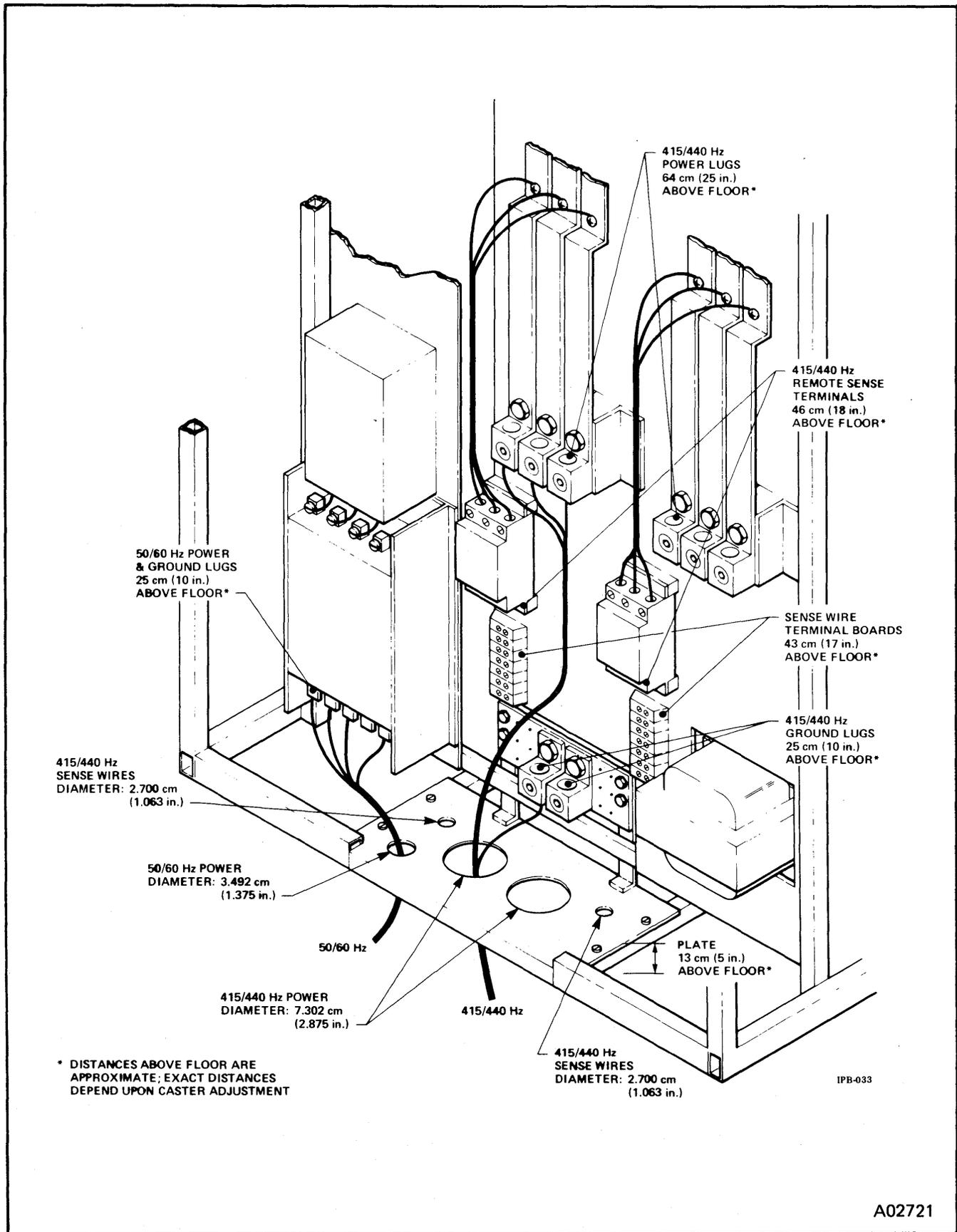
Figure 7. PDU MOD V, Interconnection Wiring Block
