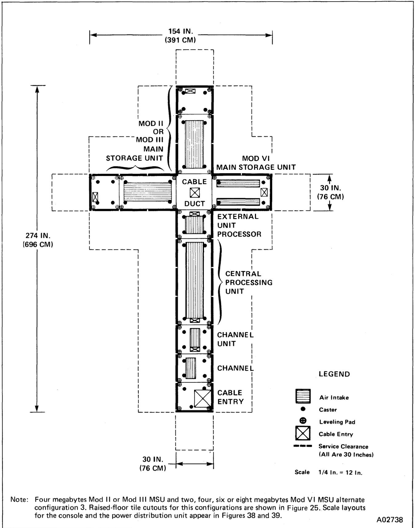
Figure 24. V/5 and V/6 Scale Layout Showing "Long-Left-L", Alternate Configuration 3
