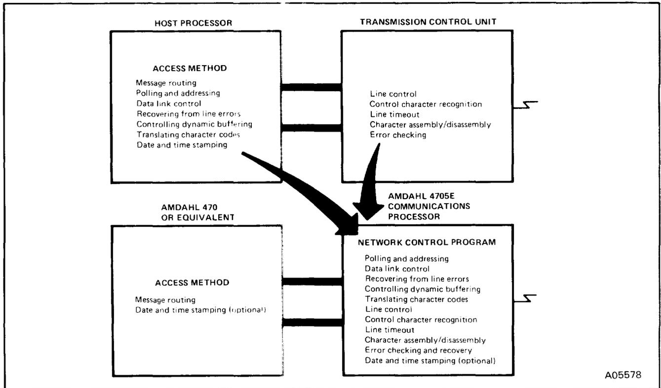
Figure 1. Centralization of Function in the AMDAHL 4705E
