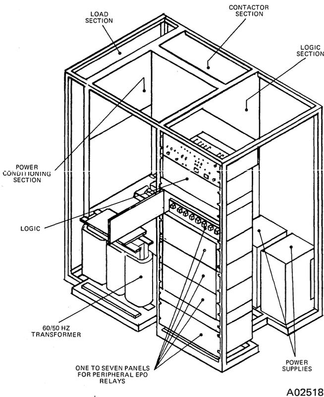
Figure 2. The 580 Power Distribution Unit
