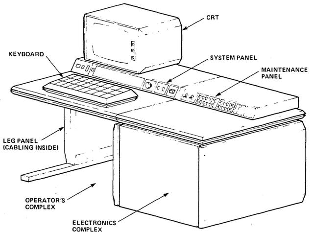
Figure 3. The 580 Main Operator's Console
