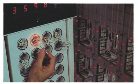
2048 sub-channels are standard. The 470V/8 offers full channel configuration flexibility, with each of the 12 or 16 channels configurable as a byte or block multiplexer or a selector channel, in any combination. Selector and block multiplexer channels can handle data transfer rates of approximately 2 megabytes/second, and byte multiplexer channels handle 110 kilobytes/second.
