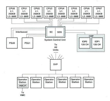
CH: Channel 1.1: Level 1 Cache CHP: Channel Processor L2: Level 2 Cache CPU: Central Processing Unit PSU: **Processor Storage Unit** HMC: Hardware Management Console SC: System Controller HMCIF: **HMC Interface Feature** System Data Switch SDS: IOP: I/O Processor SVP: Service Processor
