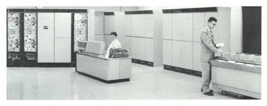
Ampex Computer Tape Handlers installed in a GE-100 data-handling system. These instruments are also used in the G.E.-built Bank of America ERMA system. Both the computers provide automated, accurate high-speed handling of bank accounts.
