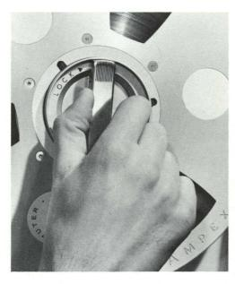
New Ampex expanding reel holddowns provide quick, positive locking and release with a quarter turn. These devices automatically center the tape reel and position it properly and accurately on the turntable with respect to the tape transport and all tape-guiding surfaces.
