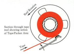
Tape-Packer Arm presses incoming tape against pack, forcing out inter-layer air which would otherwise be whipped into the pack.
