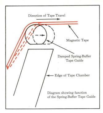
As the tape is pulled forward at the initiation of a "start" command, the Spring-Buffer Tape Guide moves too, supplying a minute length of tape just at the proper instant. This greatly decreases the effects of static friction, air-pressure resistance and tape inertia, allowing much quicker, gentler start times.
