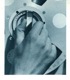
New Ampex expanding reel holddowns provide quick, positive locking and release with a quarter turn. These devices automatically center the tape reel and position it properly and accurately on the turntable with respect to the tape transport and all tape-guiding surfaces.
