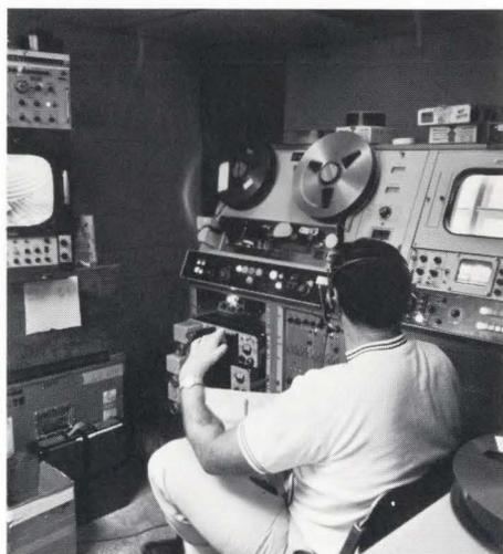
Underneath the Olympic Stadium, this VR-2000 worked in conjunction with an HS-100 to record many events and select segments for slow and stop motion. Scene on monitor at left is from ABC's crane-mounted camera high over stadium.
