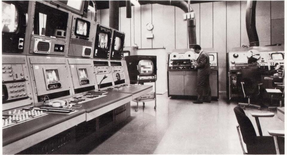
Control and recorder room at ZDF (Second Network) color broadcasting facility near Mainz with two of the five VR-2000's located here. The entire ZDF network uses some 24 Ampex videotape machines.
