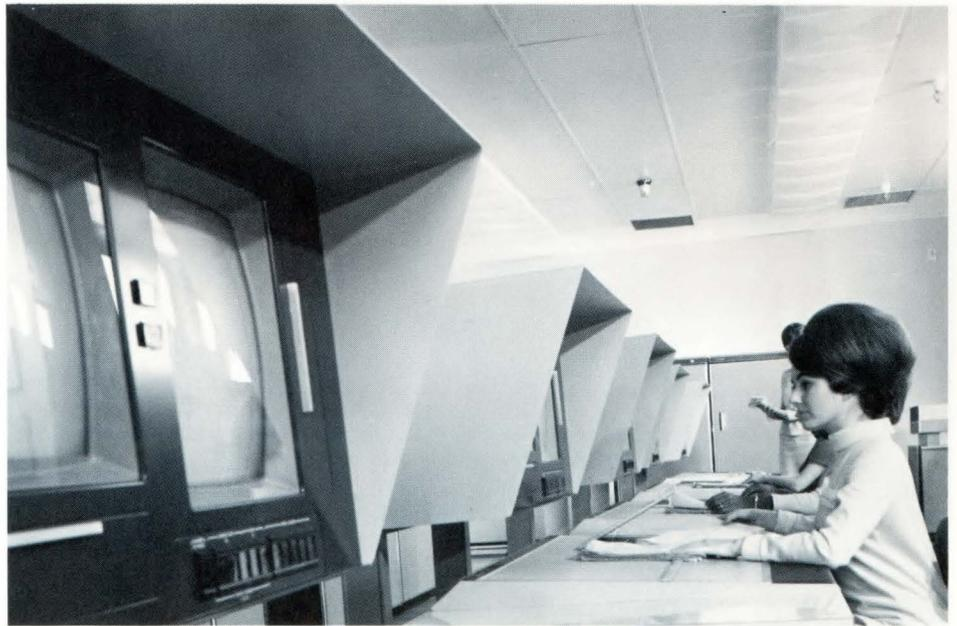
Filing consoles in the Videofile System at Southern Pacific. Waybills are filed instantaneously with their digital address as electronic images on magnetic tape.
