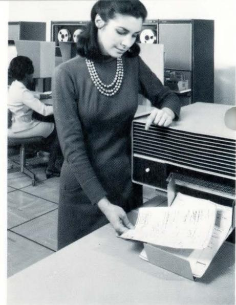
Documents in a Videofile System are available as soft copy images on a display screen or as hard copies from an electrostatic printer. This unit at Southern Pacific prints out hard copies of waybills.
