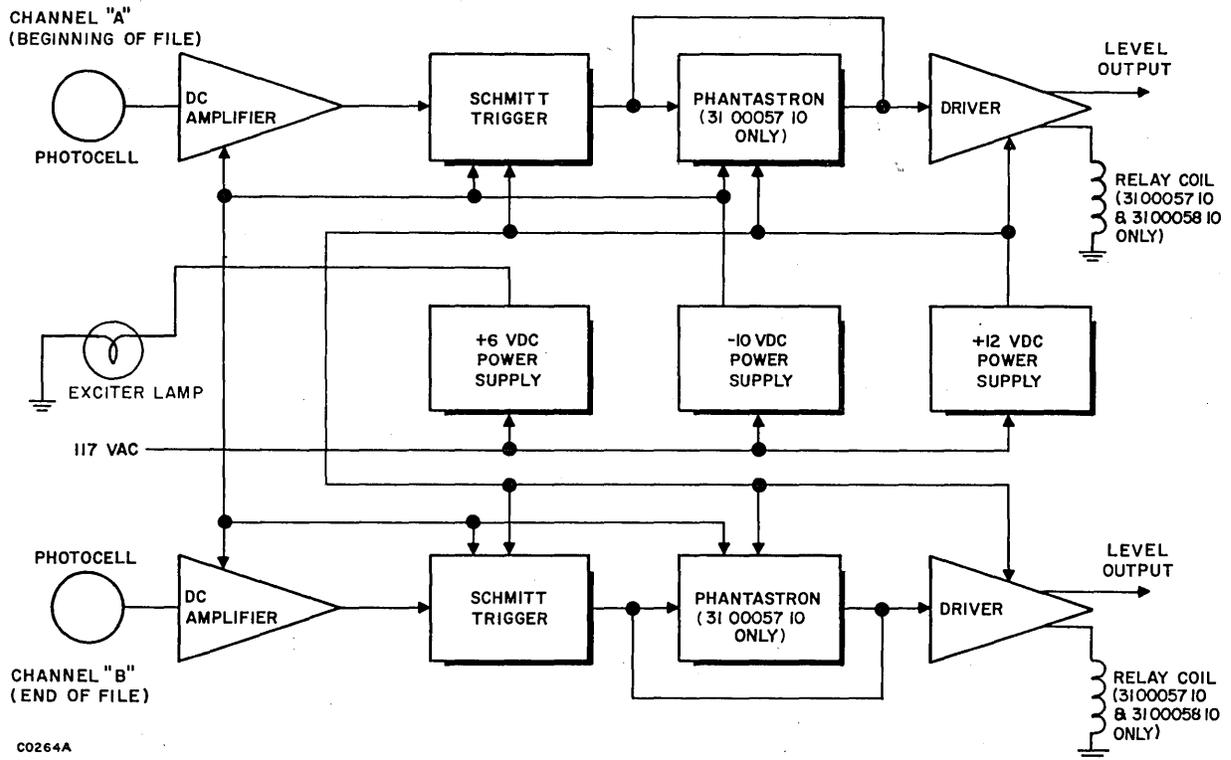
Figure 4-10. Block Diagram of Photosensor Kit
