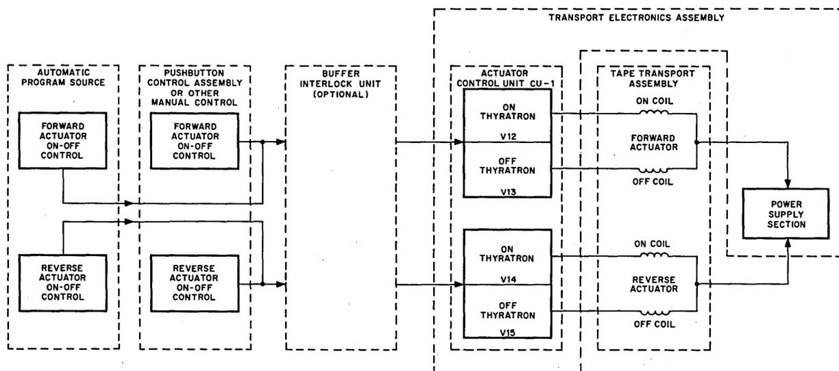
Figure 4-5. Block Diagram of Actuator Control System
