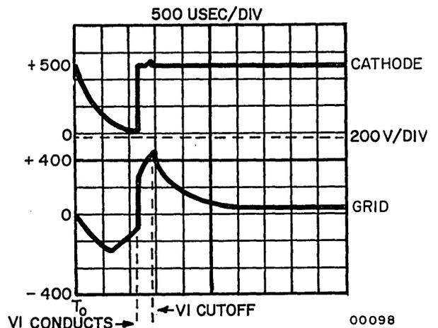
Figure 4-9. Voltage Waveforms, Cathode and Grid of V1
