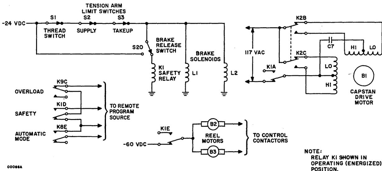
Figure 4-2. Tension Arm Limit Switch and Motor Details
