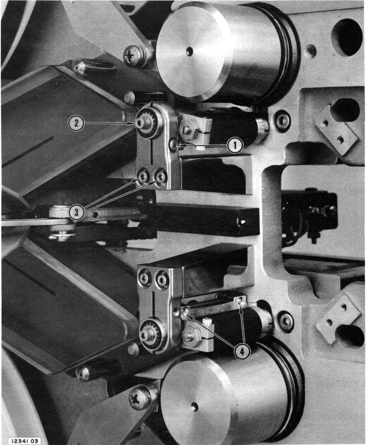
Figure 5-16. Removing Capstan Roller Assembly
