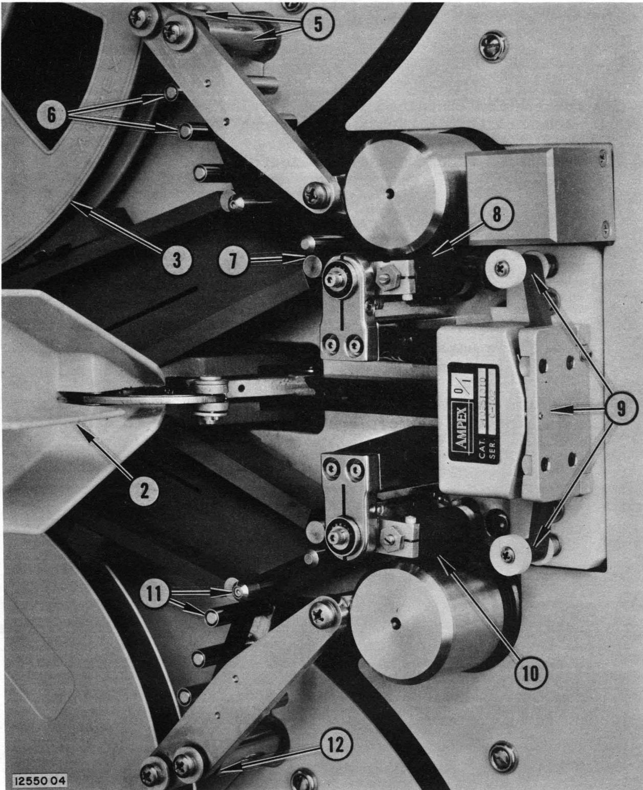
Figure 3-1. Threading the Tape Transport
