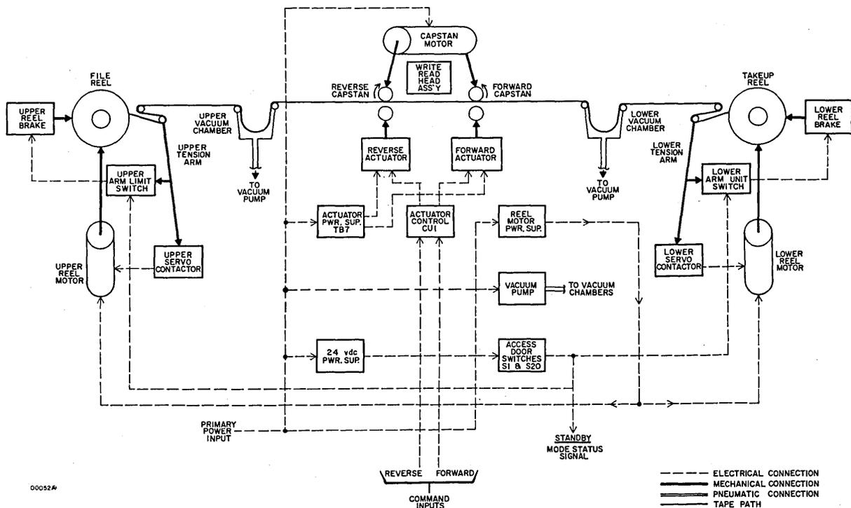
Figure 1-2. Block Diagram of Tape Transport and Transport Electronics
