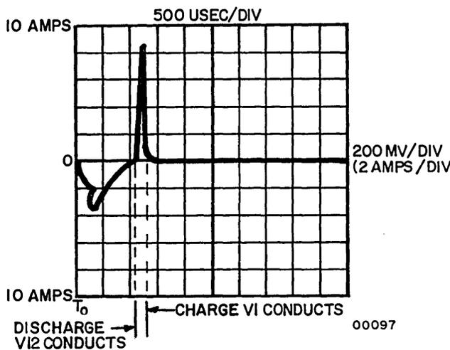
Figure 4-8. Current Waveform, Discharge and Charge of C4
