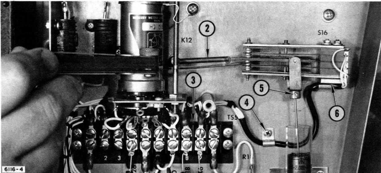
Figure 5-18. Removing Servo Contactor
