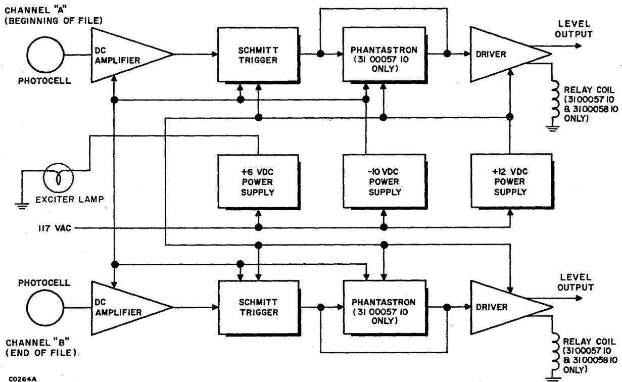
Figure 1-3. Block Diagram of Photosensor Electronics System
