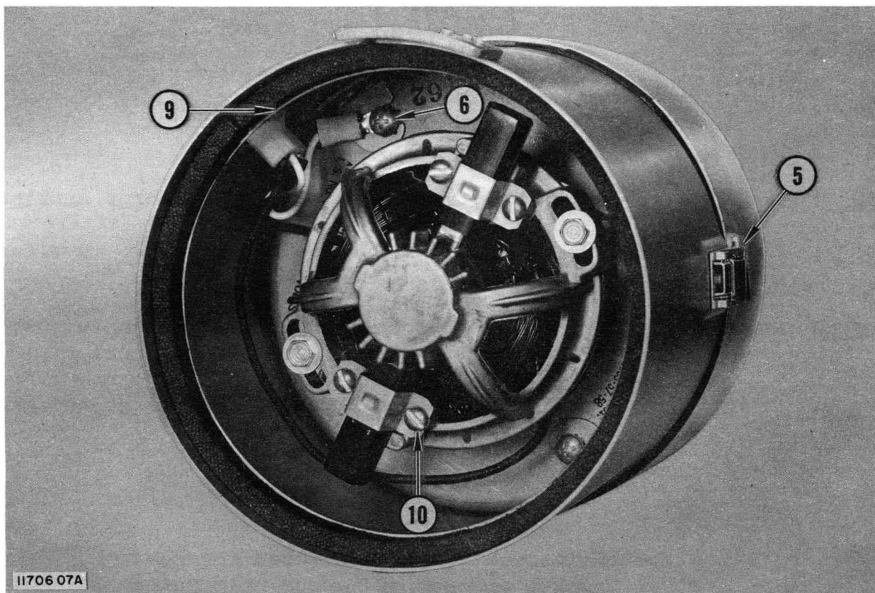
Figure 5-20. Removing Vacuum Unit Motor and Brushes
