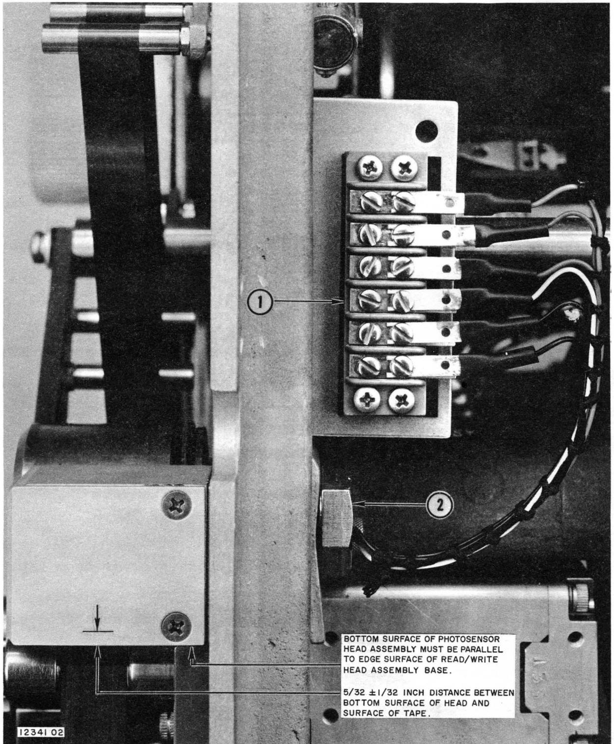
Figure 5-23. Removing Photosensor Head Assembly
