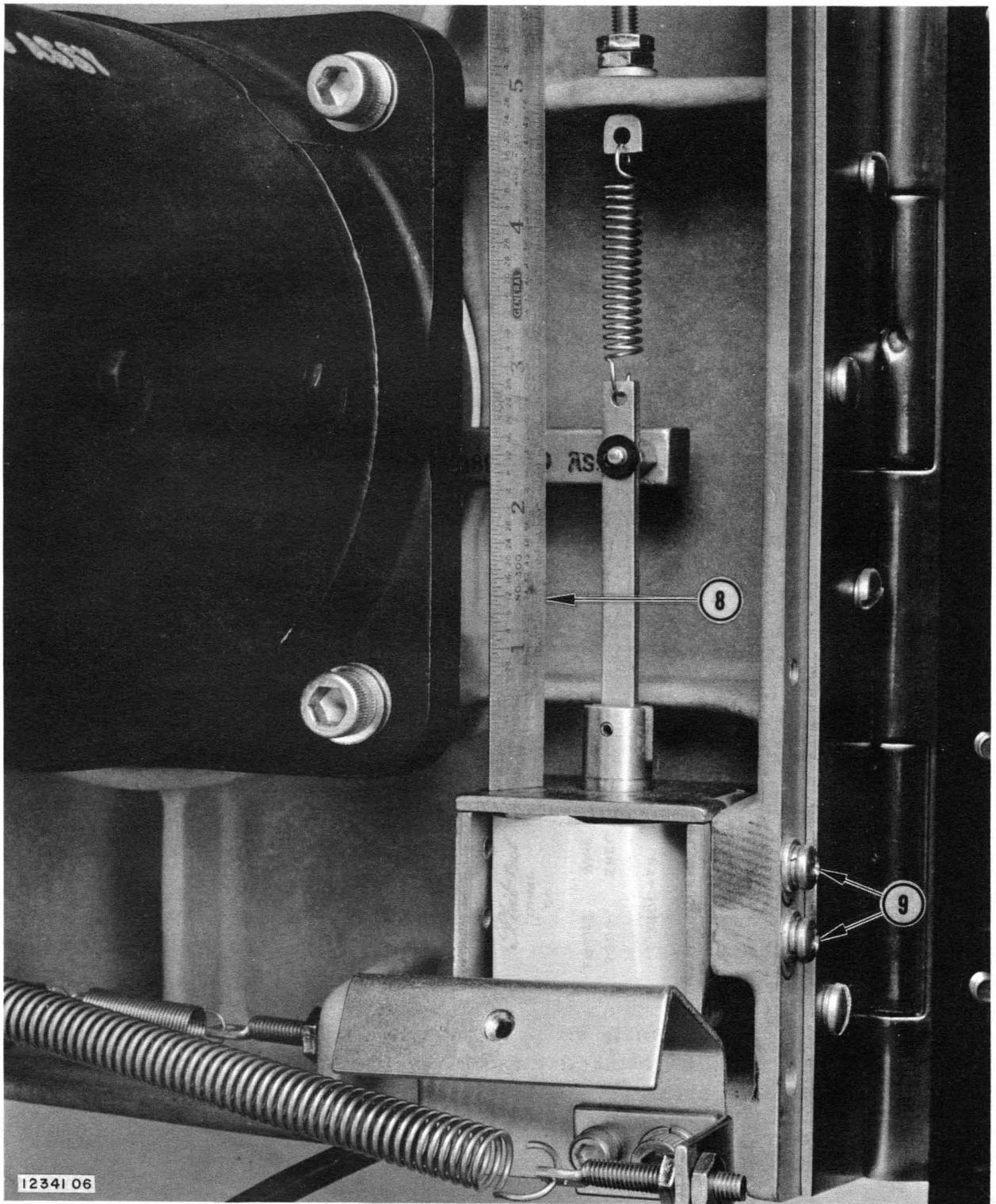
Figure 5-14. Adjusting Reel Brake
