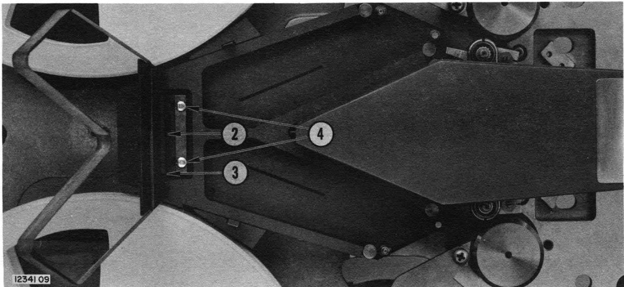
Figure 5-22. Removing Vacuum Chamber Door
