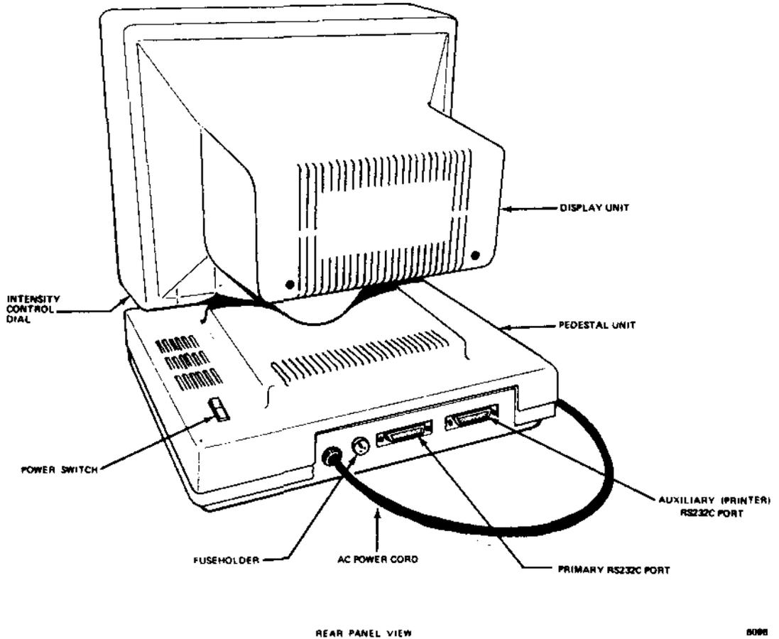
Figure 1-4. Terminal, Rear View
