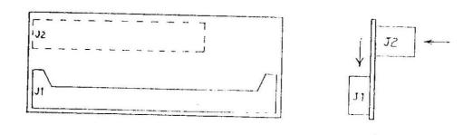
Attach the WPC5F to the disk drive as shown below. The 34-line PC edge connector of the WPC5F attaches to the 34-line connector of the disk drive. Plug the 50-line cable from the UDC11 into the 50-line connector of the WPC5F.
