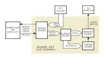
roll/page and command set operations. The Serial board converts incoming serial data to bit-parallel for the Cursor board, converts bit-parallel keyboard data to serial for transmission, and provides gating for local, half-, and full-duplex operation.
