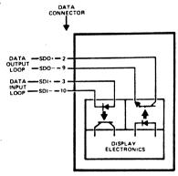
Note: For half-duplex operation, jumper pin 3 to pin 9 on mating connector.
