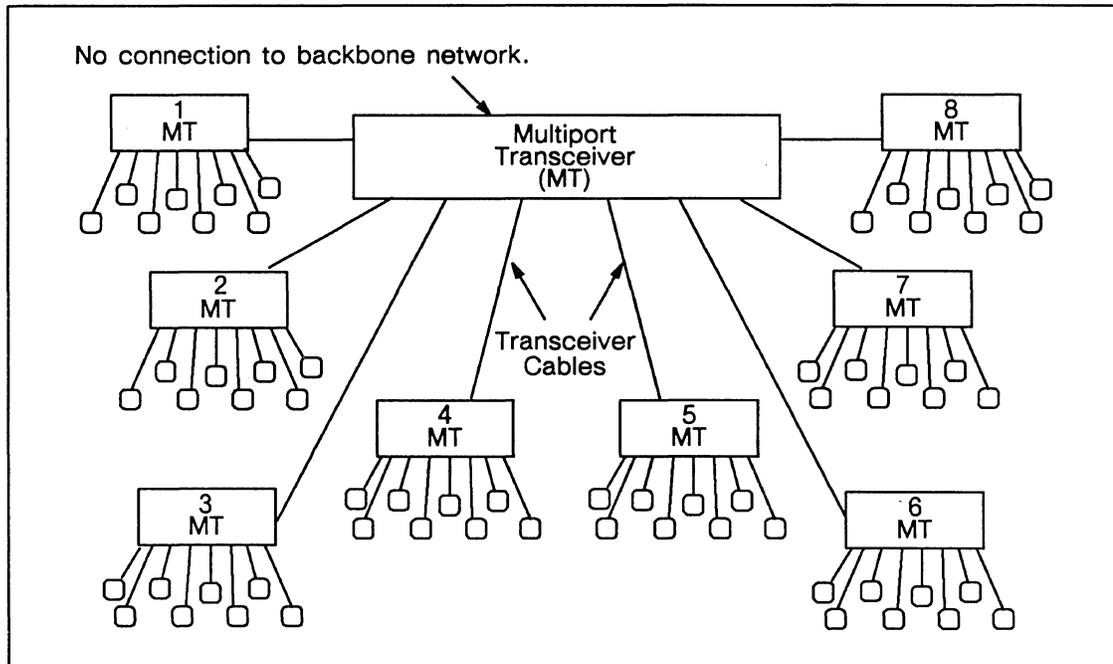
Figure 6-5. Multiport Transceiver in a Stand-Alone, Star-Wired Network
