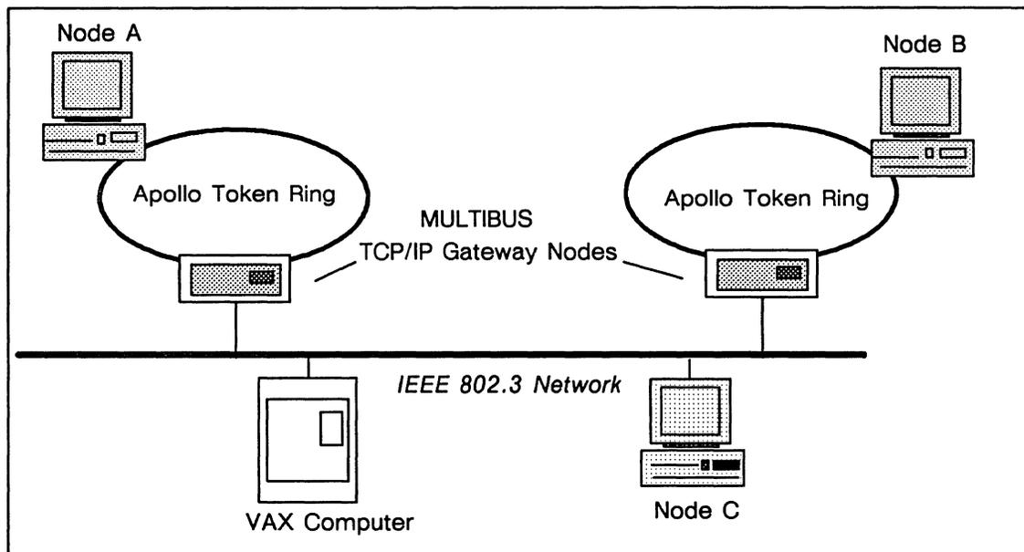
Figure 8-14. MULTIBUS Gateway Nodes Connecting ATRs to an IEEE 802.3 Network
