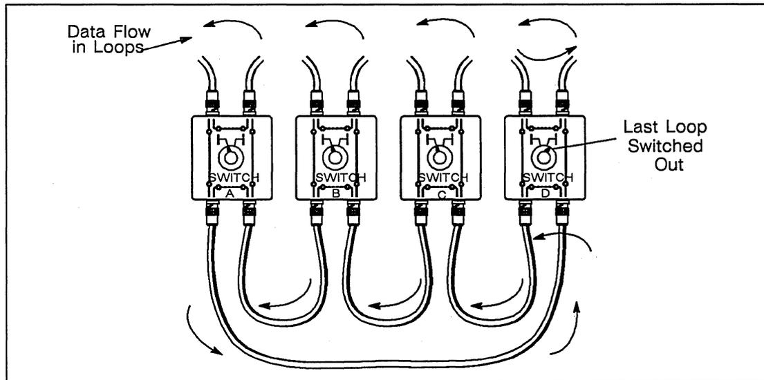
Figure 3-5. Data Flow Through the Network Switch and Several Loops
