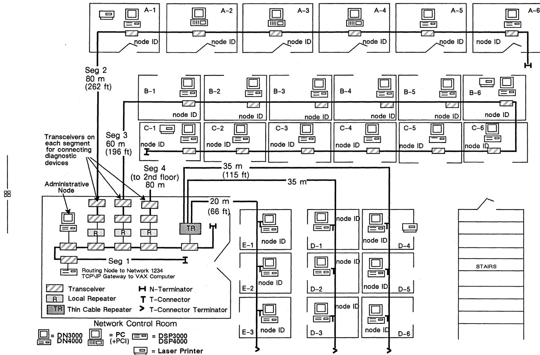
Figure 6-9. Sample IEEE 802.3 Network Layout Diagram
