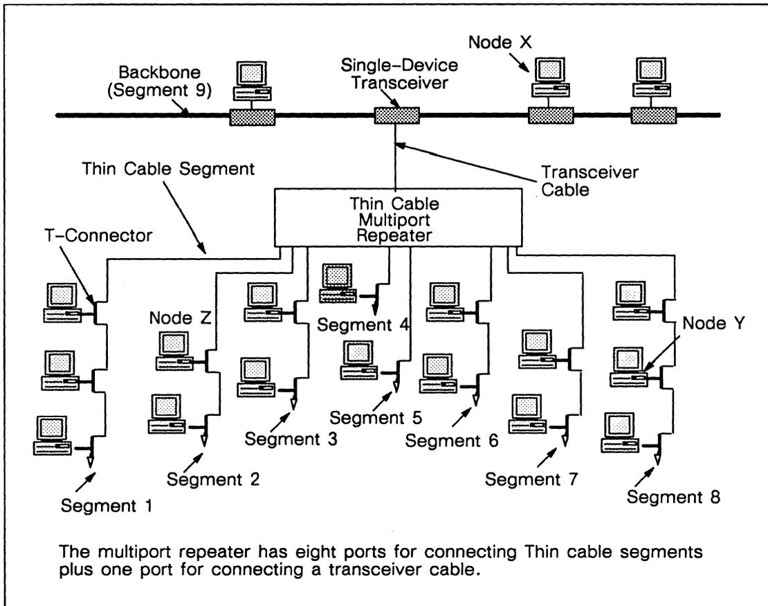
Figure 6-8. Thin Cable Repeater Configurations
