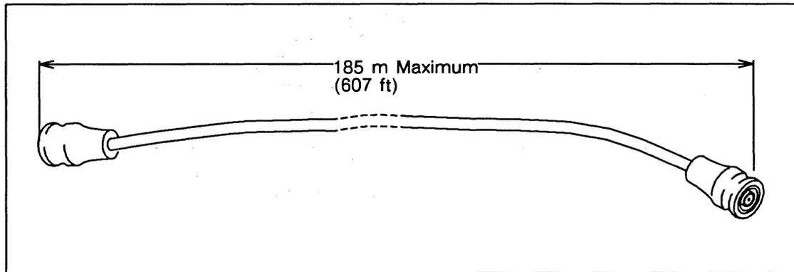
Figure 5-3. Thin Cable Segment
