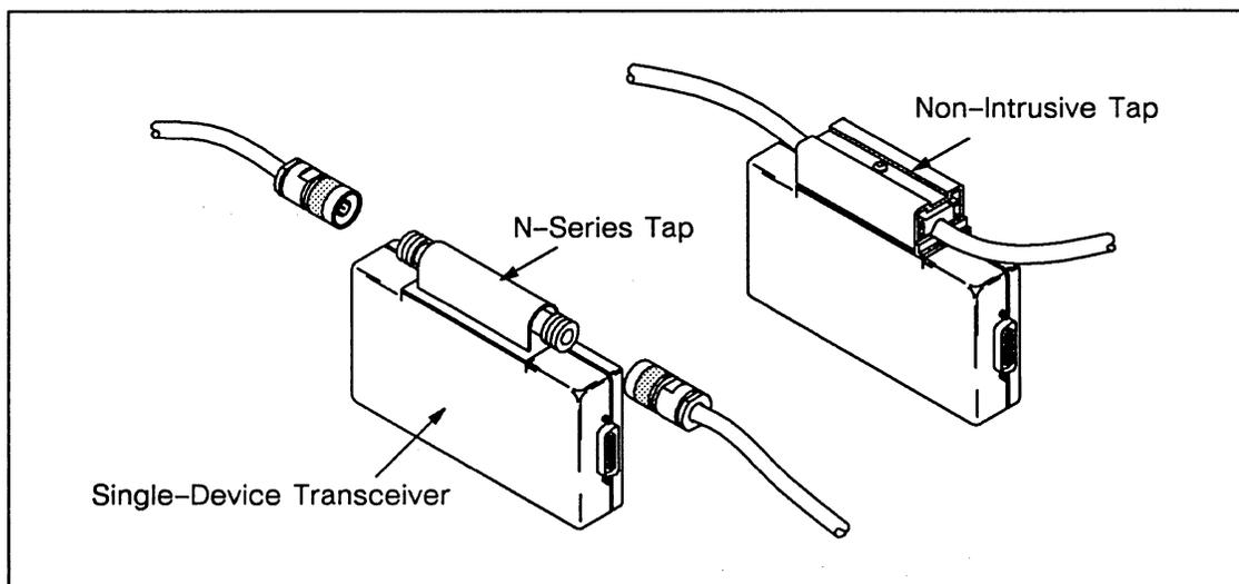
Figure 5-8. N-Series Transceiver Tap
