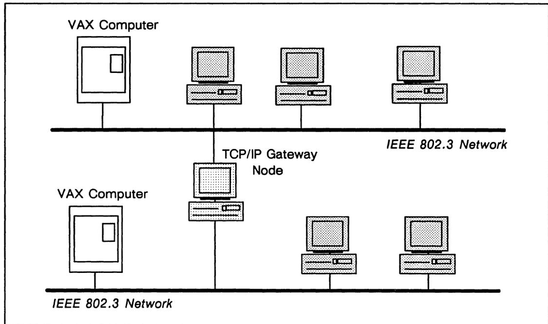
*Figure 8-8. Direct Connection Internet Configuration Between Two IEEE 802.3 Networks*
