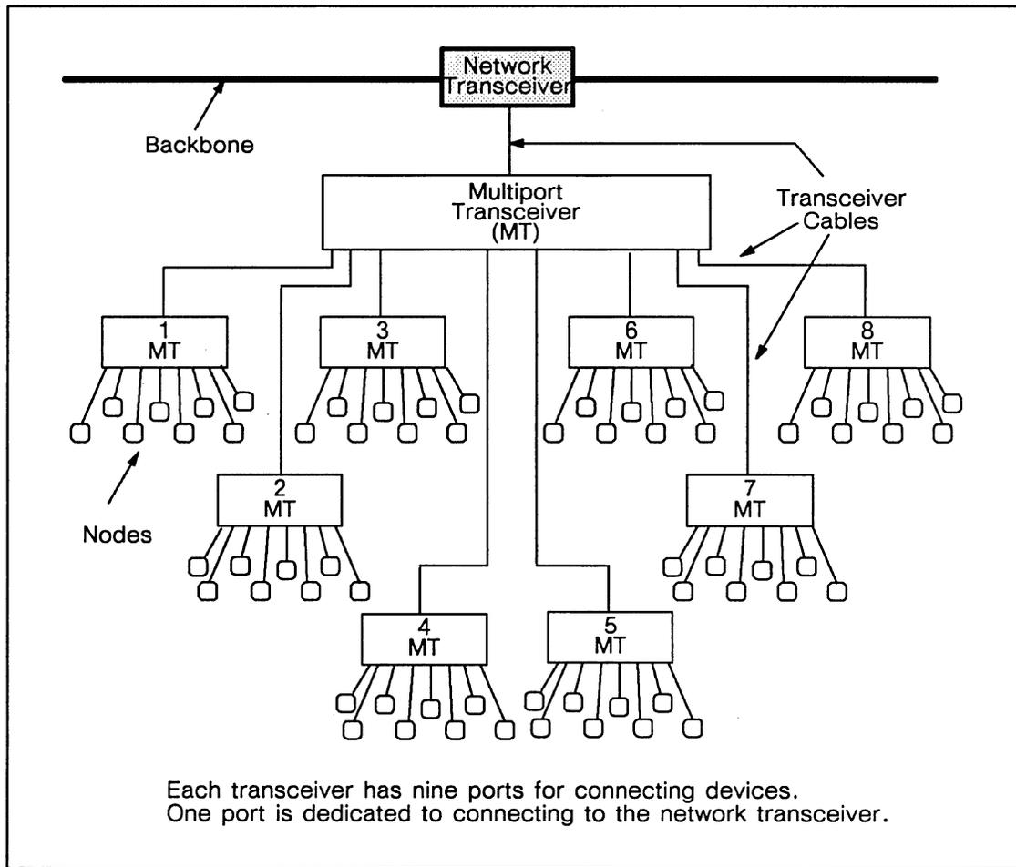
Figure 6-4. Multiport Transceiver in a Cascaded Configuration
