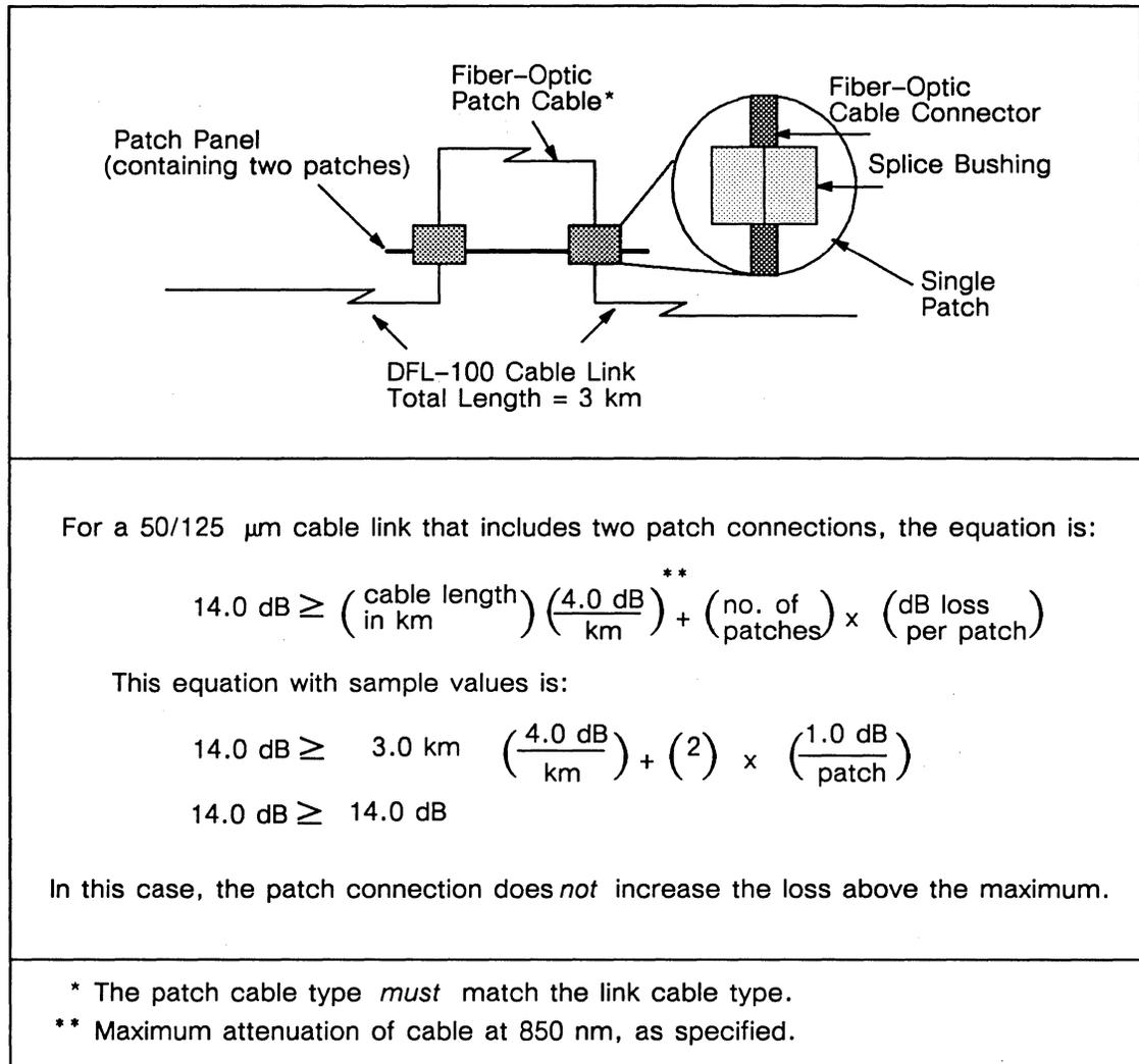
Figure B-1. Sample Attenuation Calculations for DFL-100 Link with Patch Panel
