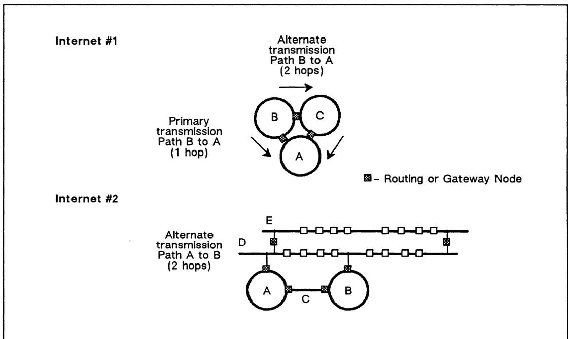
Figure 8-2. Using Redundant Communication Paths
