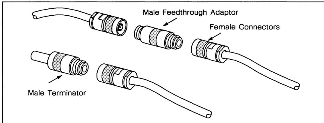
*Figure 5-2. N-Series Cable Connectors and Terminators*
