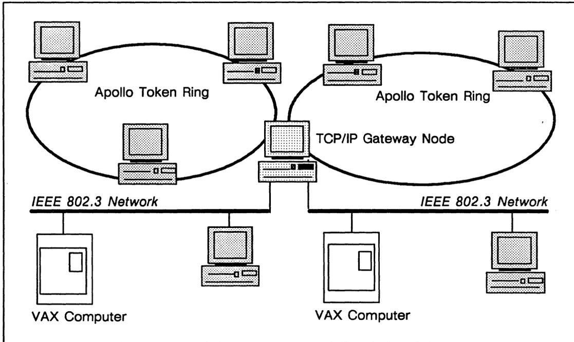
Figure 8-12. Maximum Number of Networks Connected to a Single TCP/IP Gateway Node
