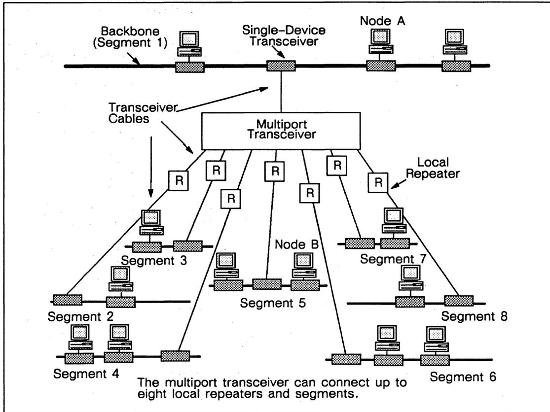
Figure 6-7. Multiple Local Repeaters Connected with a Multiport Transceiver
