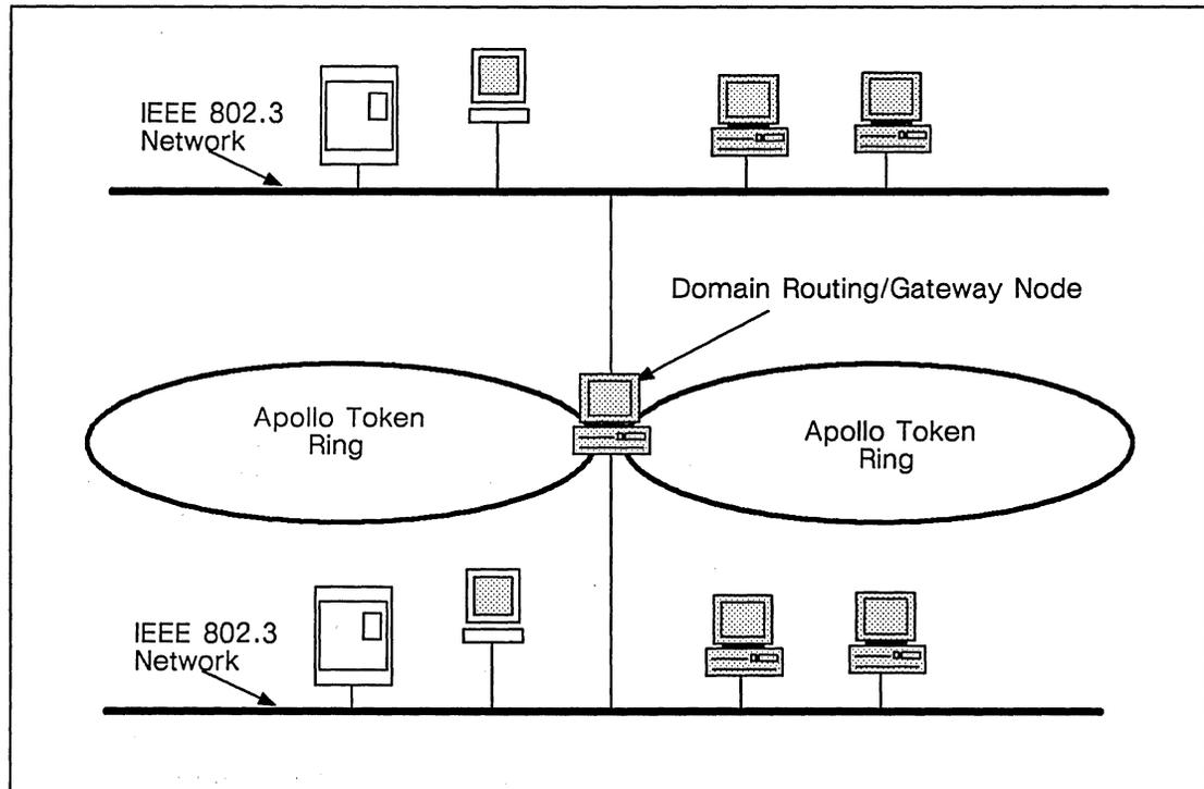
Figure 7-4. A Single Node Joining Four Networks
