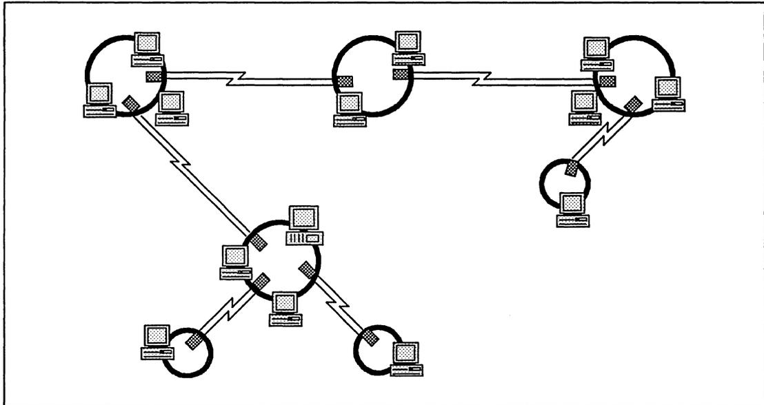
Figure 2-6. DFL-100 Extended Ring Spanning Seven Sites
