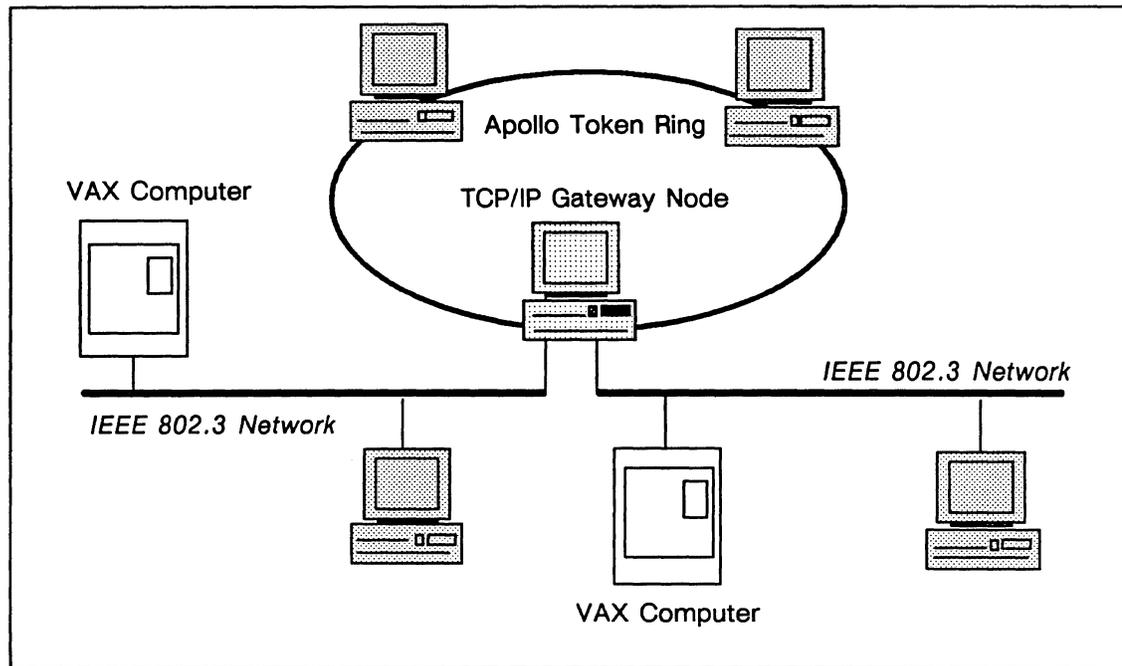
Figure 8-11. TCP/IP Gateway to Two IEEE 802.3 Networks and an Apollo Token Ring
