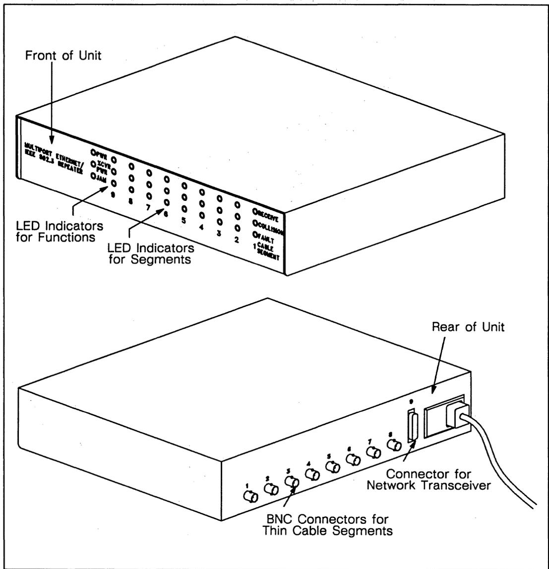
Figure 5-10. Thin Cable Multiport Repeater
