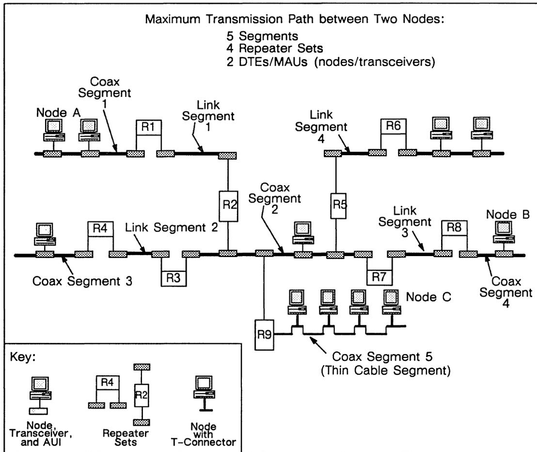
Figure 6-3. A Large IEEE 802.3 Network Illustrating Maximum Transmission Paths
