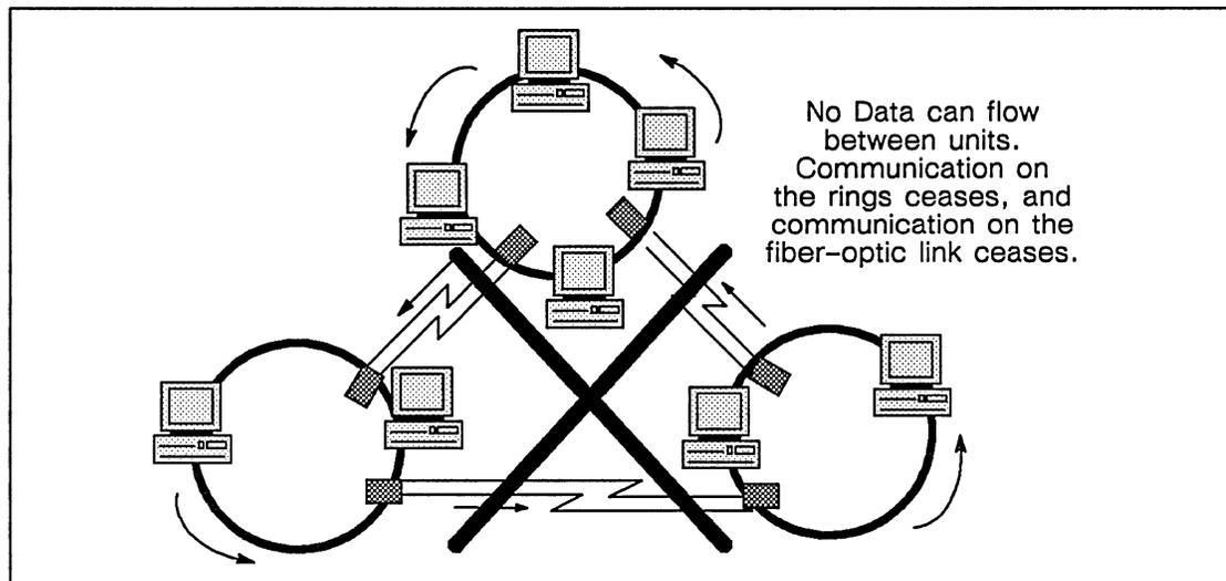
Figure 4-6. An Inoperable Redundant DFL-100 Configuration
