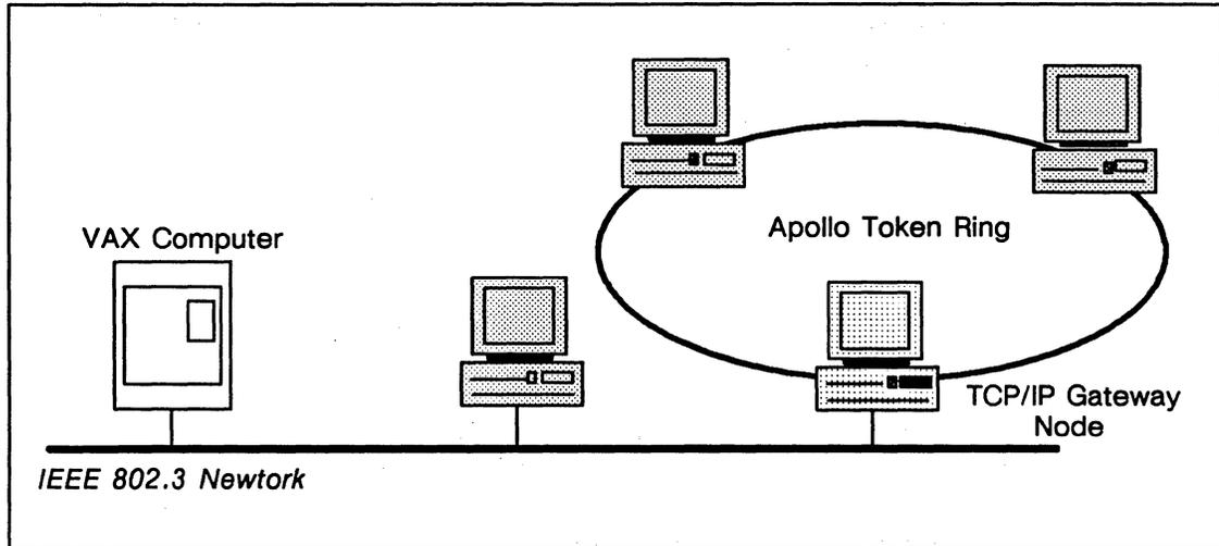
*Figure 8-9. AT-Compatible TCP/IP Gateway Between an IEEE 802.3 and Apollo Token Ring Network*
