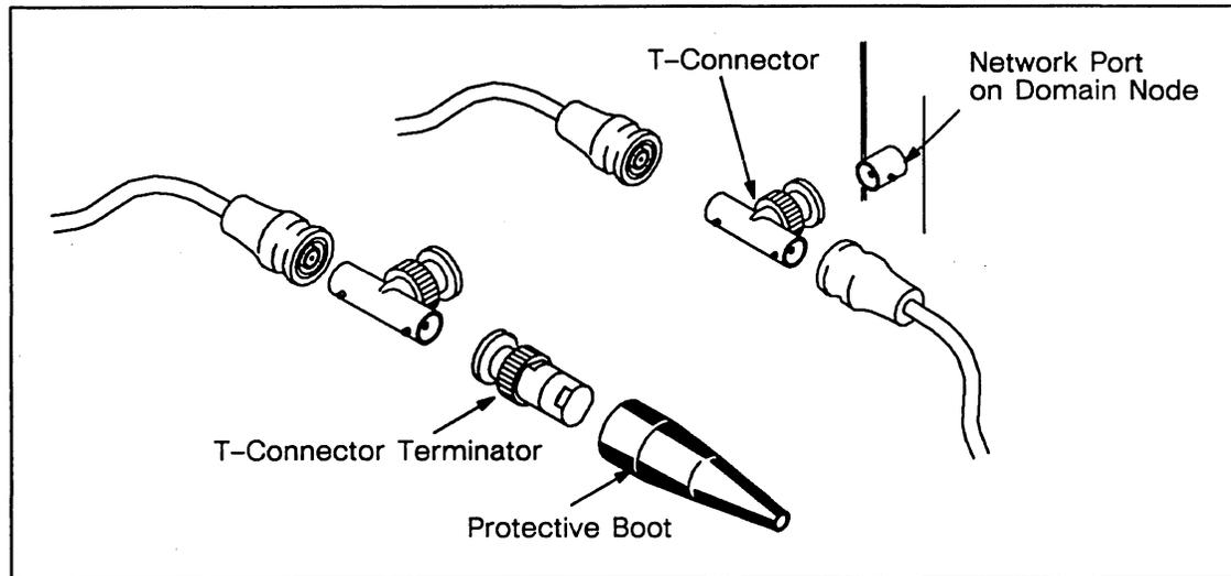
Figure 5-4. Thin Cable T-Connector and Terminator
