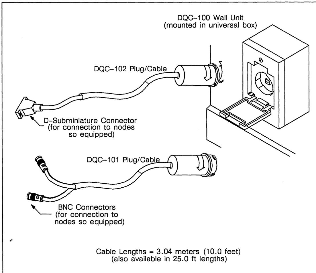
Figure 3-2. The Domain/DQC Quick Connect System
