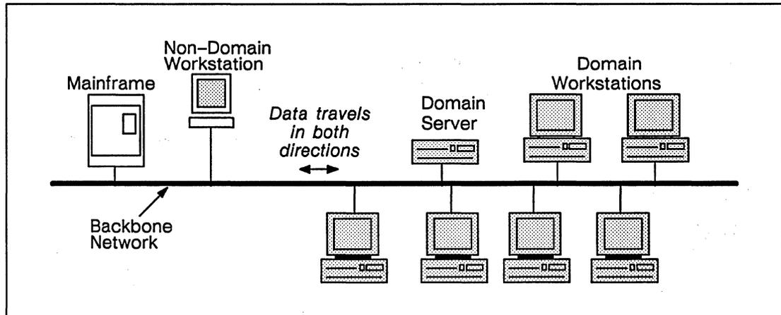
Figure 2-8. Single-Backbone IEEE 802.3 Network
