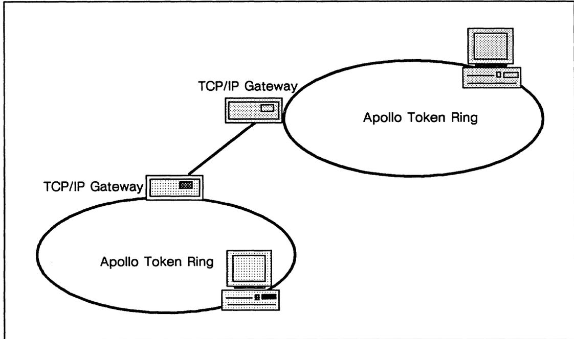
Figure 8-13. Two MULTIBUS TCP/IP Gateway Nodes in a Point-to-Point Configuration
