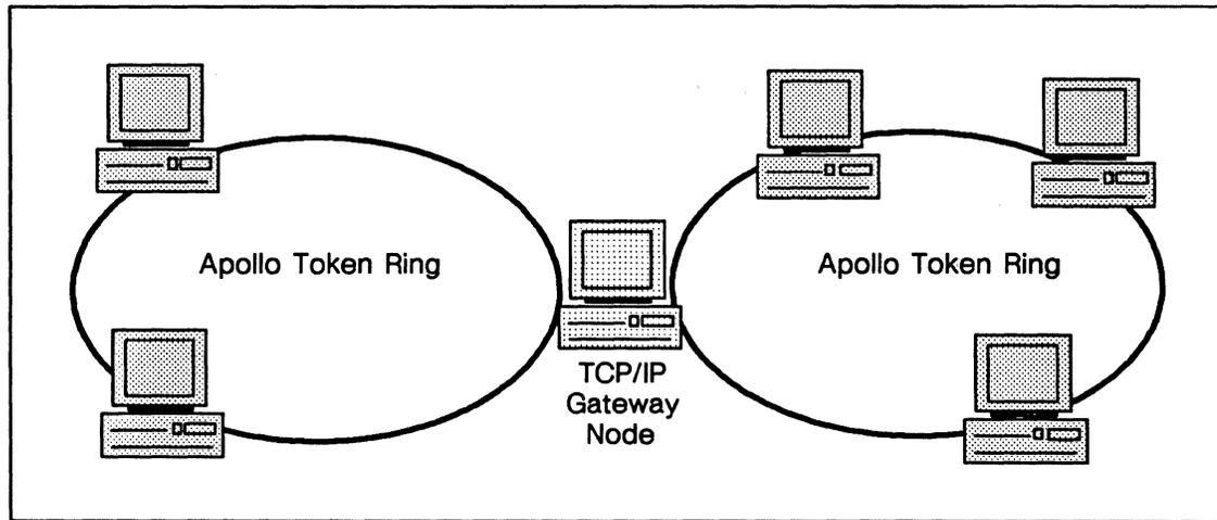
*Figure 8-10. AT Compatible Node as a Gateway Between Two Apollo Token Rings*
