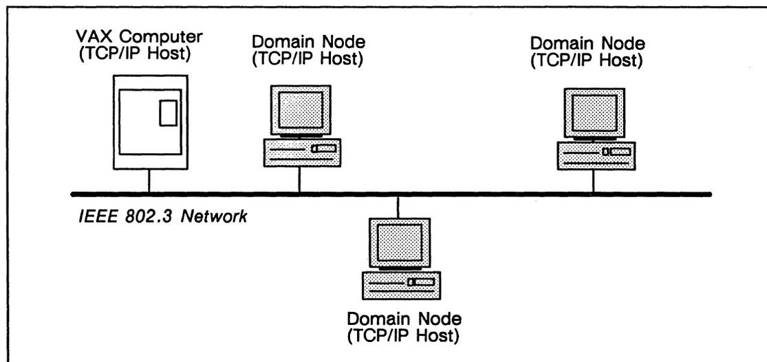
Figure 8-7. TCP/IP Hosts on an IEEE 802.3 Network
