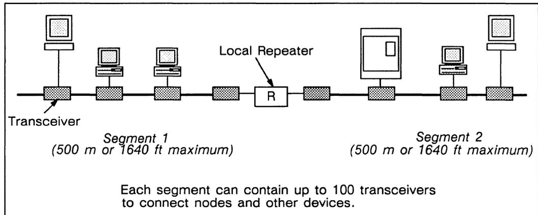
*Figure 6-6. Two Segments Connected with a Local Repeater*
