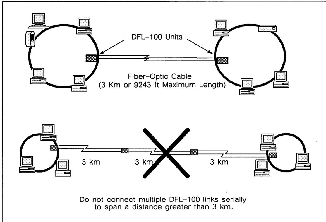
Figure 4-2. Proper and Improper DFL-100 Configurations
