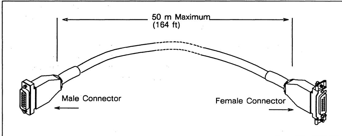
Figure 5-7. Transceiver Cable
