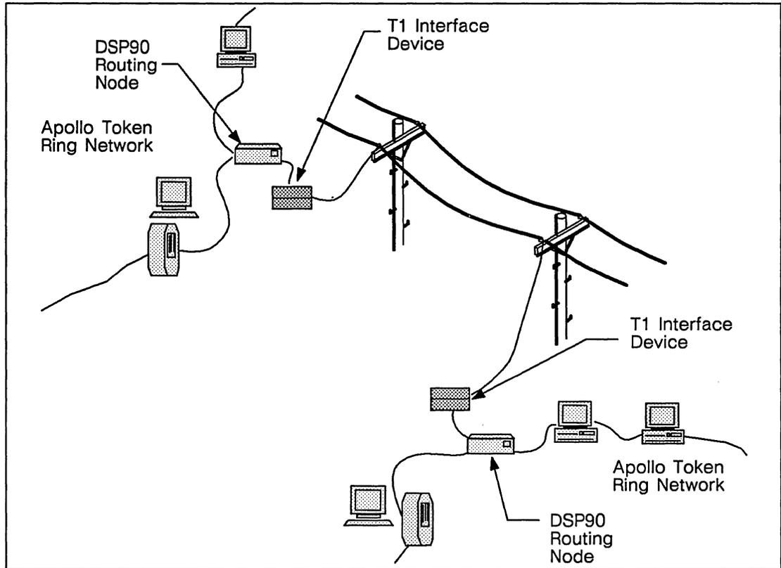
Figure 7-2. A Point-to-Point Link Using T1 Service
