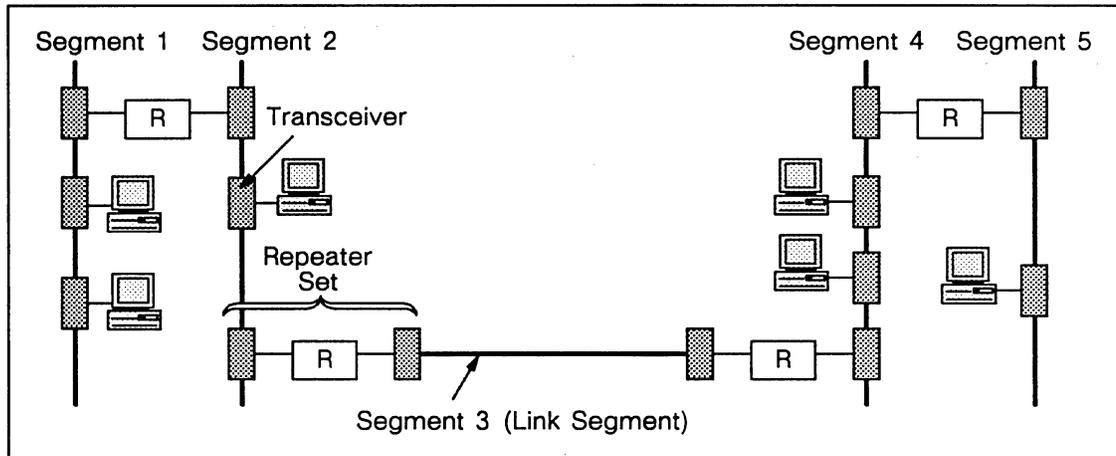
Figure 6-1. Standard Cable and Link Segments Connected in Series
