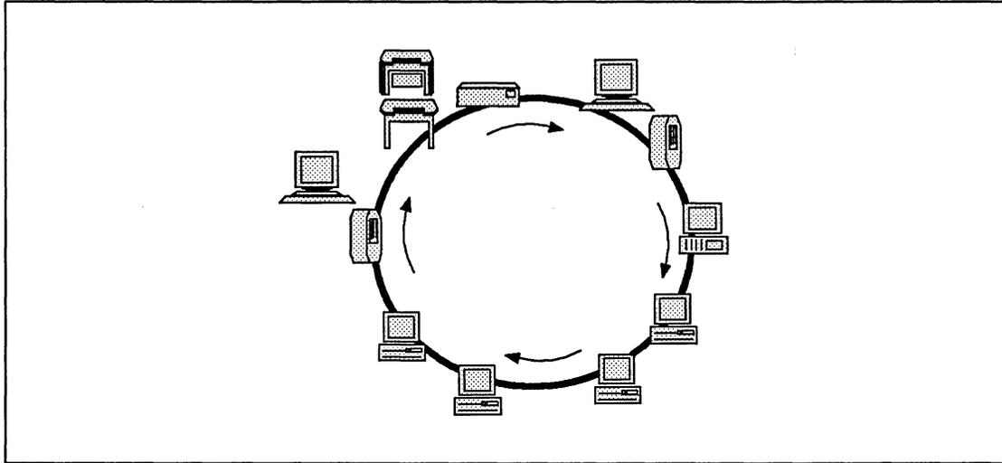
*Figure 2-1. Serially-Wired Apollo Token Ring Network*
