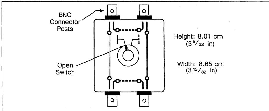
Figure 3-4. The Network Switch
