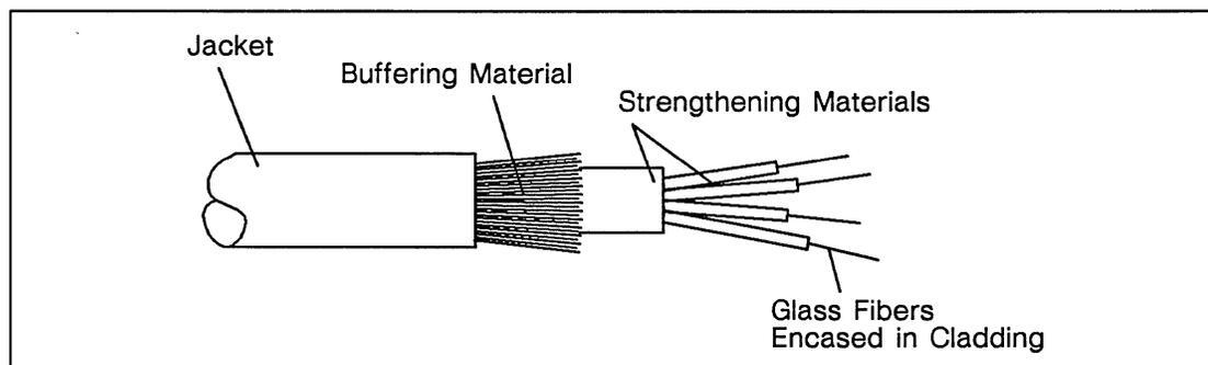
*Figure 3-7. Fiber-Optic Cable Cross Section*
