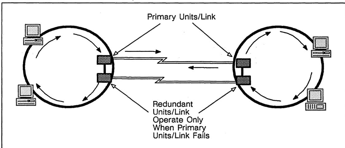
Figure 2-7. Redundant DFL-100 Configuration
