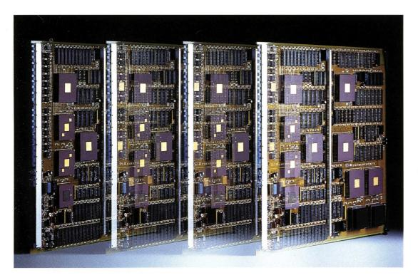
The Series 10000 supports up to four central processors—each with an independent integer processor, FPU, dual caches, and memory management unit.
