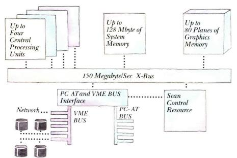
The Series 10000's wellbalanced architecture means all system components are designed to work together to deliver high system performance. parallelism of its multiprocessor design, and thereby deliver unrivaled *system* performance.
