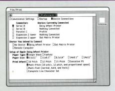
Printer set-up options such as paper size and type, and print wheels are all controlled from within Lisa applications. Simply point with the mouse to select each option.
