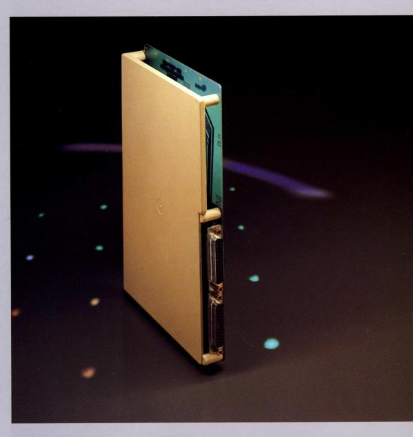
The Parallel Interface Board enables your Lisa™ system to accommodate peripherals structured with a parallel interface, such as Apple's ProFile™ hard disk and the Apple Dot Matrix Printer.
