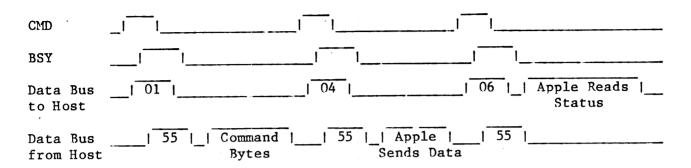
Important: The host must raise CMD following the last operation requested, since changes in Profile's spare and bad block tables do not get rewritten onto the disk until this occurs.
