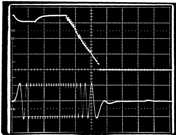
WAVEFORM: DAC Output and Position A
