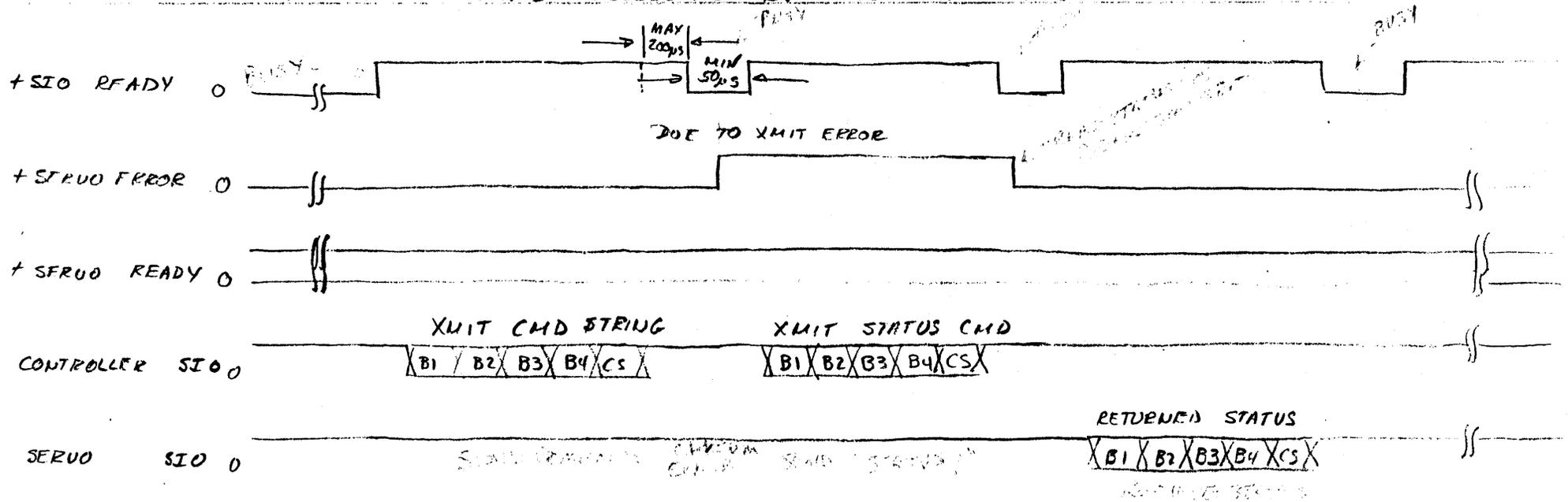
CONDITIONS: Servo is ready (track following) <sup>or not</sup>. Transmitted command and/or checksum had bit error (servo error goes active).
