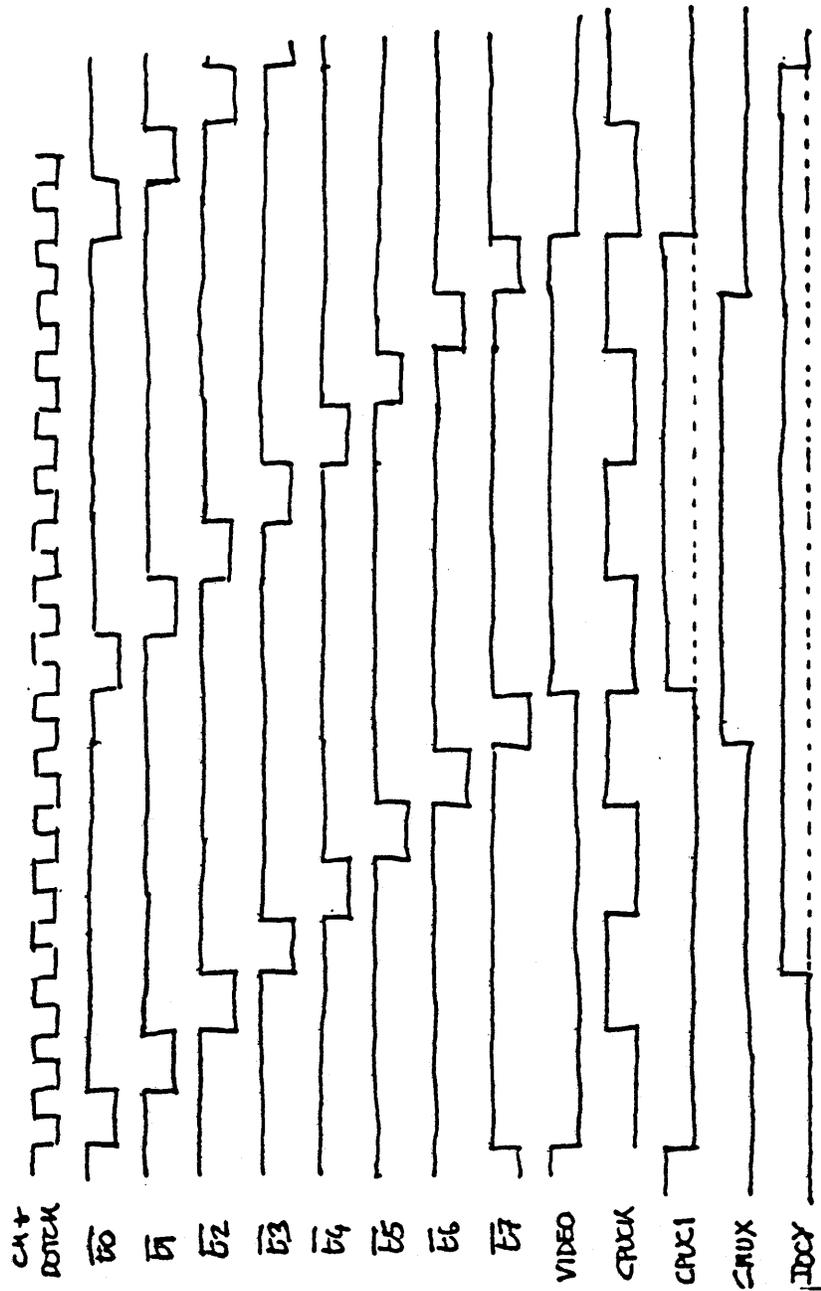
Figure 4-12. Processor Board Timing Generation
