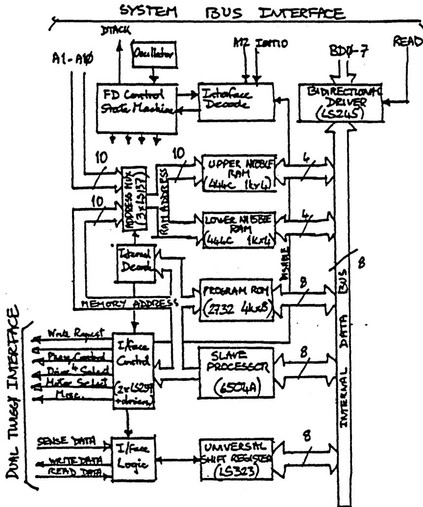
Figure 6-2. Floppy Disk Controller Block Diagram
