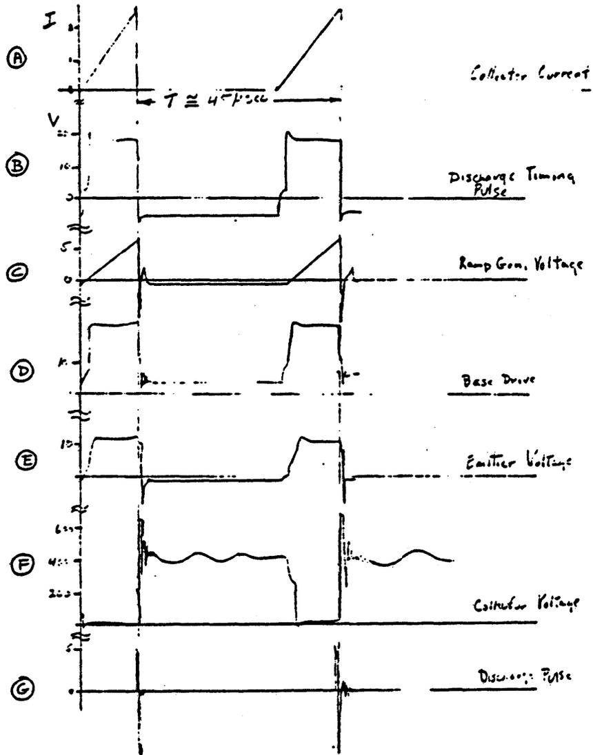
Figure 10-4. Flyback Oscillator Waveforms
