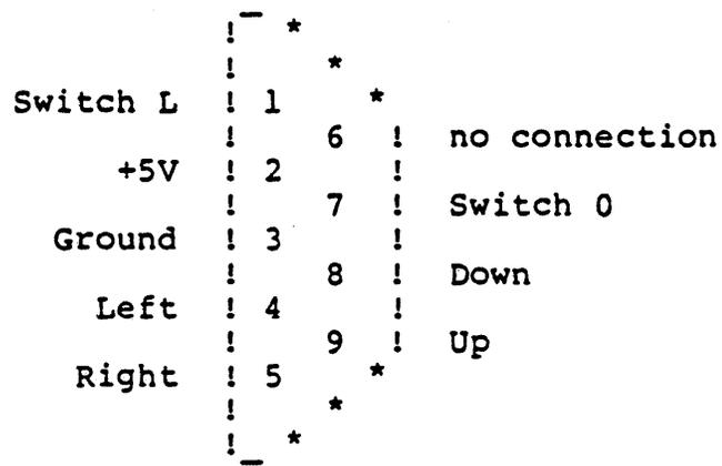
Figure 3-11. Mouse Interface Pin Assignment
