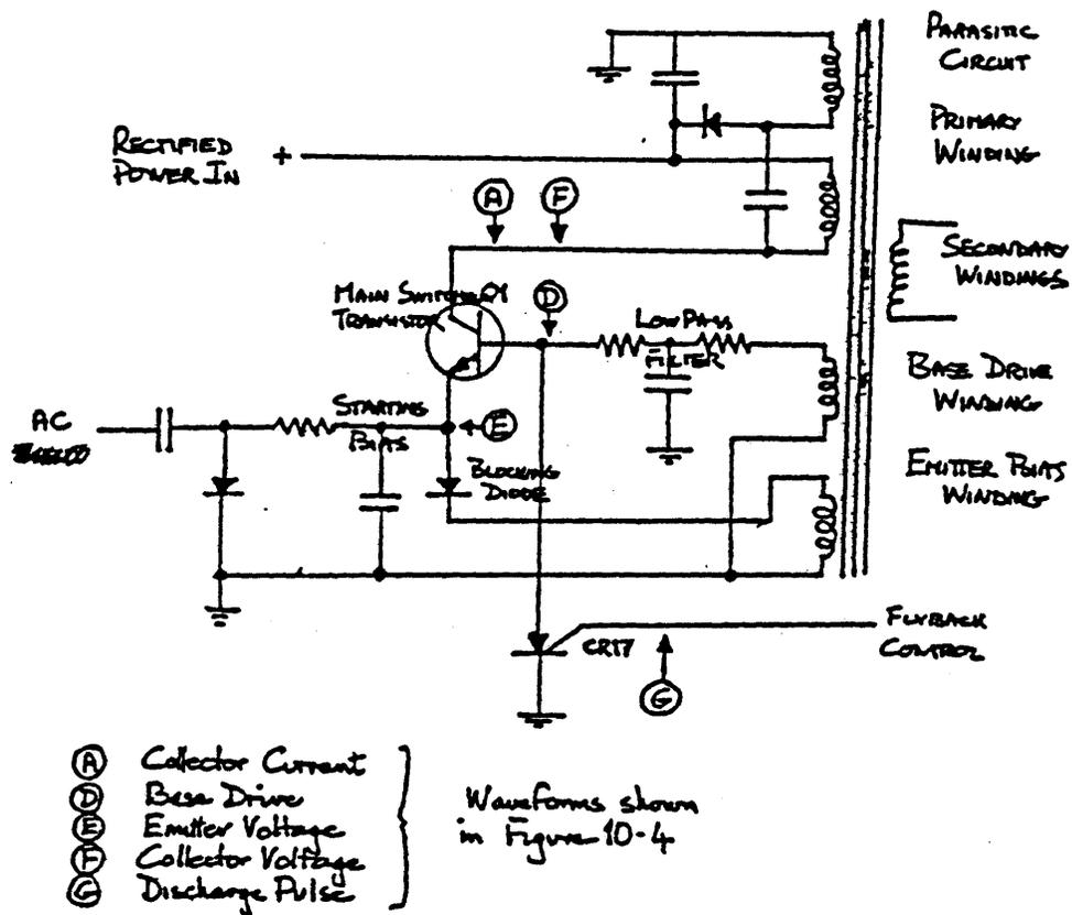
Figure 10-3. Flyback Oscillator Circuit
