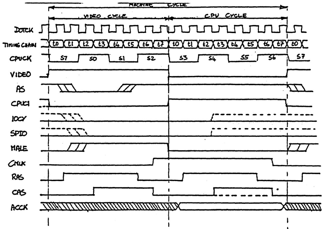
Figure 4-7. Processor Board Internal Timing
