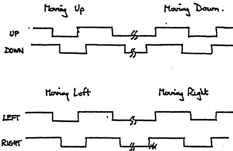
Figure 8-3. Mouse Movement Waveforms
