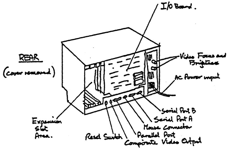
Figure 1-2. System Rear View
