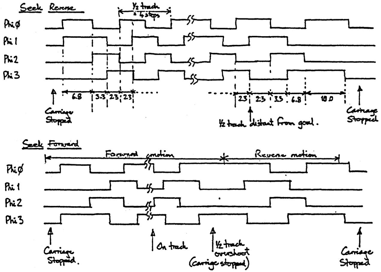
Figure 9-3. Carriage Movement Timing
