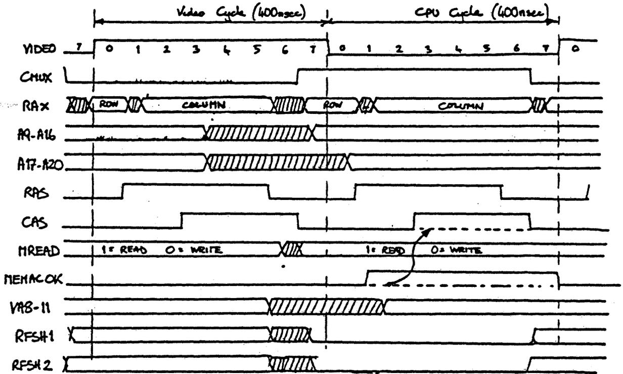
Figure 4-9. Memory Control Timing Diagram
