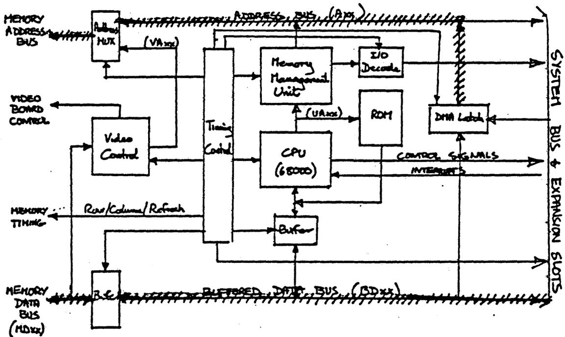
Figure 4-6. I/O Access to Memory (DMA)
