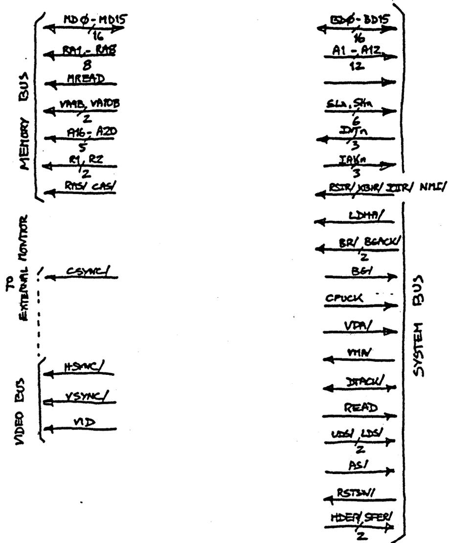
Figure 4-16. Processor Board Bus Interfaces
