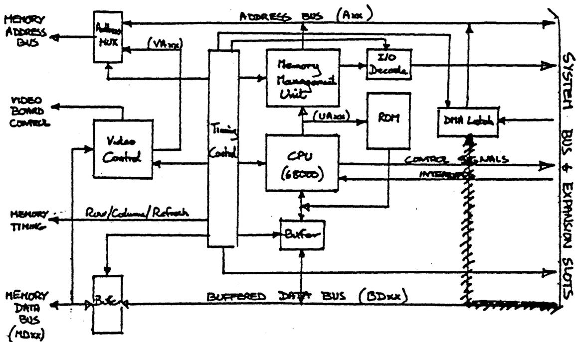
Figure 4-5. I/O Access to DMA Address Latch
