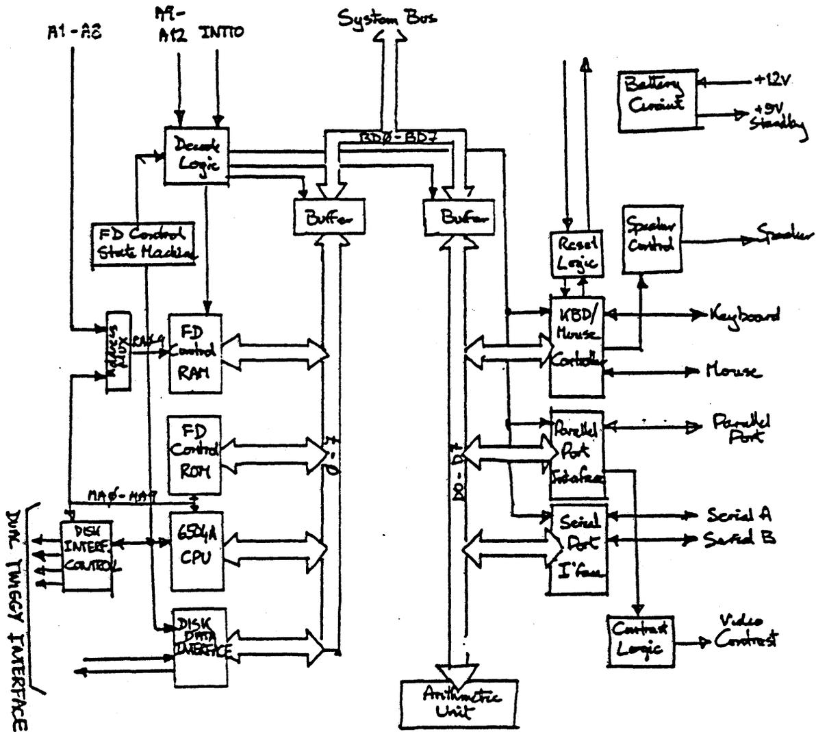
Figure 6-1. I/O Board Block Diagram
