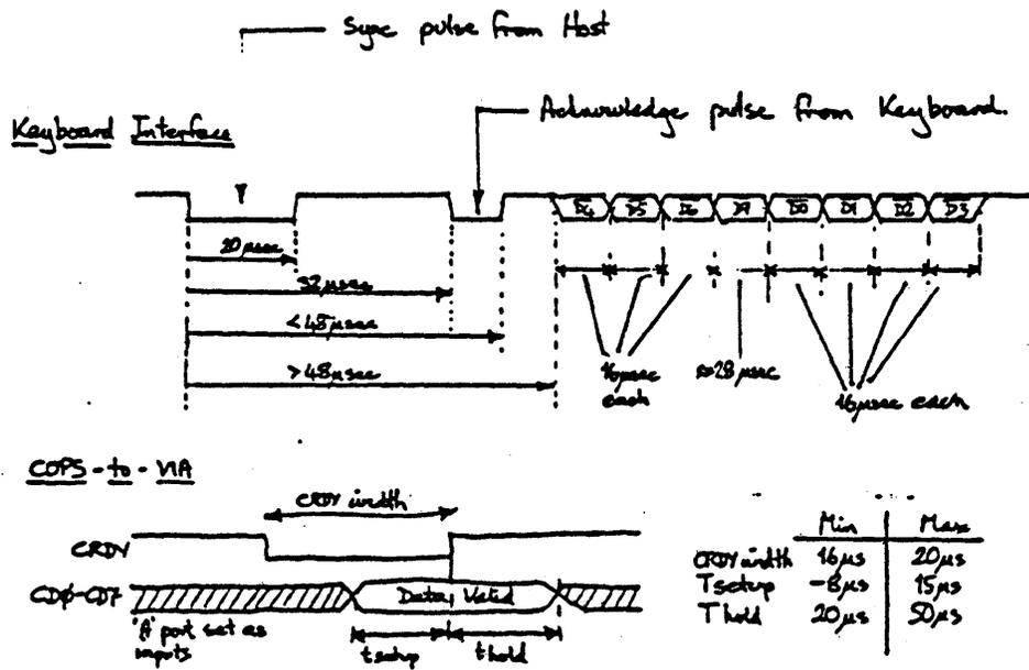
Figure 6-13. Keyboard Data Format and Timing
