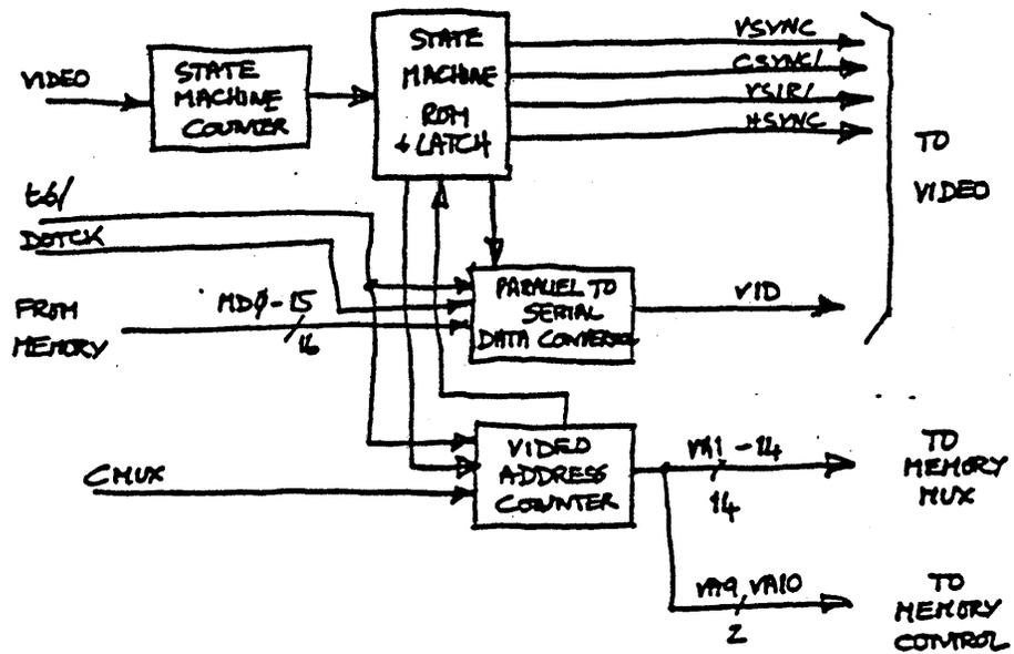
Figure 4-15. Video Control Block Diagram
