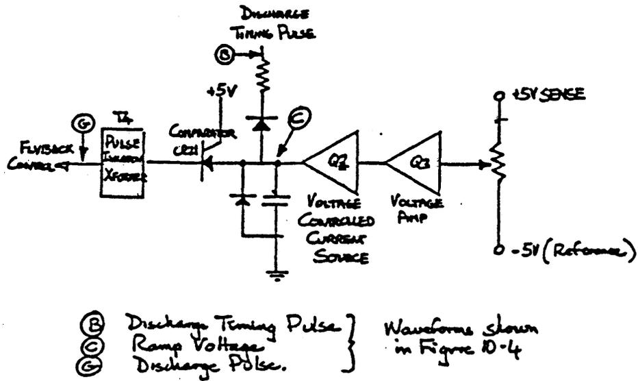
Figure 10-5. Flyback Control Block Diagram
