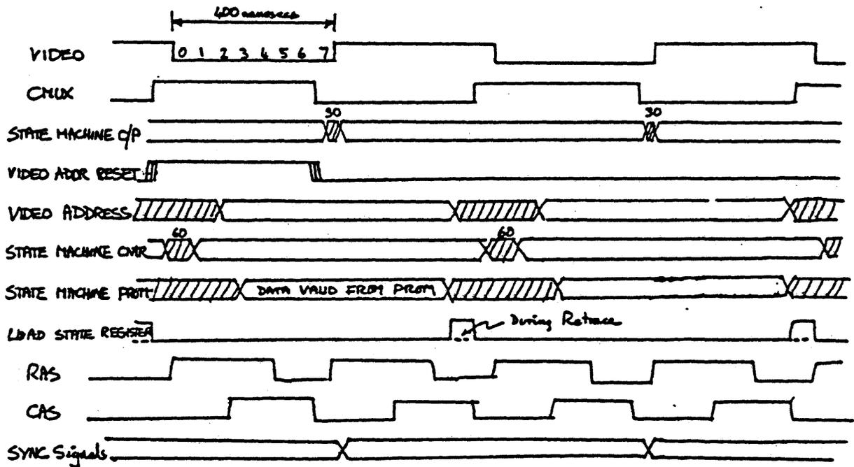
Figure 4-10. Video Control Timing Diagram
