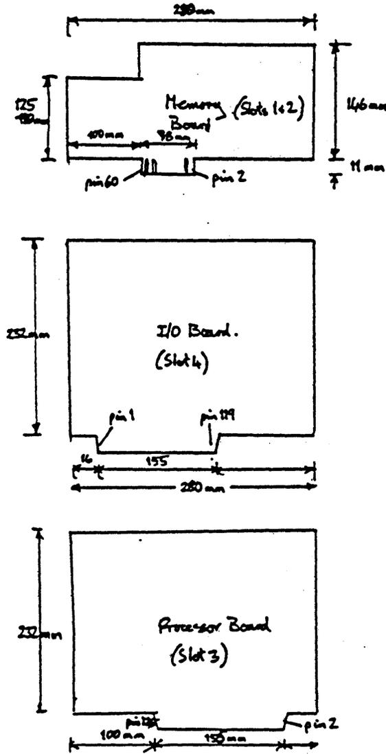
Figure 3-3. Circuit Board Dimensions
