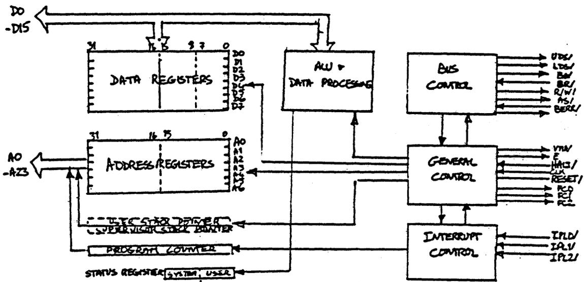
Figure 1-4. Processor Block Diagram
