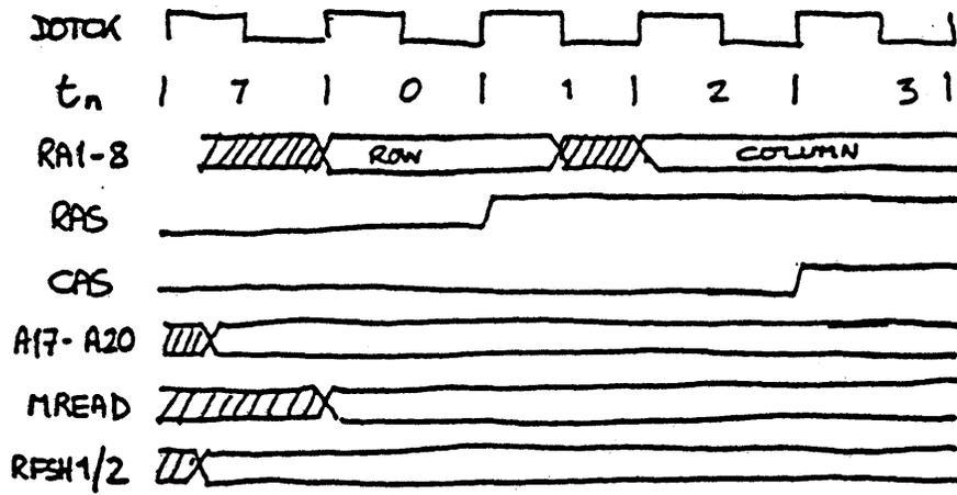
Figure 5-5. Memory Row Address Timing
