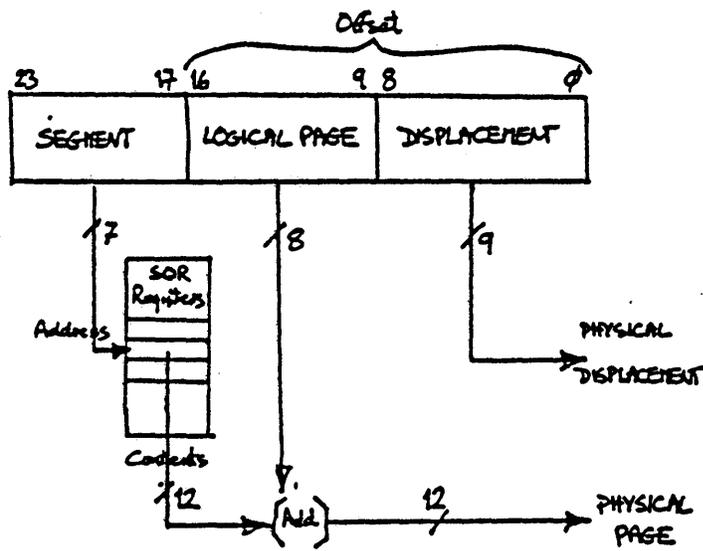
Figure 2-1. Address Word Decode
