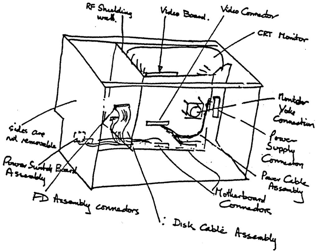
Figure 3-2. Main Chassis Assembly
