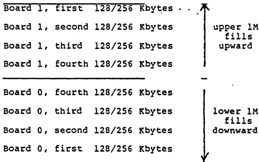
Figure 5-2. Memory Address Decoding
