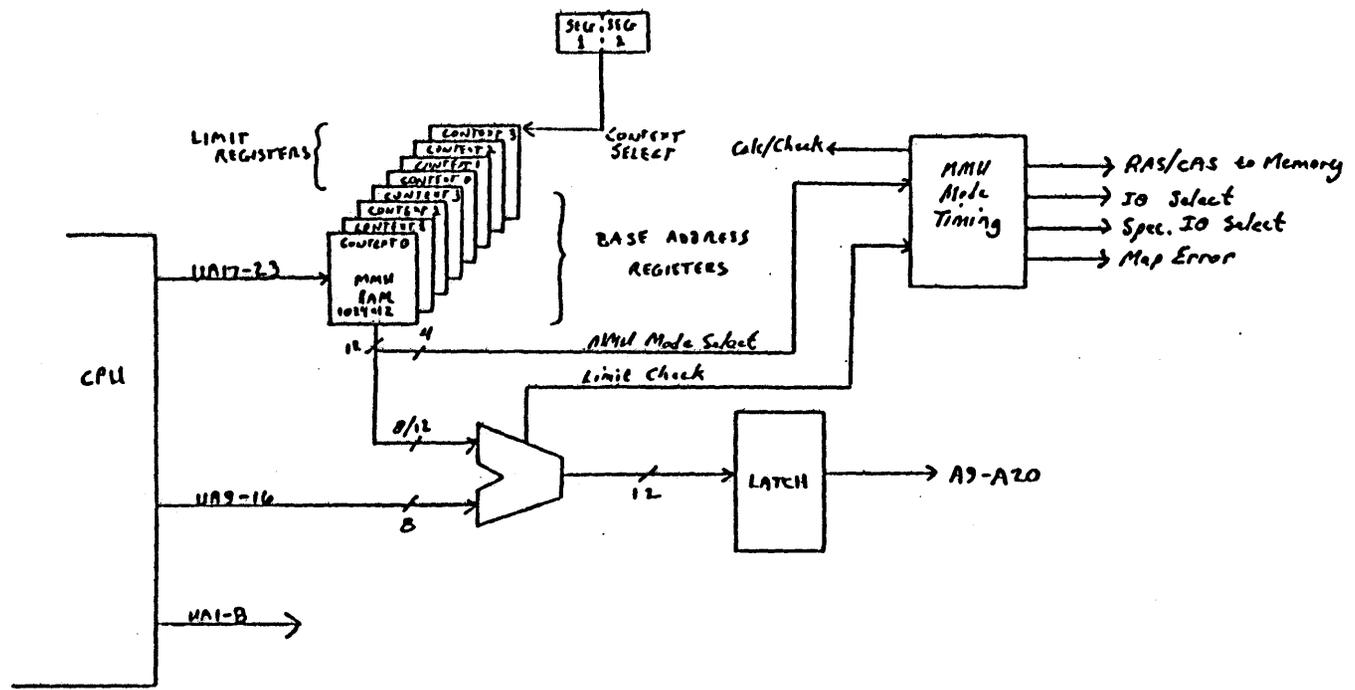
Figure 4-13. MMU Block Diagram
