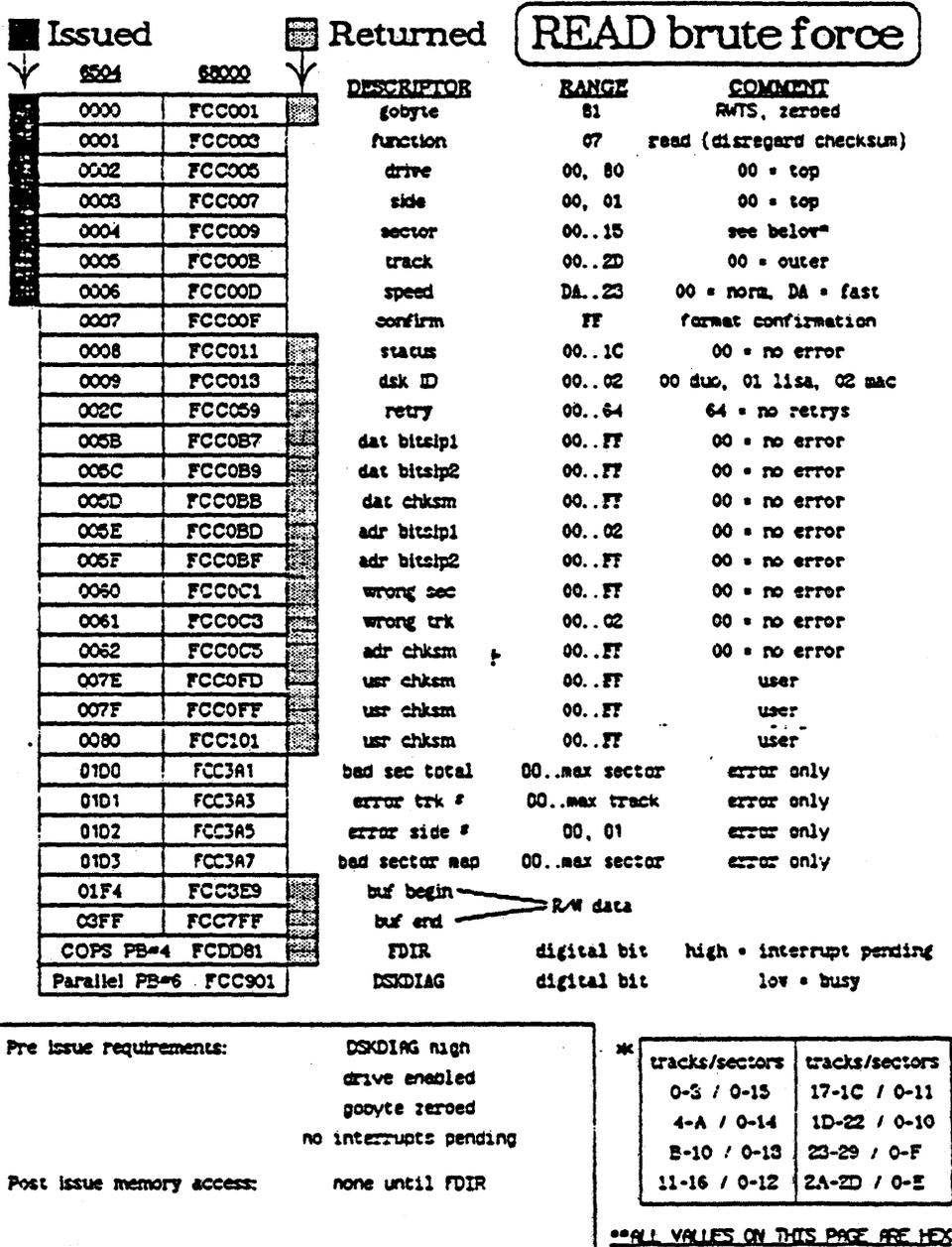
Figure 6-6i. FD Controller Read Brute Force Command
