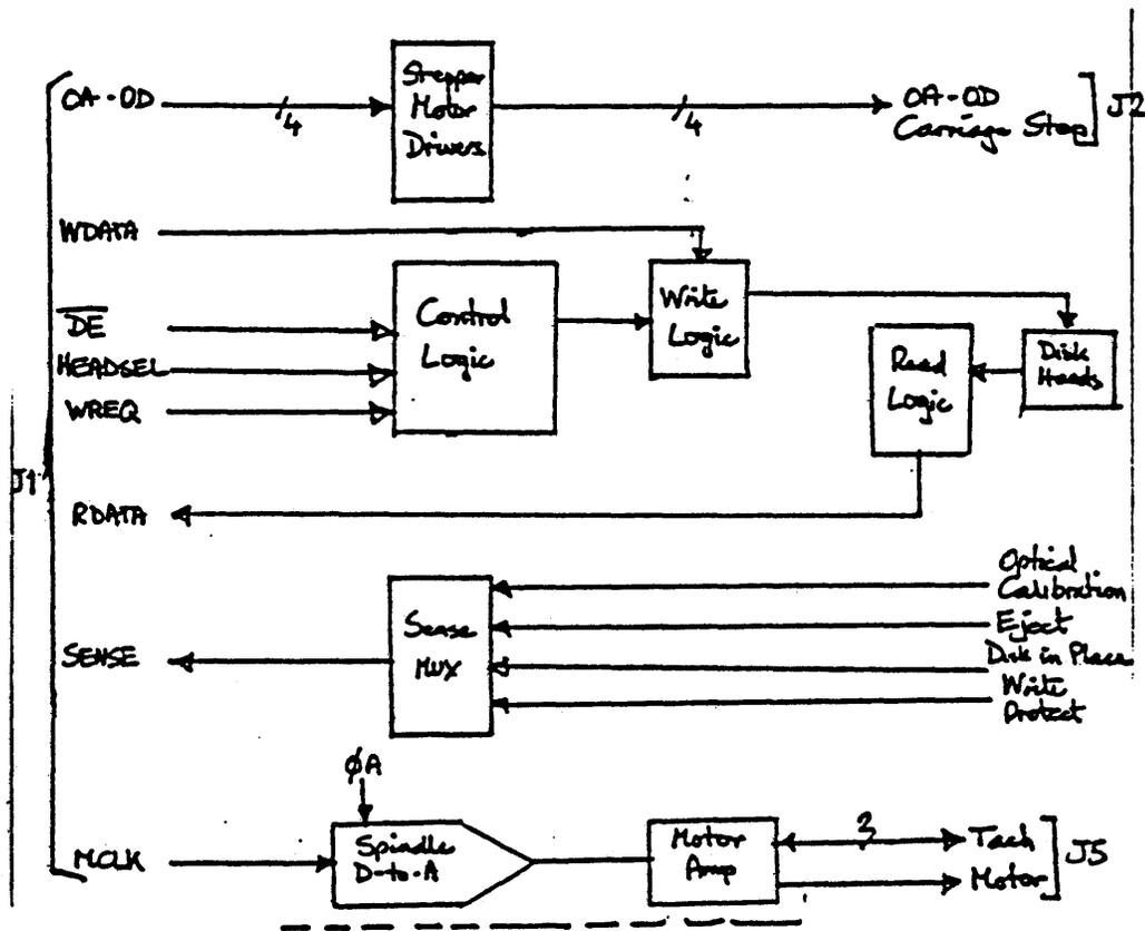
Figure 9-1. Drive Block Diagram
